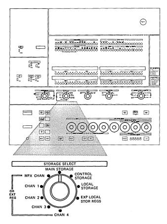
This switch selects the proper storage for manual store/ display operations. It is also used with the ADDRESS COMPARE switch and the ADDRESS COMPARE CONTROL toggle switch for address match functions.
