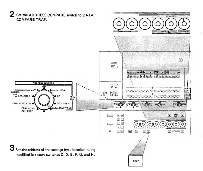
Set data switches A and B to the desired byte match value.
