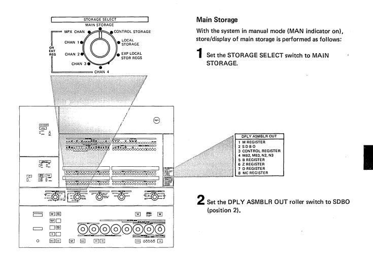
**3** Dial the desired word address into rotary switches, C, D, E, F, G, and H.
