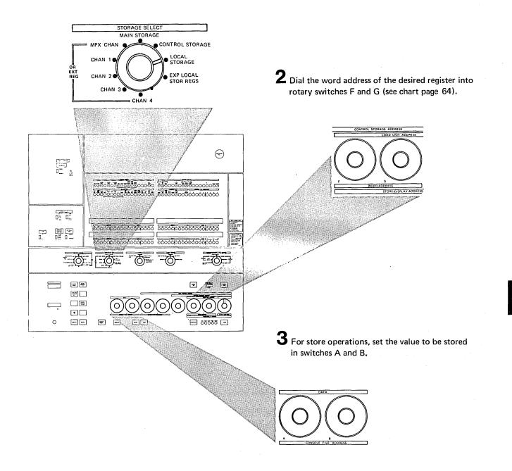
4 Set the byte address at which the data is to be stored in switch H (only the two low-order bits of switch H designate the byte). For example, if switch H is set to C (1100 binary), byte zero is selected.
