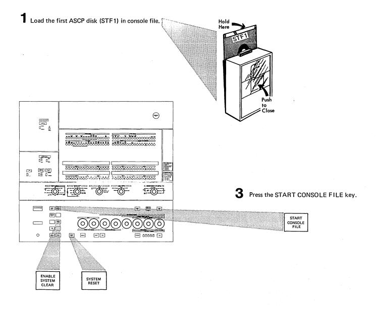
**2** Hold the ENABLE SYSTEM CLEAR key in the operated position and press the SYSTEM RESET key.
