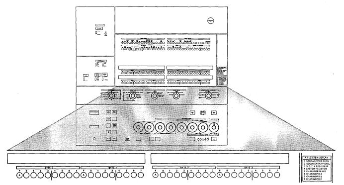
The A-REGISTER DISPLAY roller switch is used with the STORAGE SELECT switch to display the following.
