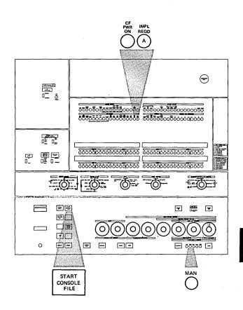
4 When control storage is loaded, the console file powers off automatically. The CF PWR ON indicator and the START CONSOLE FILE key light turn off.
