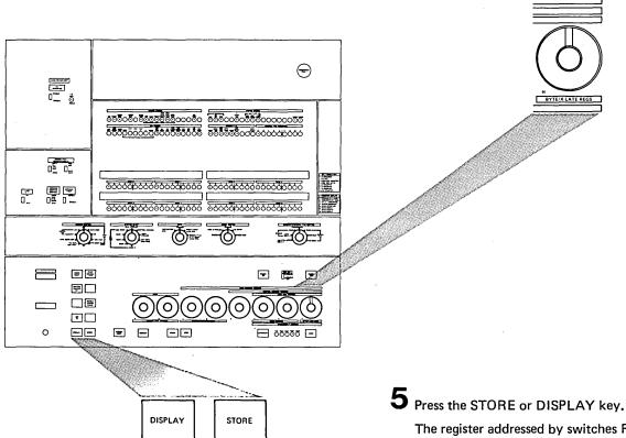
The register addressed by switches F and G is displayed in the A-REGISTER DISPLAY roller switch indicators at the end of the store or display operation.
