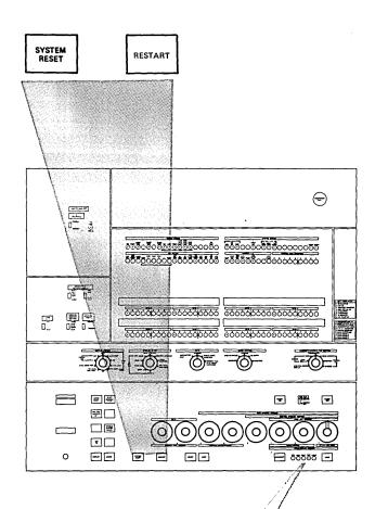
**9** The WAIT indicator comes on and the system enters a wait state. At this point, ready the device that is to be used as an output (example: 1403 Printer).
