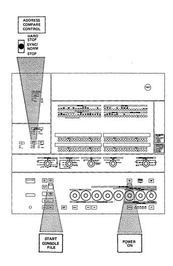
2 If power is not on, press the POWER ON key. An automatic IMPL occurs. If power is on, press START CONSOLE FILE key to initiate the IMPL.
