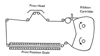
**RIBBON THREADING SCHEMATIC**
