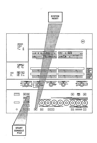
Load the ASCP Disk #2 (STF2) and press the START CONSOLE FILE key.
