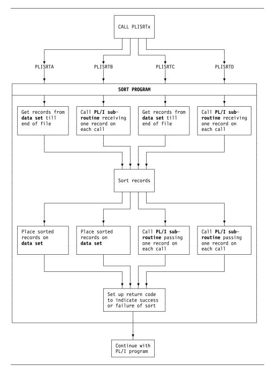
Figure 82. Flow of Control for Sort Program
