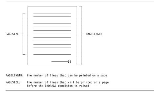
Figure 19. PAGELENGTH and PAGESIZE. PAGELENGTH defines the size of your paper, PAGESIZE the number of lines in the main printing area.
