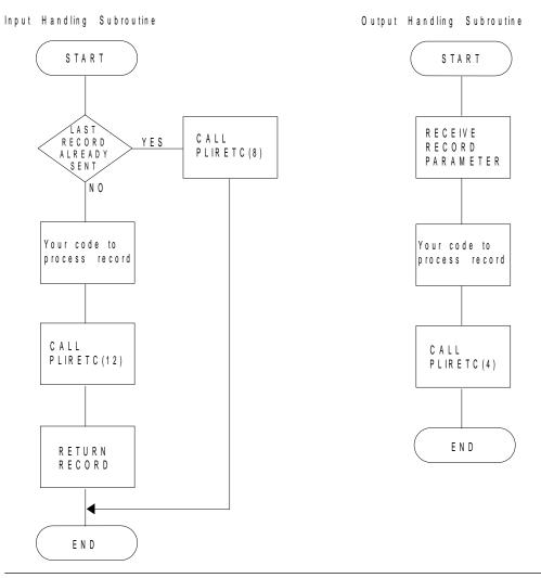
Figure 83. Flowcharts for Input and Output Handling Subroutines
