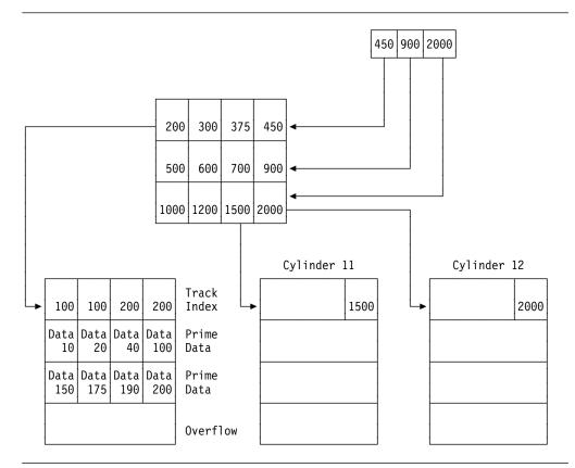
Figure 37. Index Structure of an Indexed Data Set
