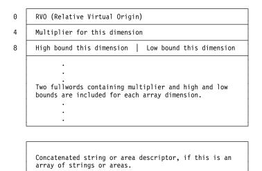
Figure 100. Format of the Array Descriptor for a Program Compiled with CMPAT(V1)
