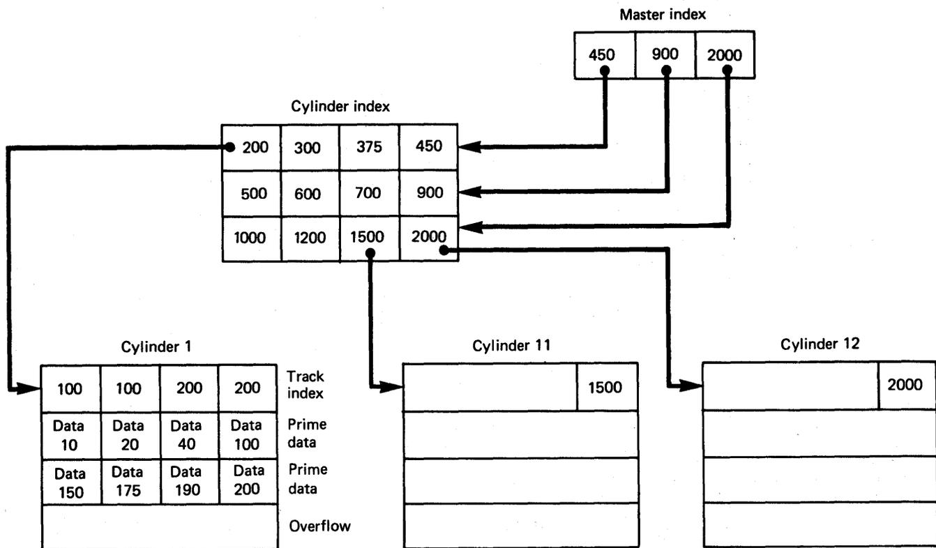
Figure 46. Index Structure of an INDEXED Data Set
