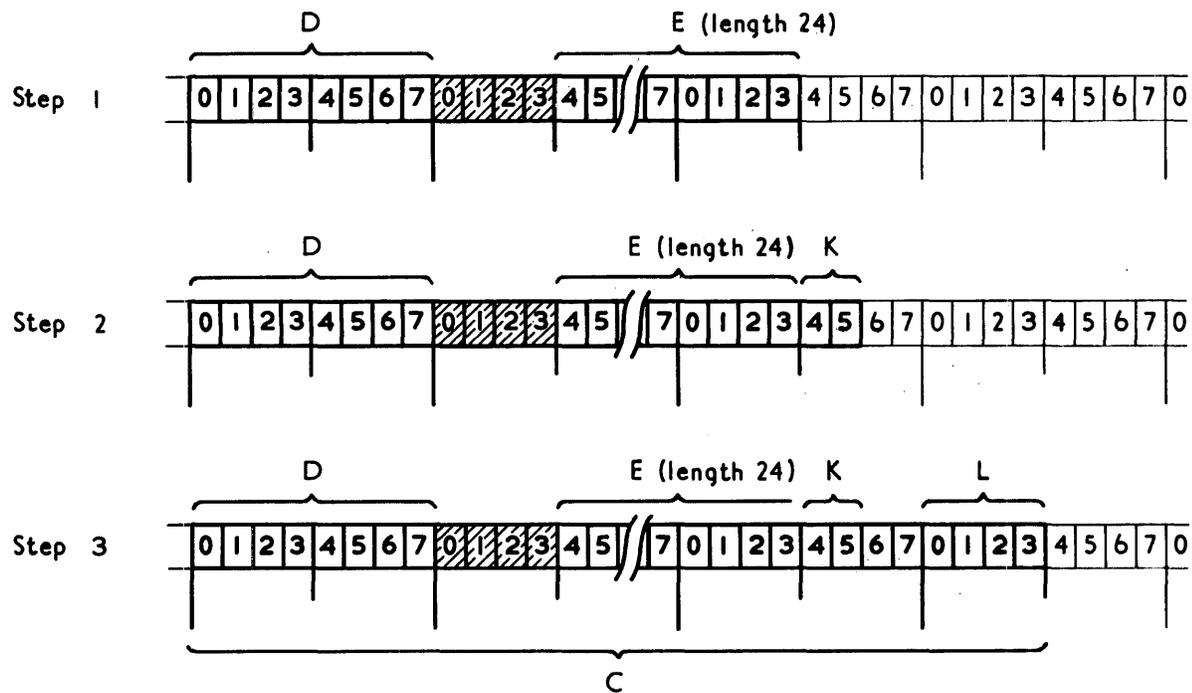
Figure K.7. Mapping of minor structure C
