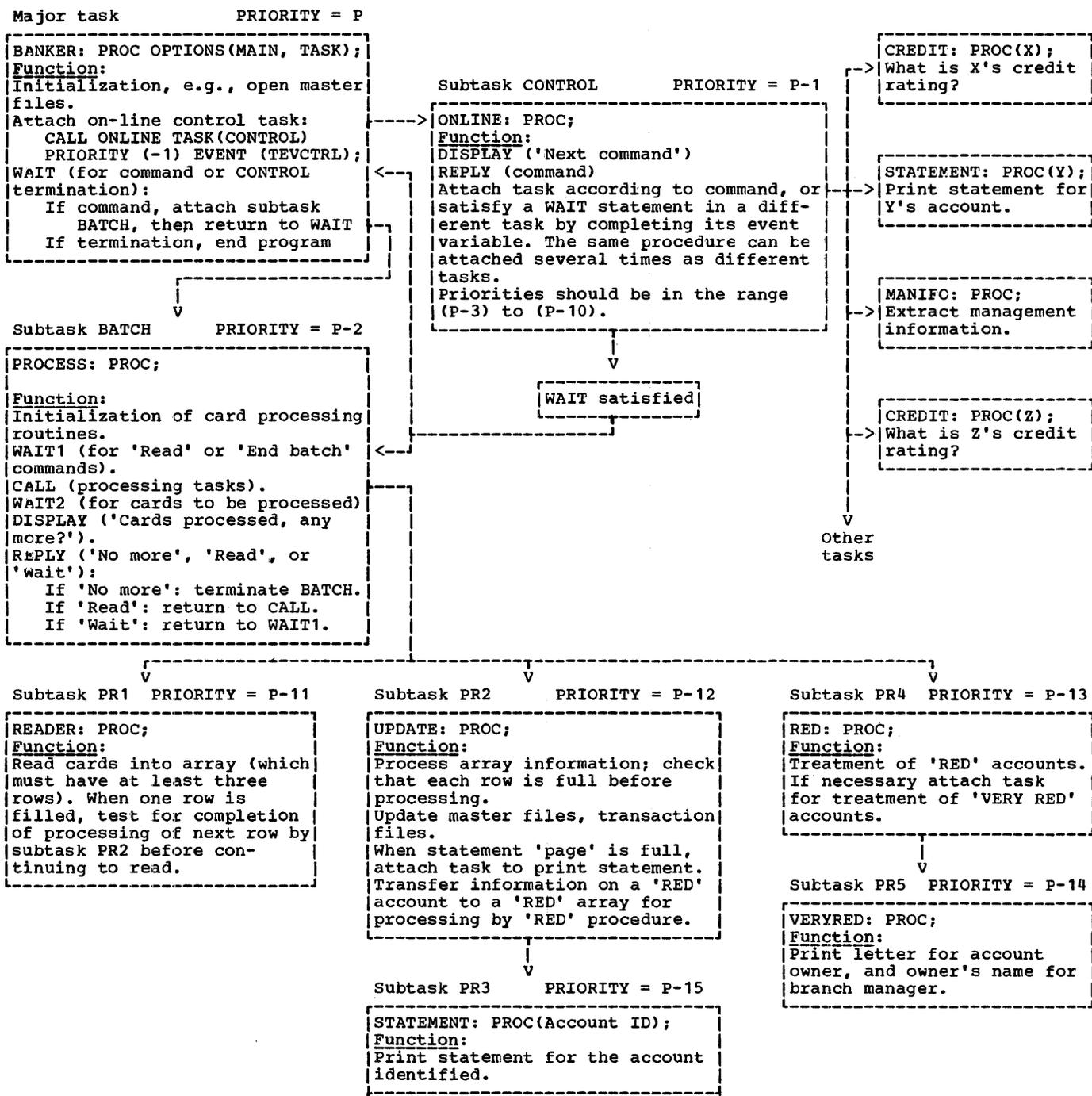
Figure 17.2. Flow diagram for programming example of multitasking
