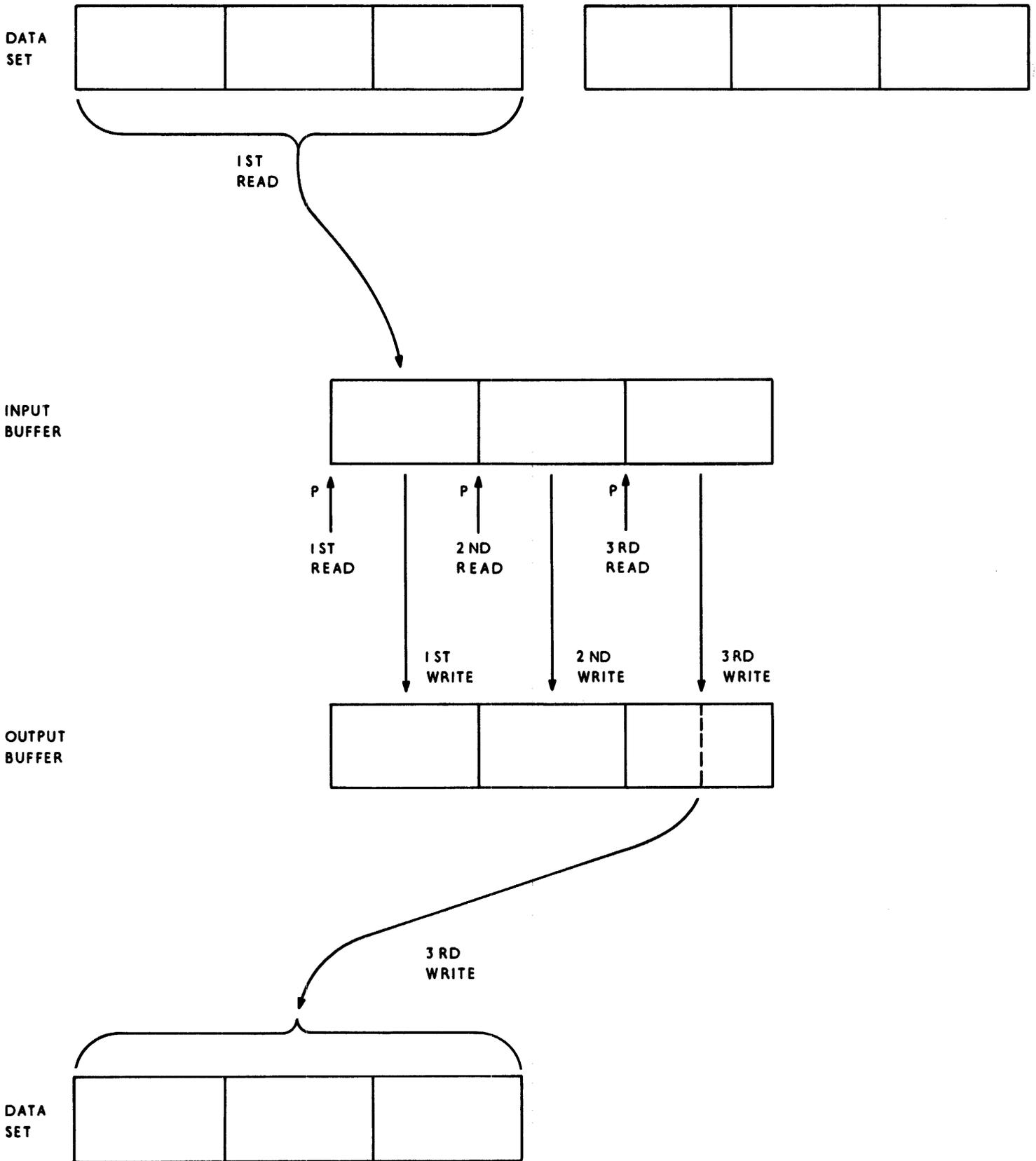
Figure 12.2. Locate mode input, move mode output
