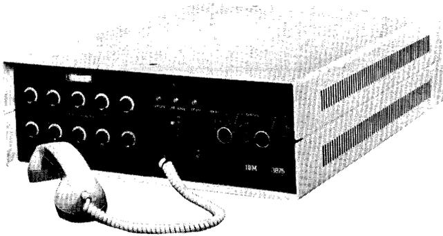
Figure 8-8. IBM 3875 Modem
