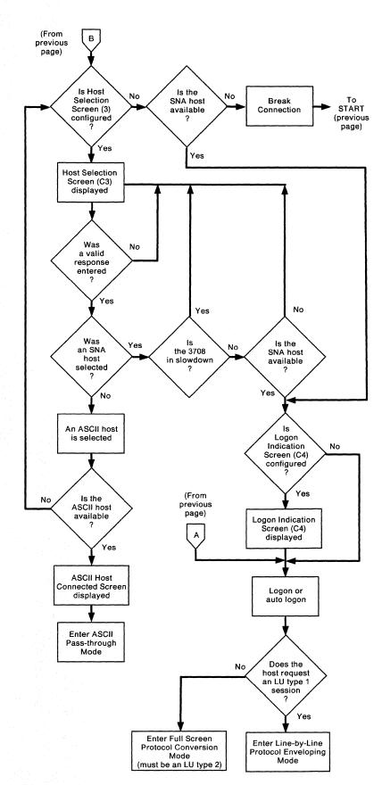
Figure A-1 (Part 2 of 2). Flowchart of the IBM 3708 Logon Process
