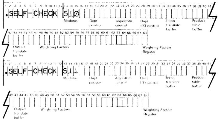
Figure 15. .SELF-CHECK Coding for Standard Modulus 10 and Modulus 11
