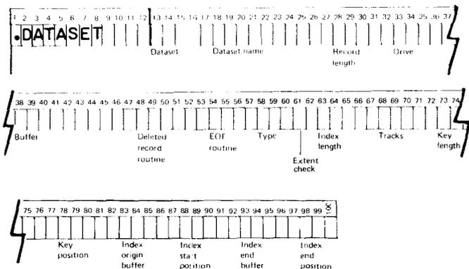
**Figure 6. .DATASET Coding Placement**
