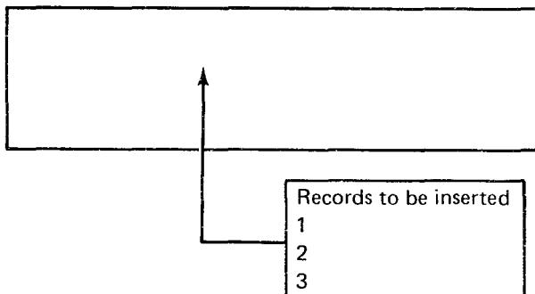
To insert records into a data set, the record insert function performs an operation which creates space in the data set for the number of records to be inserted. The 3742 puts deleted records in the space created. The deleted records have a D in position 001 and a \ (inverse slash) in position 002. The remainder of the record is blank.
