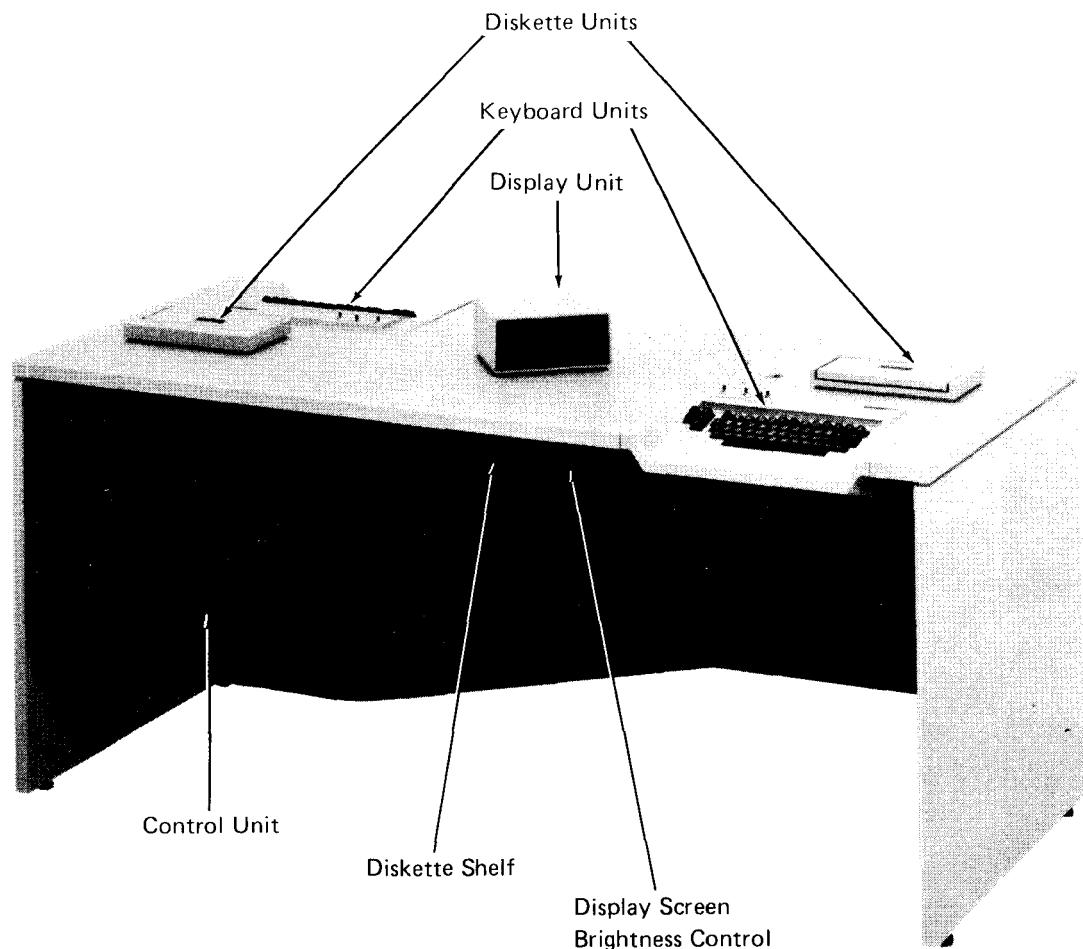
• Figure 1. IBM 3742 Dual Data Station
