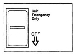
· Use this switch to stop the 3745 in case of an emergency.
