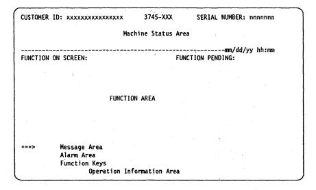
Figure 3. Console Screen Layout
