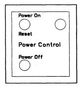
When lit, the **Power On** indicator means that the 3745 is completely powered on. It is lit when the power on procedure is started.
