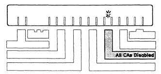
When the indicator is lit, all channel adapters are disabled. When not lit, at least one channel adapter is enabled.
