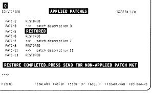
Figure 8-21. Patch Restore Execution Screen (Sample)
