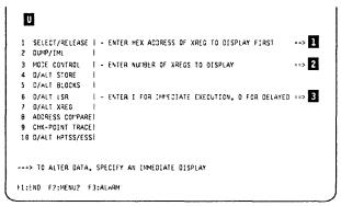
Figure 4-22. Display/Alter Scanner XREG Selection Screen
