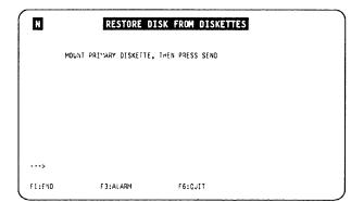
Figure 11-14. Restore Disk Function, Mount Primary Diskette Screen
