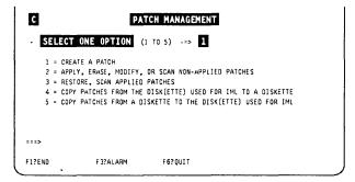
Figure 8-5. Patch Function Selection Screen
