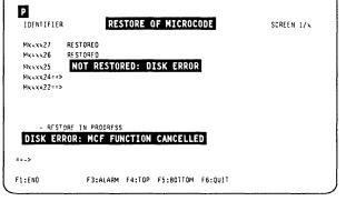
Figure 7-18. Disk Error During MCF Restore (Example)
