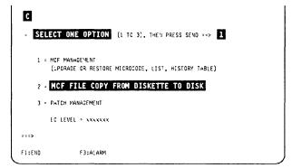
Figure 7-5. MCF/Patch Selection Screen
