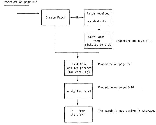
Figure 8-1. Patch Installation Sequence
