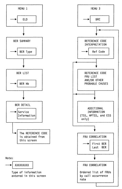
Figure 2-1. BER Display and Handling
