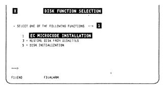
Figure 11-24. Disk Function Selection Screen (IML from Diskette)
