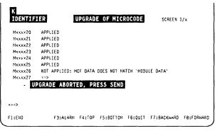
Figure 7-13. Data Error During MCF Upgrade (Example 1)
