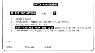
Figure 8-23. Patch Function Selection Screen
