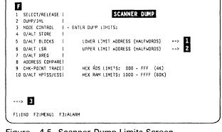
Figure 4-5. Scanner Dump Limits Screen
