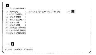
Figure 4-7. Dump or IML Selection Screen
