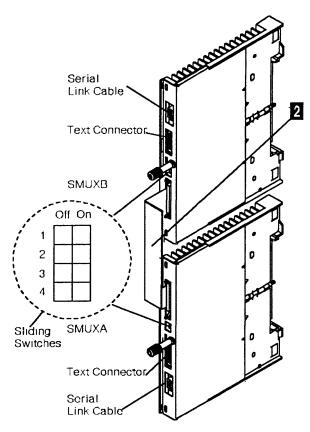
Figure 4-53. SMUX Link and Cable.
