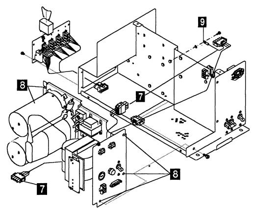
Figure 4-89. PS2 and Primary Power Box Assembly
