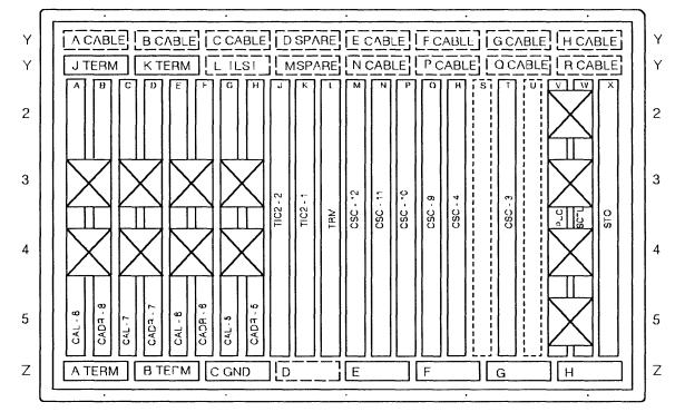
Figure 4-4. 3745 Model 170 Basic Board without TPS and without HPTSS
