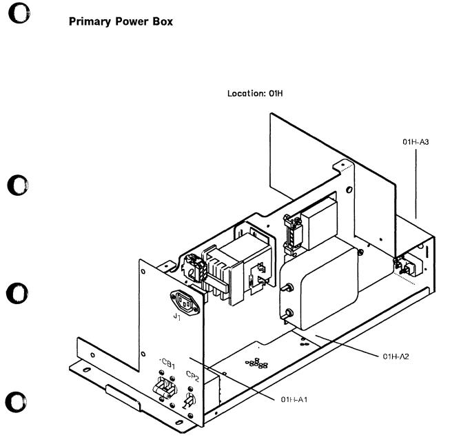
Figure 4-34. 3745 Primary Power Box Components
