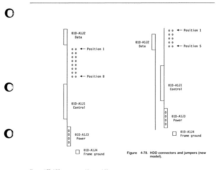
Figure 4-77. HDD connectors and jumpers (old model).
