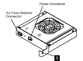
Figure 4-67. Fan 1 Air Flow Detector and Power Cables
