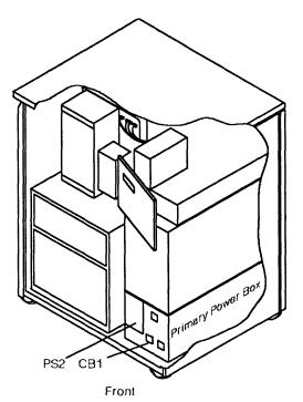
Figure 4-86. Primary Power Box, Power Supply 2 and CB1 Locations
