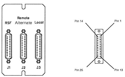
Figure 4-29. 3745 Console Operator Tail Gate
