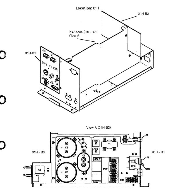
Figure 4-36. 3745 Power Supply 2 Components
