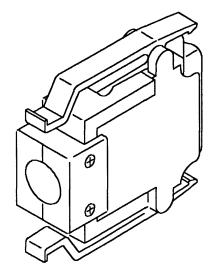
Figure 3-6. LICs Type 1 and 4 Wrap Plug P/N 65X8927
