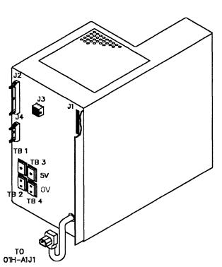
Figure 4-35. 3745 Power Supply 1 Components
