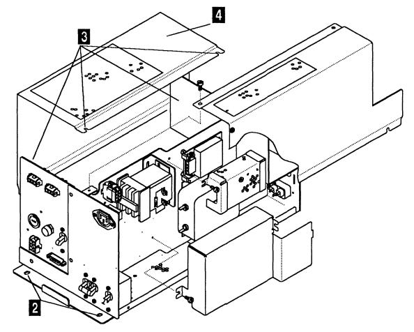
Figure 4-93. Primary Power Box and PS2 Cover Removal
