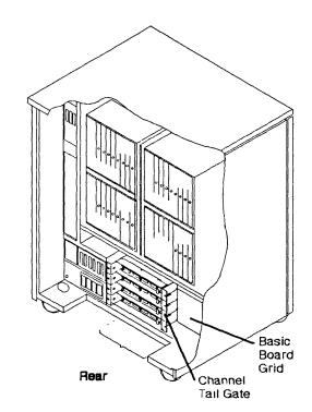
Figure 4-123. Channel Tail Gate and Basic Board Grid
