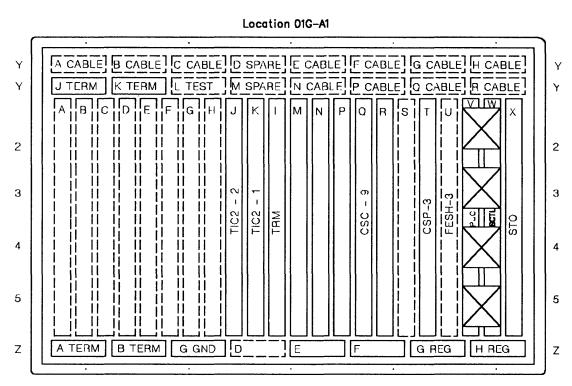
Figure 4-7. 3745 Model 150 Basic Board.
