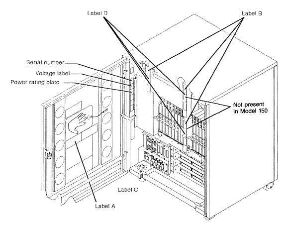
Figure 0-1. 3745 Label and Power Rating Plate Locations (Back)
