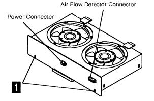
Figure 4-99. FAN 2 Air Flow Detector and Power Connectors
