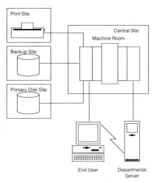
ESCON's fibre optic technology breaks through traditional computing centre barriers, opening up a wealth of new possibilities for configurations
