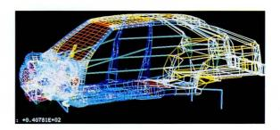
... the protection of passengers is assessed with the aid of crash test simulation ...
