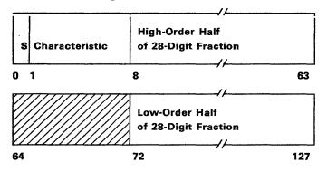
In the short and long formats, the first bit is the sign bit (S). The subsequent seven bit positions are occupied by the characteristic. The following field contains the fraction, which, depending on the format, consists of six or 14 hexadecimal digits.
