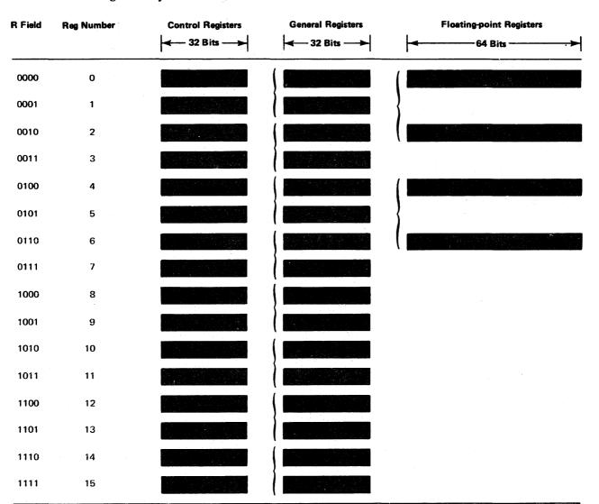
Note: The braces indicate that the two registers may be coupled as a double-register pair, designated by specifying the lowernumbered register in the R field. For example, the general-register pair 0 and 1 is designated in the R field by the number 0.
