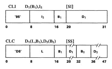
The first operand is compared with the second operand, and the result is indicated in the condition code.
