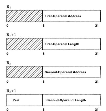
The comparison proceeds left to right, bit for bit, and ends as soon as an inequality is found or the end of the longer operand is reached. If the operands are not of the same length, the shorter operand is considered to be extended on the right with the appropriate number of padding bytes. If both operands are of zero length, the operands are considered to be equal.
