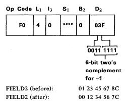
In the SRP instruction, shifts to the right are specified in the second-operand address by negative shift values, which are represented as a six-bit value in two's complement form.
