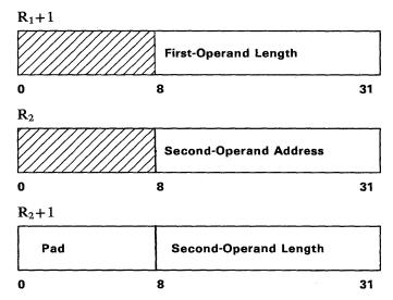
The movement starts at the left end of both fields and proceeds to the right. The operation is ended when the number of bytes specified by bit positions 8-31 of register  $R_1+1$  have been moved into the first-operand location. If the second operand is shorter than the first operand, the remaining rightmost bytes of the first-operand are filled with the padding byte.
