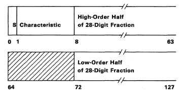
A floating-point number has two signs: one for the fraction and one for the exponent. The fraction sign, which is also the sign of the entire number, is the leftmost bit of each format (0 for plus, 1 for minus). The numeric part of the fraction is in true notation regardless of the sign. The numeric part is contained in bits 8-31 for the short format, in bits 8-63 for the long format, and in bits 8-63 followed by bits 72-127 for the extended format.
