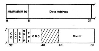
A read operation is initiated at the I/O device, and the subchannel is set up to transfer data from the device to storage. For devices such as magnetic-tape units, disk storage, and card equipment, the bytes of data within a block are provided in the same sequence as written by means of a write command. Data is placed in storage in an ascending order of addresses, starting with the address specified in the CCW.
