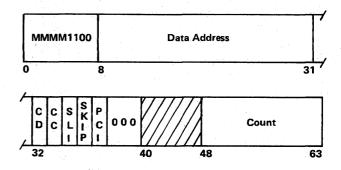
A read-backward operation is initiated at the I/O device, and the subchannel is set up to transfer data from the device to storage. On magnetic-tape units, read backward causes reading to be performed with the tape moving backwards. The bytes of data within
