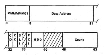
A write operation is initiated at the I/O device, and the subchannel is set up to transfer data from storage to the I/O device. Data in storage is fetched in an ascending order of addresses, starting with the address specified in the CCW.
