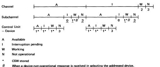
When a device-not-operational response is received in selecting the addressed device, a condition code 3 is set.
