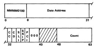
A sense operation is initiated at the I/O device, and the subchannel is set up to transfer data from the device to storage. The data is placed in storage in an ascending order of addresses, starting with the address specified in the CCW.
