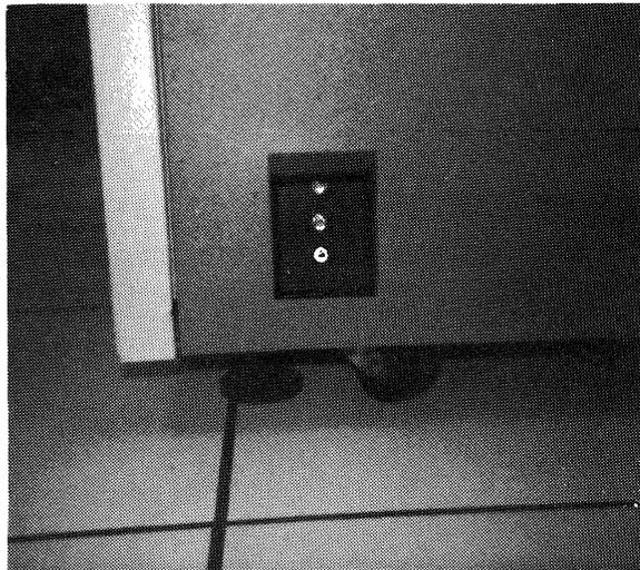
Figure 2. Attachment Aperture for Optional Devices
