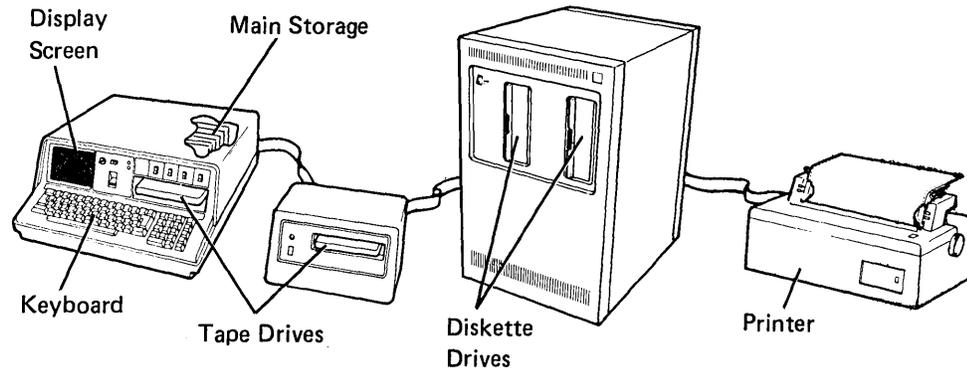
Figure 2. 5110 Computing System Data Processing Elements
