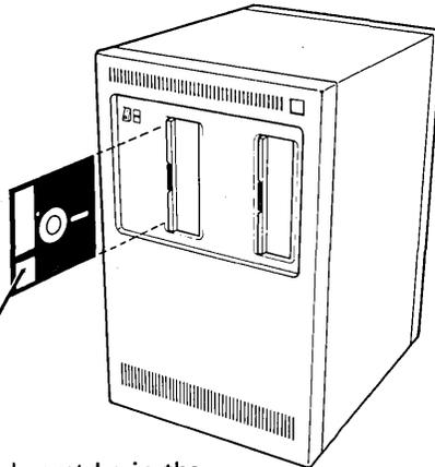
This label must be in the lower corner as the diskette is inserted in the diskette drive. The diskette drive door must be closed and latched after the diskette is inserted.
