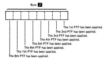
Each bit of the second byte of information indicates whether a program temporary fix has been applied to a module.
