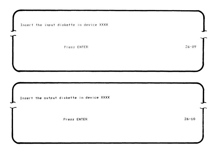
Prompts 26-09 and 26-10 will be displayed each time a diskette should be inserted into a diskette drive. This exchanging of diskettes continues until the entire module is replaced.
