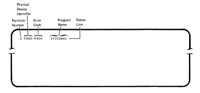
The load prompt and the close failure recovery SCP have the following status line.
