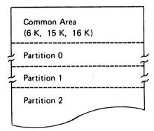
While only one common functions option can be loaded into the IBM 5280 system storage at one time, three versions are available on the IBM 5280 system. Option one (SYSDPRT2) resides on the IBM-supplied SCP diskette and is read into storage when you perform the IPL on the system. Options two (SYSCFA) and three (SYSHELP) reside on the utilities diskette.
