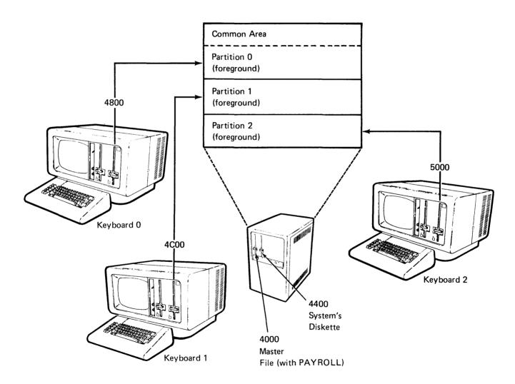
Logical device IDs were assigned in the resource allocation table to each physical device as follows:
