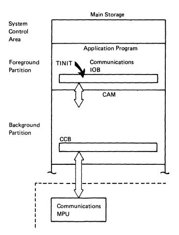
When the CAM reads the TINIT instruction, it completes setting up the CCB and buffers, then turns off the status bit in the IOB and waits for the next instruction.
