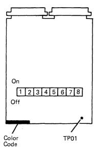
**Note:** Remove the plastic switch cover to change the settings of the switches. After you have changed the settings of the switches, reinstall the switch cover over the switches.
