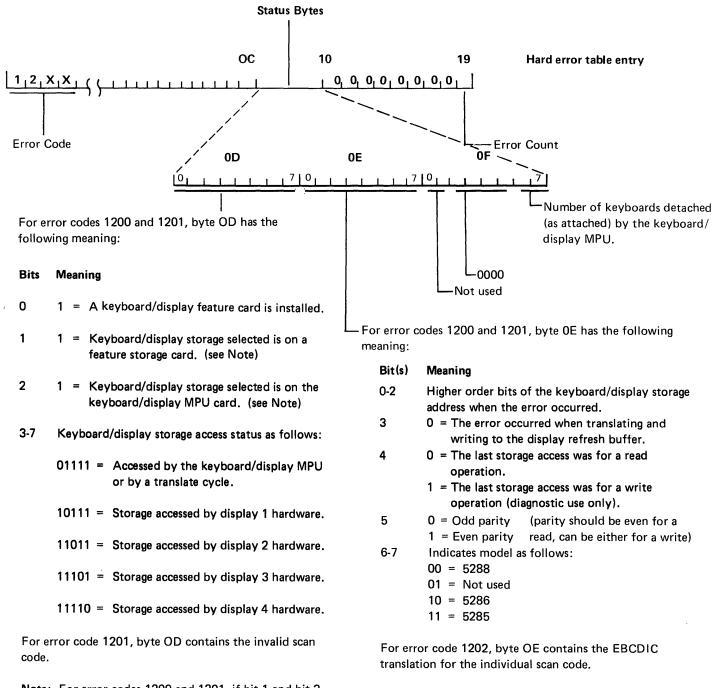
Note: For error codes 1200 and 1201, if bit 1 and bit 2 of byte OD are both 0, an invalid address was accessed.
