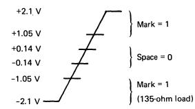
The DDSA interprets receive voltage levels more positive than +1.05 V and more negative than -1.05 V as mark levels.
