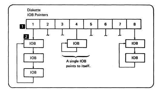
Eight of the IOB pointers in the main storage system control area **1** are assigned to diskette drives: one for each drive that can be installed on the system. Byte 3 of the IOB pointer is set to hexadecimal 00 if a drive is not installed for that IOB pointer. The diskette MPU uses the IOB pointers to find the IOBs **2**.
