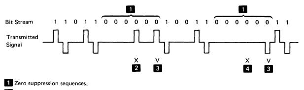
2 First X-bit is opposite in polarity to the preceding 1-bit.
