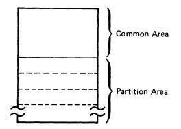
The common area is always located at the beginning of main storage beginning at address 0000. The information here is common to programs located in the partition area. This information is used by the system when executing the application program.
