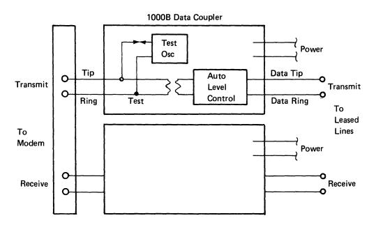
Data Tip (DT) and Data Ring (DR): These lines are used to provide an analog data signal between the user's modem and the coupler.
