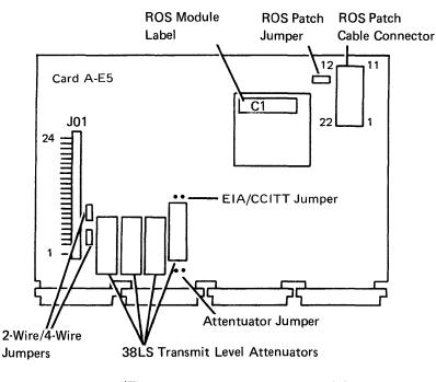
(The attenuators are present on cards in the United States and Canada when a 38LS switched network card is installed.)
