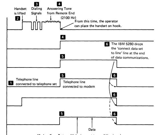
Modem Sync Pattern (if the 'request to send' line is on)
