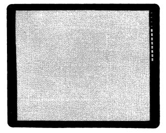
No parity check: mixture of reverse image and normal image -This column of data flashing
