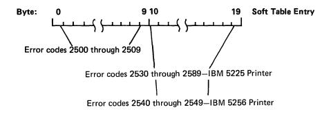
If a count byte reaches 255 (hexadecimal FF), the error code assigned to that byte is no longer counted.
