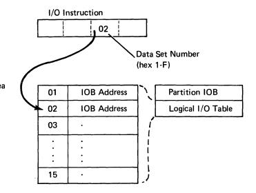
The logical I/O table consists of 4-byte entries in two different formats. One format is associated with keyboard/display IOBs, the other format is for both diskette and printer IOBs. The table contains the address of the device IOB, which the main MPU uses to locate the IOB. The device IOB defines the I/O operation that the device performs.
