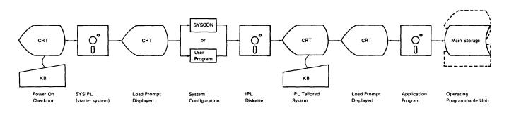
When the power switch on the system is set to the On position, a power-on check is performed to test the operation of several areas of the system. If an area fails, power-on check indicators are displayed to show where the failure occurred. For a detailed description of the power-on check and indicators, see 931 in the diagnostic aids section.
