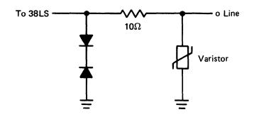
The circuit passes the low-voltage data signals through the 10-ohm resistor. If a high voltage surge occurs on the telephone line, the protection circuit shunts the circuit to ground, protecting the 38LS in most cases.
