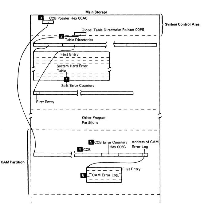
Because these tables are in main storage, they must be dumped to diskette before power off, soft IPL, or before canceling the communications access method. If the tables are not dumped to diskette, they will be lost. The following chart shows the methods and the programs supplied for displaying or printing the error tables:
