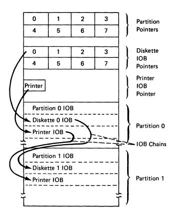
When more than one device IOB is assigned to an I/O device such as the diskette or printer, an IOB chain is created. Each device IOB contains the address of the next assigned device IOB. IOB chains can be either in the same partition or they can address additional device IOBs in another partition. In either case, the last device IOB on the chain points back to the first IOB.
