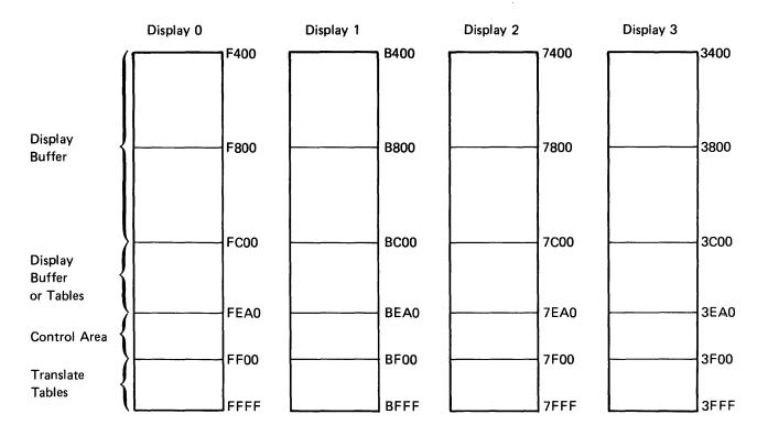
Each partition contains a control area, translate tables, and a display buffer for its assigned keyboard/display.
