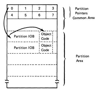
The partition IOB also specifies other information, such as how long the main MPU can execute object code instructions within the partition. A timer, set when a program is assembled, is used to time program execution. When the time limit is reached, the main MPU leaves the partition and goes to the next partition.
