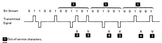
2 First X-bit is opposite in polarity to the preceding 1-bit.
