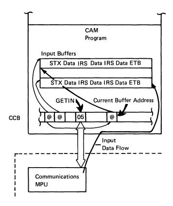
6. The application program can now read the data from the buffer one record at a time. It does this with the TREAD instruction. The application program must issue one TREAD instruction for each logical record. When the CAM program reads the TREAD instruction, it places one logical record (from the buffer acquired by the GETIN command in step 5) into the logical record buffer as shown in the following illustration:
