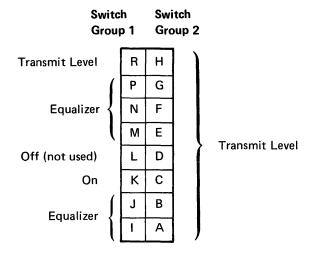
Remove the plastic switch cover to change the settings of the switches. After you have changed the settings of the switches, reinstall the cover switch over the switches.
