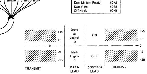
Data Tip (DT) and Data Ring (DR) 7 8 : These lines are used to provide an analog data signal path between the customer's modem and the coupler.
