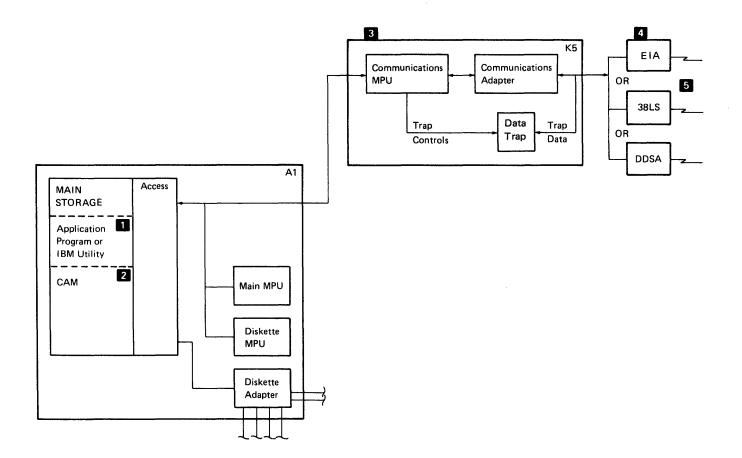
**1** The application program manages data for the user's job. For example, if the user is transmitting data from diskette to the remote station, the application program reads the data from the diskette and writes it to the CAM (communications access method) program. When data is being received, the application program reads the data from the CAM program and writes it on diskette, prints it on the printer, or displays it on the screen.
