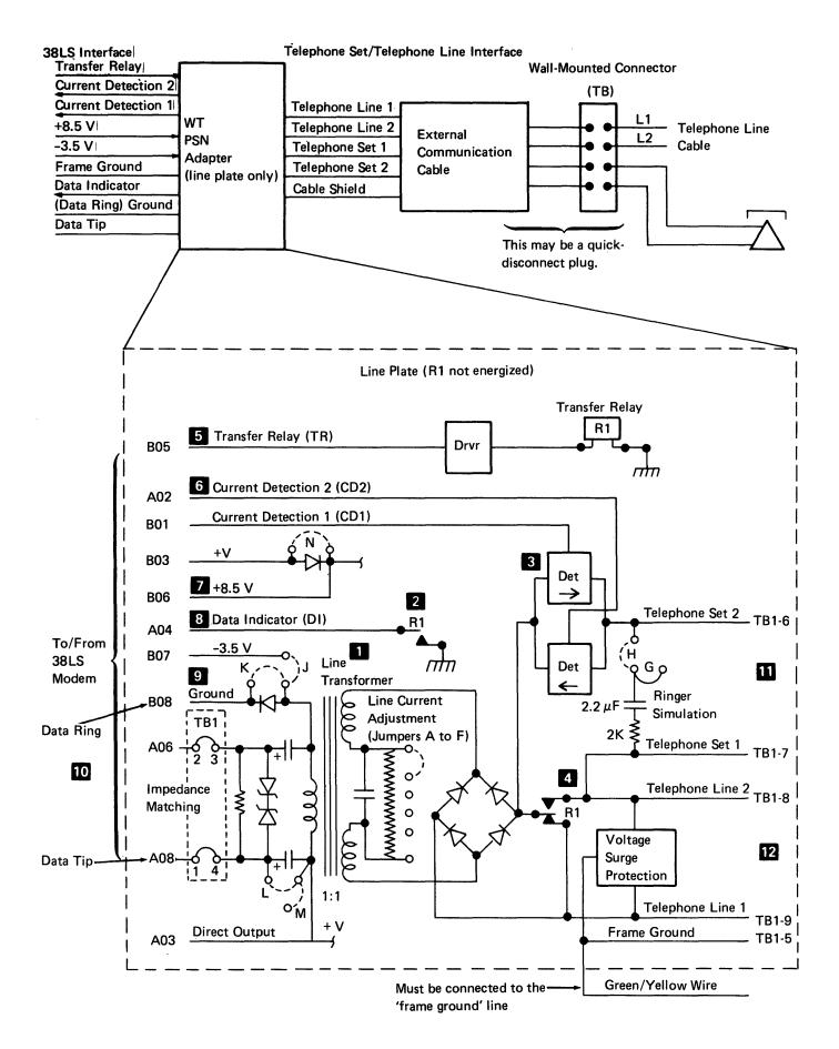
During ringing, the 'current detection 1' and 'current detection 2' lines become alternatively active.
