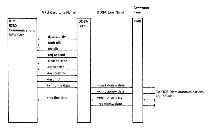
'+xmit line data': This line is activated by the communications MPU card in sync with the transmit clock. A mark (1-bit) is sent as a positive (+5 V) signal, and a space (0-bit) is sent as 0 volts.
