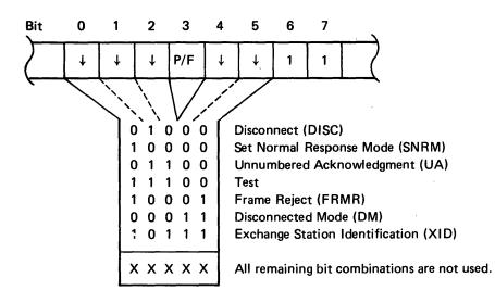
The nonsequenced format is used to perform data link control functions. The commands and responses for the nonsequenced format are:
