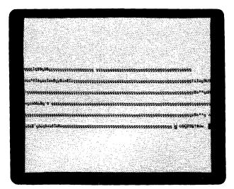
Parity Check: Reverse image All data flashing
