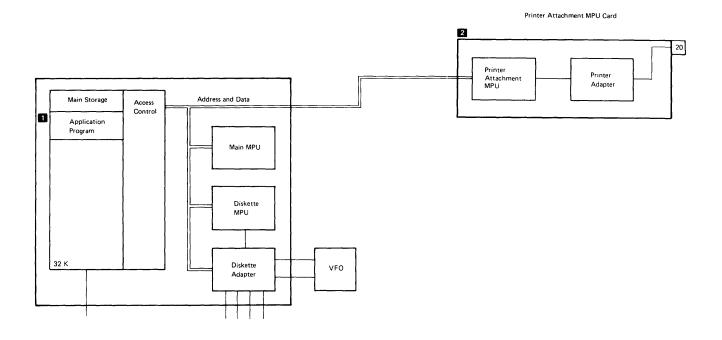
The components required are an application program in main storage **1** and the printer MPU card **2**.
