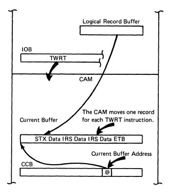
6. When the buffer is full and ready to transmit, the CAM program issues a PUTOUT command to the MPU. The MPU then places the current buffer address on the bottom of the output queue. At least one output buffer is required; however, if storage is available, there can be more than one buffer. The communications MPU transmits the data from the buffer on the top of the output queue as shown:
