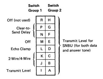
Remove the plastic switch cover to change the settings of the switches. After you have changed the settings of the switches, reinstall the switch cover over the switches.
