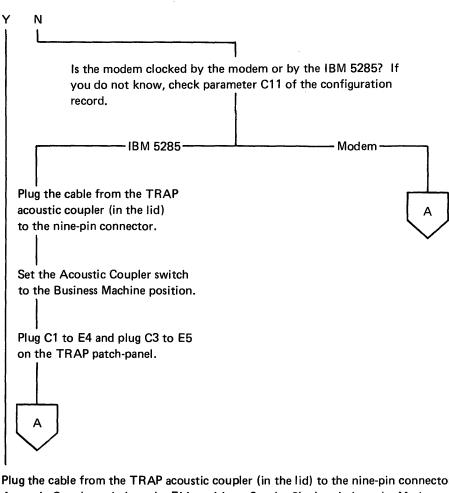
Plug the cable from the TRAP acoustic coupler (in the lid) to the nine-pin connector. Set the Acoustic Coupler switch to the EIA position. Set the Clock switch to the Modem position. Turn the On/Off switch to the Off position.
