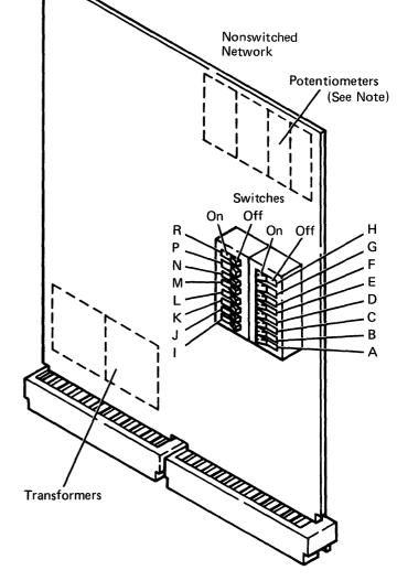
**Note:** The 38LS for a nonswitched network with manual answer SNBU has three potentiometers. The 38LS for a nonswitched network with auto-answer SNBU has four potentiometers.
