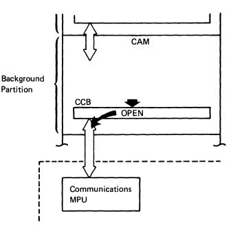
When the communications MPU reads the bit indicating a new command is in the CCB, it reads the command (in this case the OPEN command) and performs the operation specified as follows. Refer to logic diagram *LD11* in the *System Logic Manual* while you read the following description.
