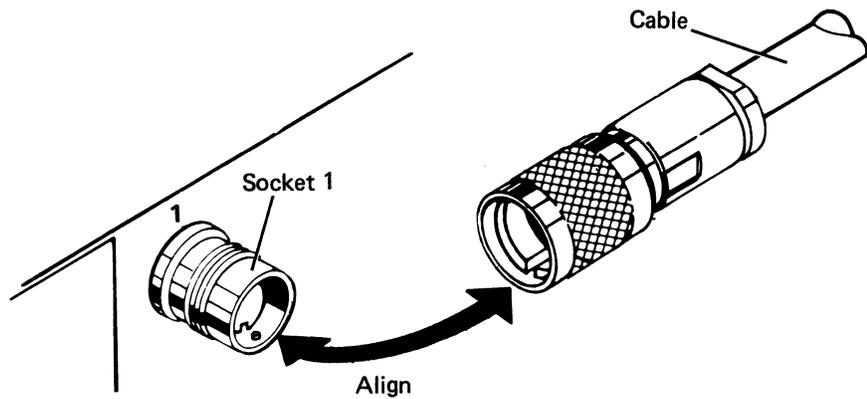
4. Turn the retaining ring clockwise until it is tight.
