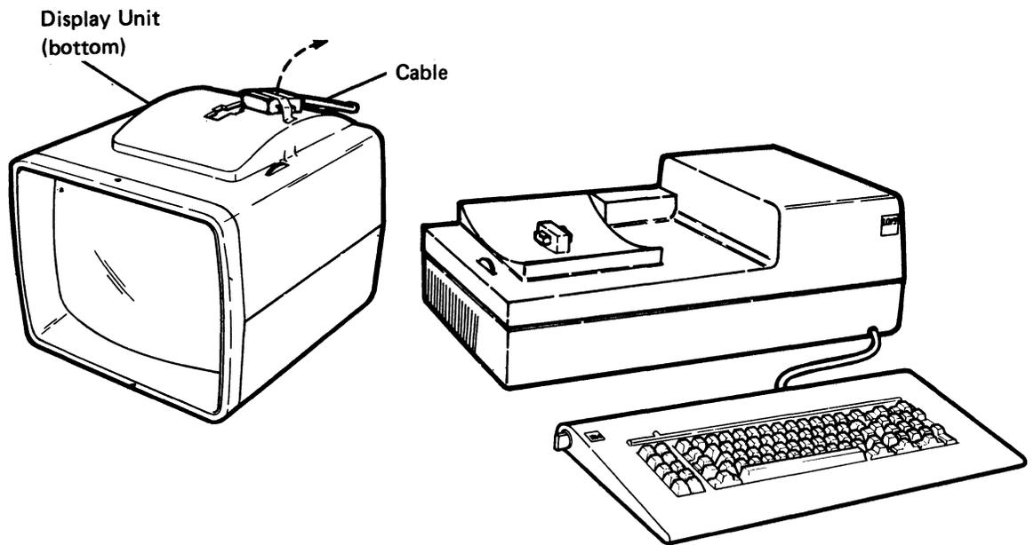
2. Turn the display unit over; then align and slowly position it over the lower unit.
