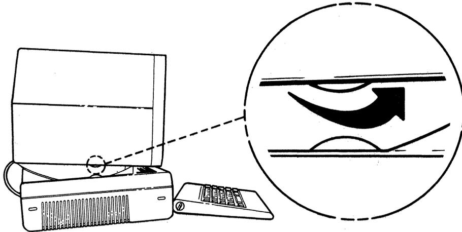
15. Allow 20 seconds for the display station to warm up. When the dash (-), five display indicators (--), and cursor (■) appear on the display screen, adjust the Brightness control until the display is at a comfortable brightness. Go to Section 3, *Connecting the Display Station*.
