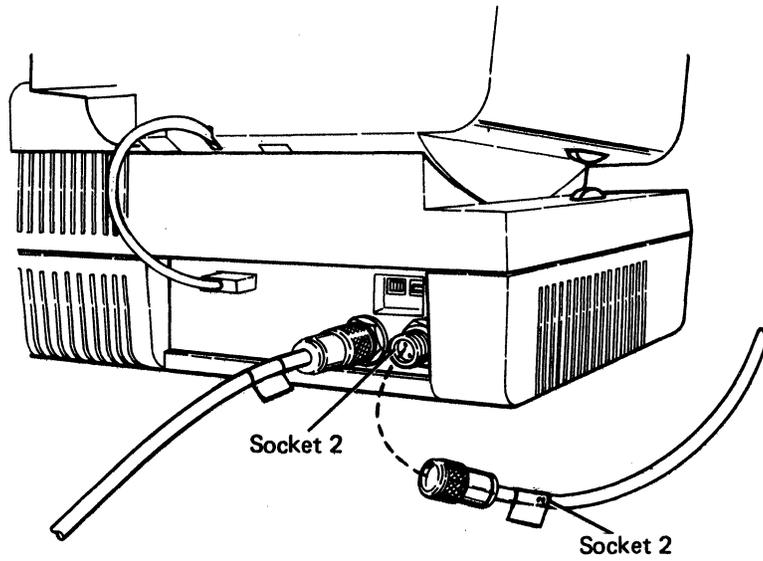
**Note:** A cable connected to socket 2 must always go to socket 1 on the next work station.
