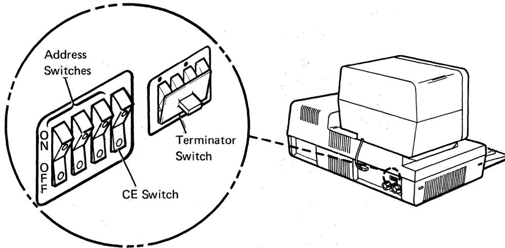
1. **Get the address from the floor plan, from the label attached to the cable, or ask your planner. The *address* for the display station that you are setting up is a *number* (0 through 6).**
