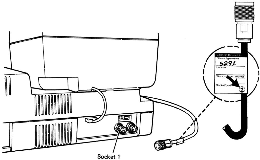
3. Align and push the cable into socket 1.
