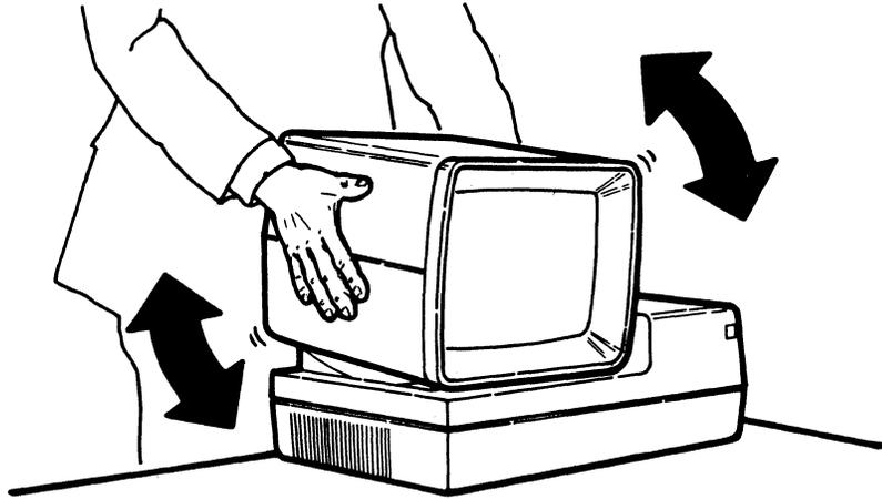
4. Ensure that the display unit is properly seated onto the lower unit.
