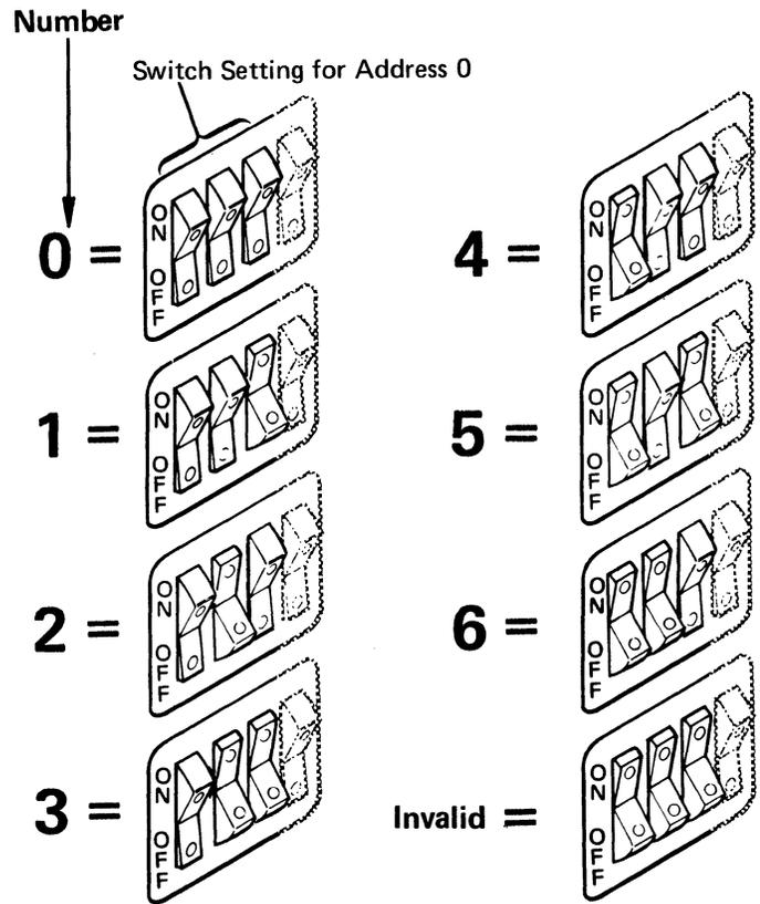
3. Using the switch setting in the above chart as a guide, use a ballpoint pen or pencil to set the switches.
