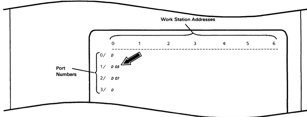
Press the **Cursor Up** or **Cursor Down** key to increase or decrease the value in field 1 -> until it is the same as the code beside the first D on the setup form.
