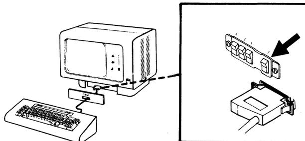
The following illustrations show the location of the Terminator switch on the printers.
