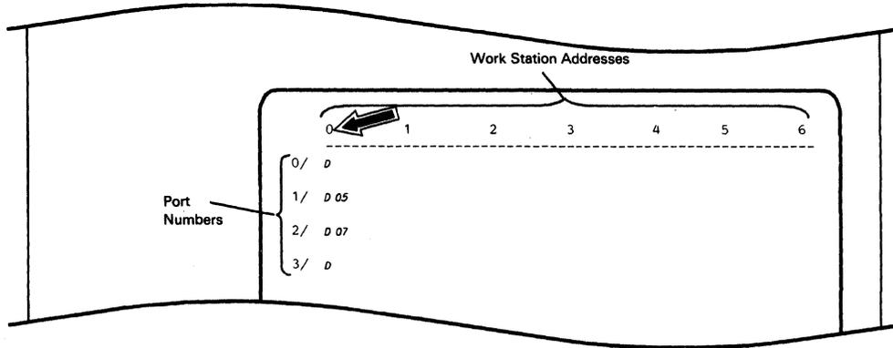
Press the **Cursor Up** key until the address appears in the position of the second dash.
