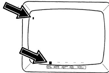
**Do these indicators on the 5294 Control Unit and the display station(s) come on?**
