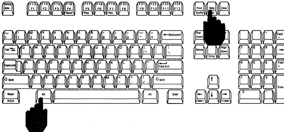
If an error code appears in the upper left corner of the display after you press these keys, press the Reset key and repeat Step 3.4.
