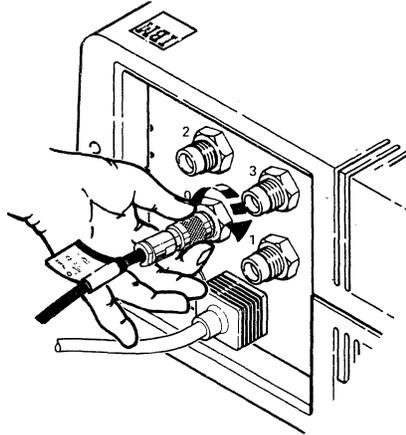
This part of the cable connector is the retaining ring.
