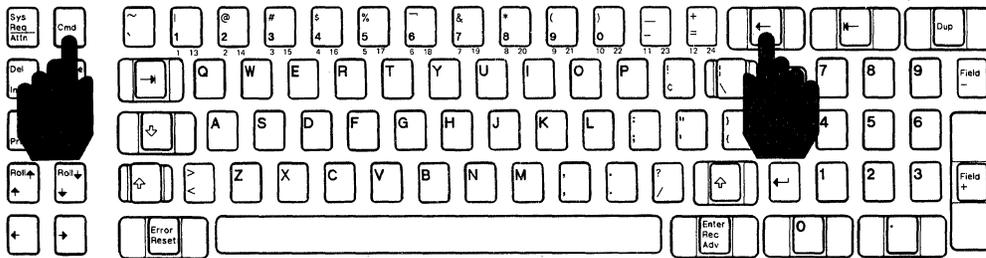
If the display station is a 3179 Model 2, a 3180 Model 2, or a 3196 without the Enhanced Keyboard, press and hold the Alt
