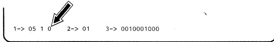
After you press the Enter key, the code that you entered in the previous section of this manual appears in field 1->. The code you just entered should appear beside the D on your display.
