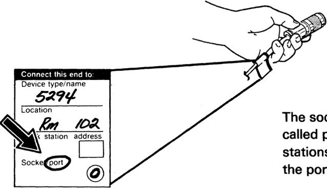
The sockets on the 5294 are called ports. Sockets on the work stations are exactly the same as the ports on the controller.
