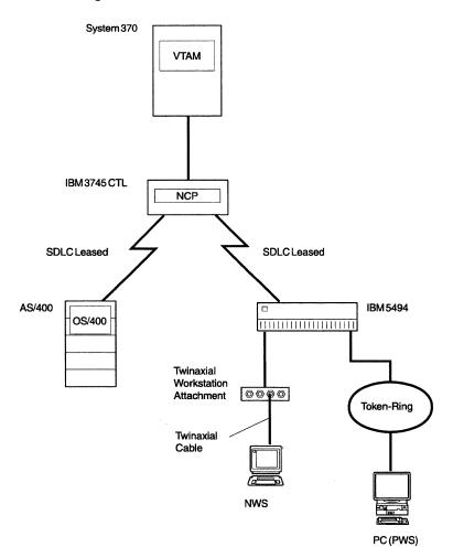
Figure C-1. Example of Physical Attachment of an AS/400 System, IBM 3745, and IBM 5494
