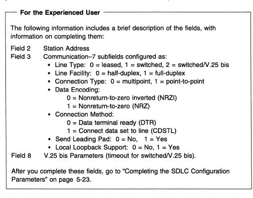
Figure 5-8. Summary of SDLC Configuration Parameters
