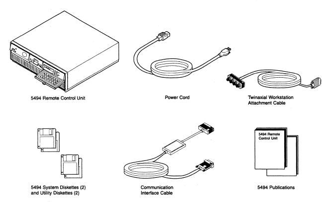
Figure 2-1. 5494 Standard Equipment Shipped with the Product
