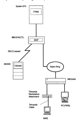
Figure C-2. Example of Physical Attachment of an AS/400 System, IBM 3745, and IBM 5494
