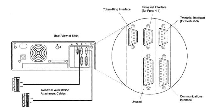
2 Find the twinaxial connector of the workstation cable that connects to port 0 on the Twinaxial Workstation Attachment cable. (The twinaxial connectors on the Twinaxial Workstation Attachment cable are called ports.) If you are using telephone twisted-pair (TTP) or IBM Cabling System cables instead of twinaxial cables, refer to the attachment cable documentation to identify your cables.
