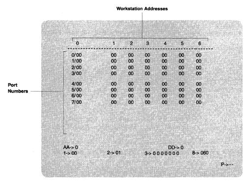
Figure 5-1. Configuration Screen for Initial SDLC Configuration
