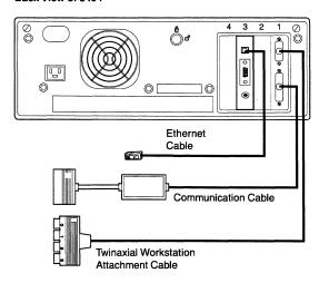
4 Connect the Ethernet cable to the Ethernet network.
