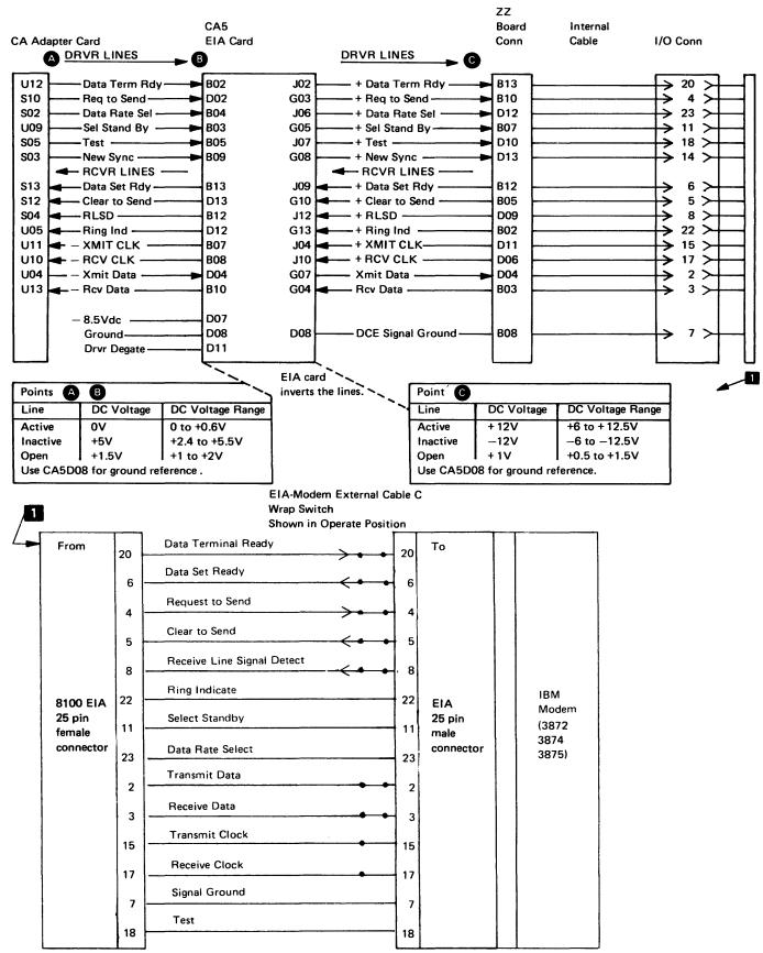
Figure CA548-1. Troubleshooting Diagram for Routine 16, EIA/Modem Data Wrap
