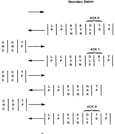
1. The primary station bids for the line by sending "ENQ". Notice framing characters (two leading Pads "LP", two synchronization characters "SYN", and trailing Pad "TP"). All messages will contain the framing sequence.
