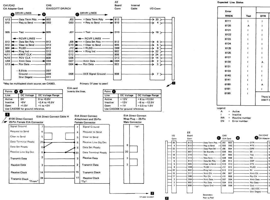
Figure CA543-1. Troubleshooting Diagram for Routine 61, EIA Direct Connect
