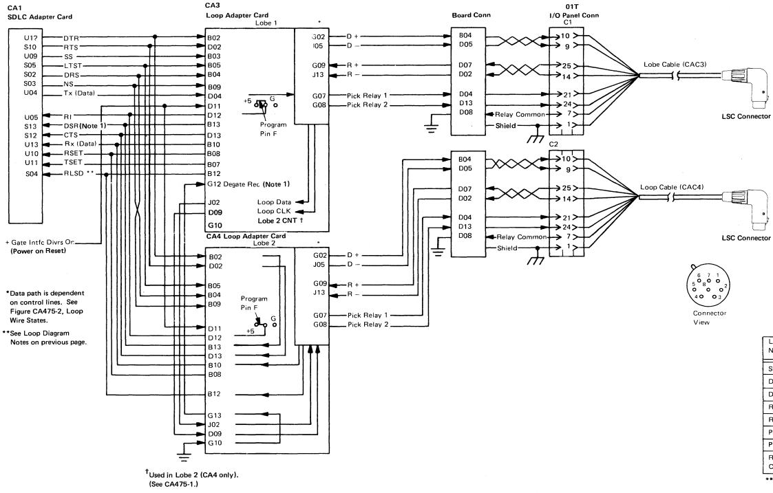
Note 1: DSR is dependent on pin G12, Degate Receive, being at ground level.
