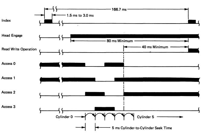
The chart below shows how a read or write operation relates to index and access timing. Note that a read or write cannot begin until at least 40 ms after the last access pulse and at least 80 ms after the rise of the Head Engage signal. Note also that the Index pulse dictates the read and write time but does not control the seek or head load (engage)
