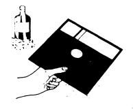
Do not place diskettes near any magnetic field. Data can be lost when exposing a diskette to magnetism.
