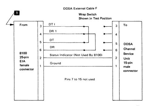
Figure CA547-1. Troubleshooting Diagram for Routine 66, DDS External Data Wrap
