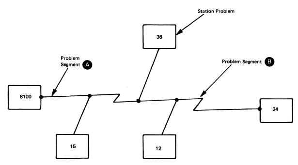
Figure CA250-2. Action Plan 18B, Data Link Fault Isolation Example
