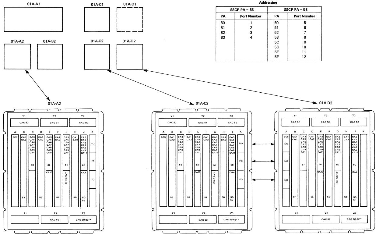
A2 Board - P/N 4939821 C2 Board - P/N 4939821 D2 Board - P/N 4939822
