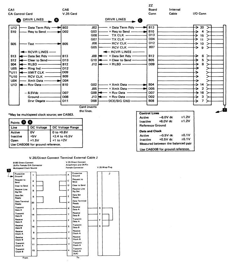
Figure CA545-3. Troubleshooting Diagram for Routine 63, V.35/ Direct Connect Terminal
