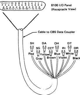
Figure CA434-2. Integrated Modem (Switched Line) Cable (CAC9)
