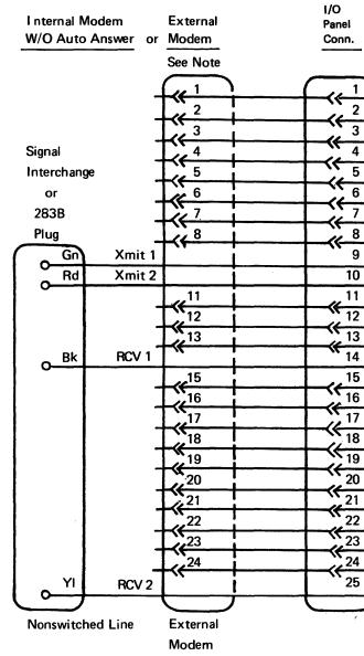
Note: West Germany has a short cable (11, 12, 16, 18, 19 wires deleted) connecting modem and cable from 8100 for D1200's modem attachment. See your TP coordinator for current requirements.
