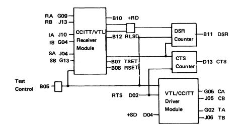
Figure CA477-1. X.21 (Nonswitched) Card (CA11) Schematic
