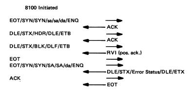
Note: In the above sequences, the 8100 enforces the flow of an EOT following an RVI. It will always send one following the receipt of an RVI. It will send one EOT as a response to a block if the host fails to send an EOT following the receipt of an RVI.
