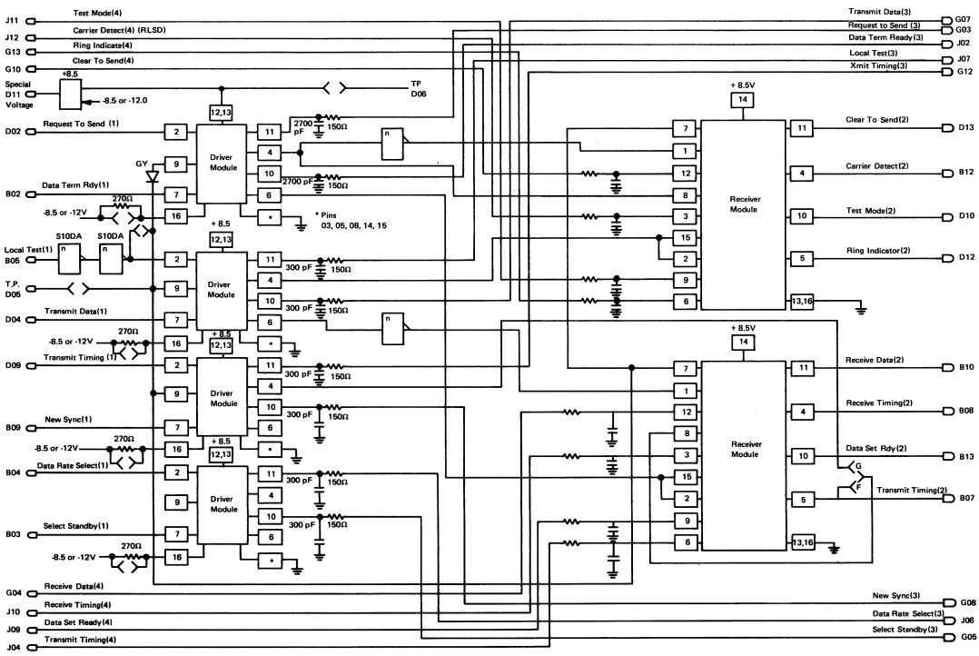
Figure CA472-1. 'EIA/CCITT Card (CA5) Schematic
