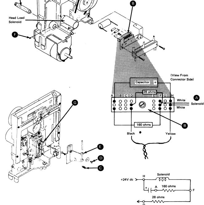
DA565 Solenoid and Bail Assembly Removal (without Connector Block)
