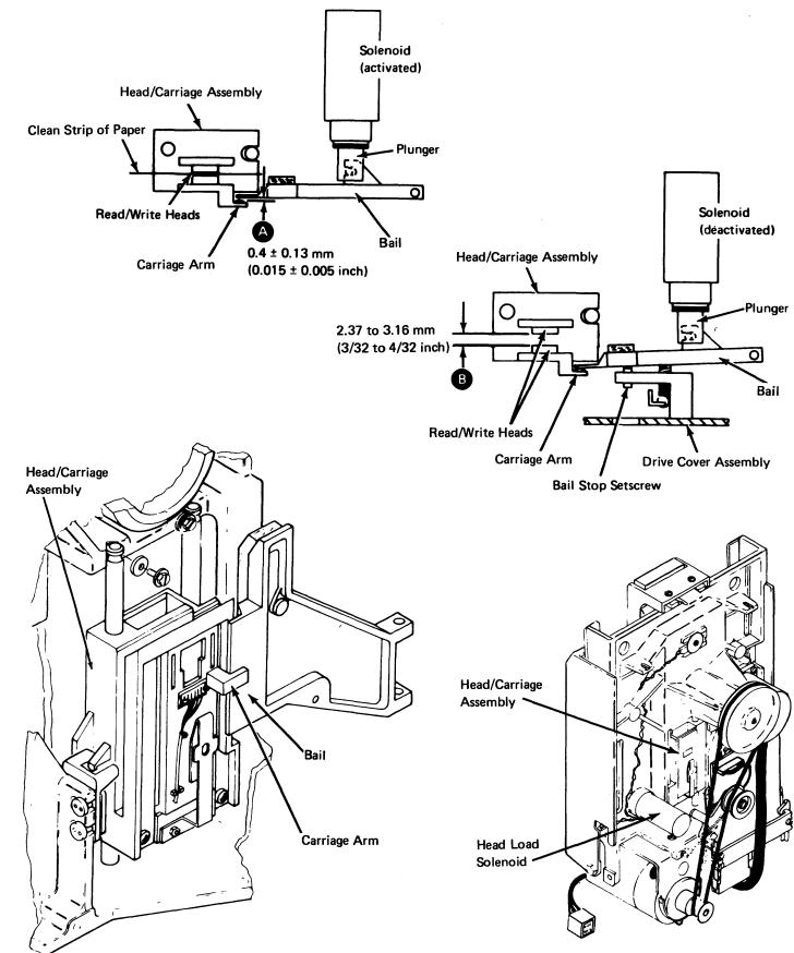
DA562 Solenoid and Bail Assembly Adjustment
