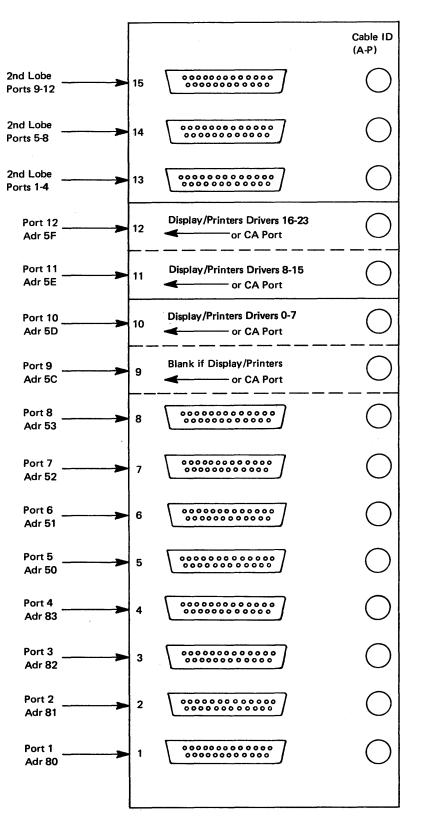
Figure CA423-1. 8140 Model BXX I/O Panel Connections (Rear View)
