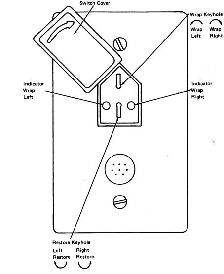
Figure CA561-1. Wrap Operation on Wrap Loop Station Connector
