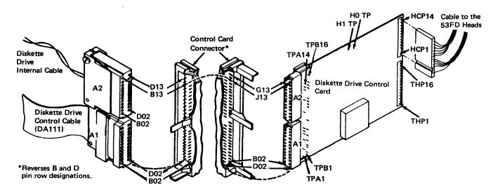
Figure DA420-3. DA3 Card, Connector, and Cable Pin Numbering
