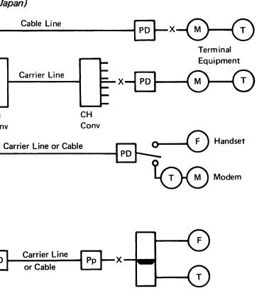
X = Maintenance Demarcation Line PD installed between Modem & Line.
