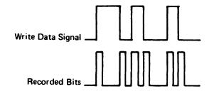
Besides the Write Data signal to determine the bit status, the adapter uses a clock pulse for bit synchronization. As the 53FD can use either FM or MFM encoding, the adapter varies the clock pulse for the encoding difference.
