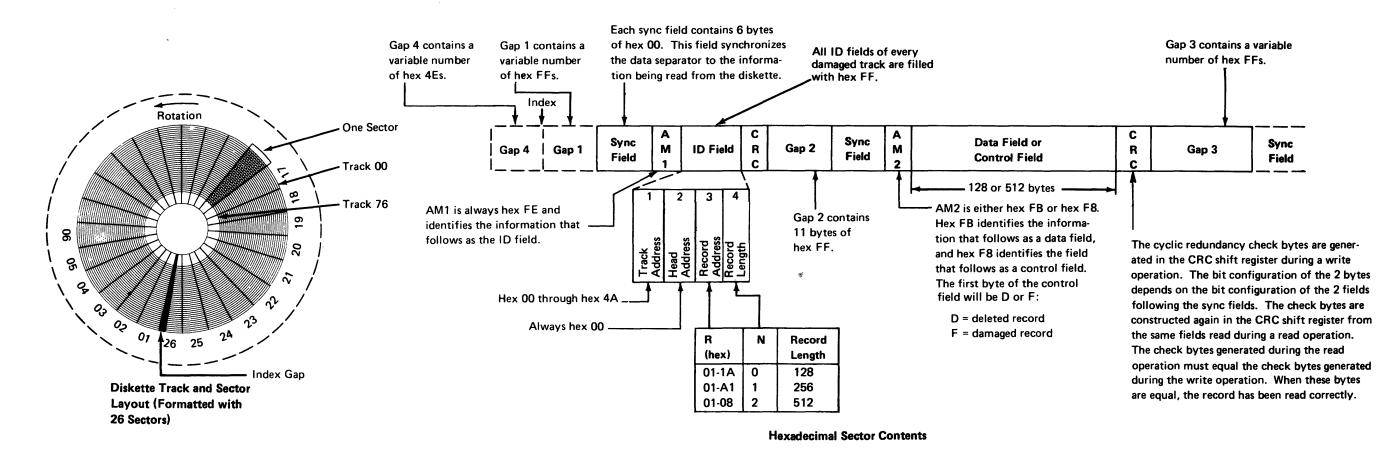
As there are 74 usable data tracks, the diskette type 1 capacity in formatted data bytes
