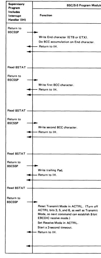
Figure CA122-4 (Part 1 of 2). BSC Transmit Operation
