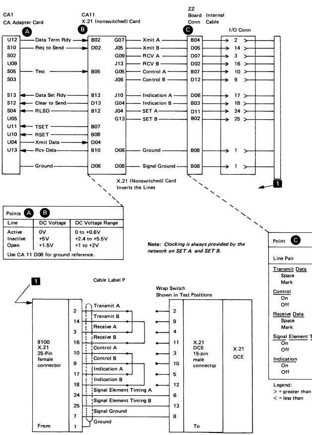
Figure CA546-1. Troubleshooting Diagram for Routine 67 and 68, X.21 (Nonswitched) External Data Wrap
