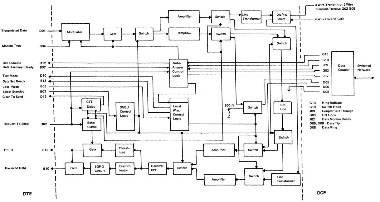
Figure CA473-1. Integrated Modem Card (CA8/CA9) Schematic
