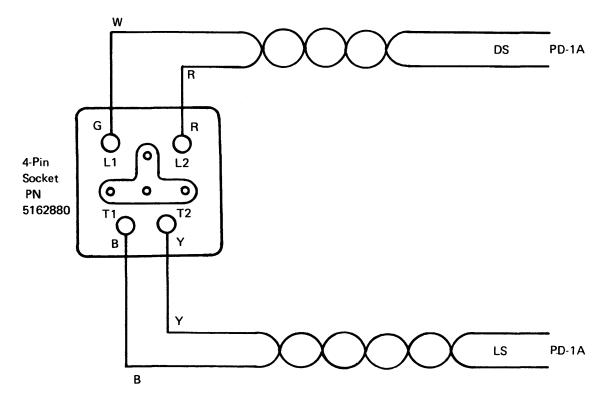
G and R connections to PD-1A terminals DS B and Y connections to PD-1A terminals LS
