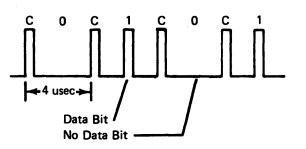
• If MFM encoding, the adapter does not use a constant clock, but generates a clock pulse only when two consecutive no-data-bit conditions occur. Therefore, the time required between a bit or no bit indication is 2 usec as follows:
