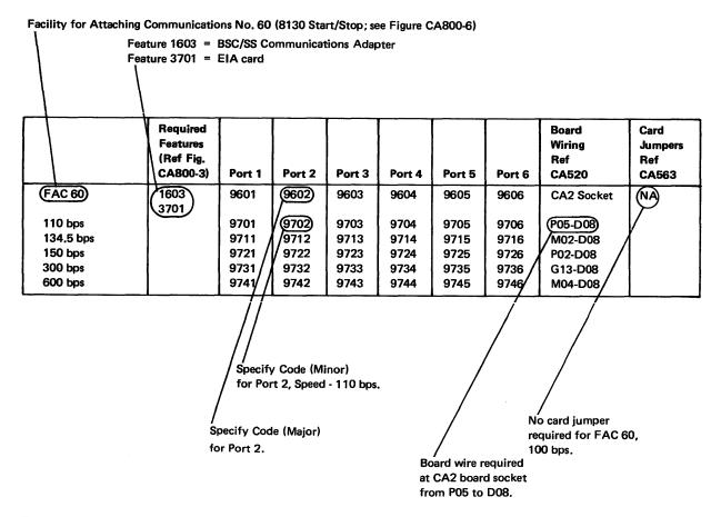
Figure CA800-2. Explanation of Communications FAC Code Table Entries; Example is for 8130 Start/Stop
