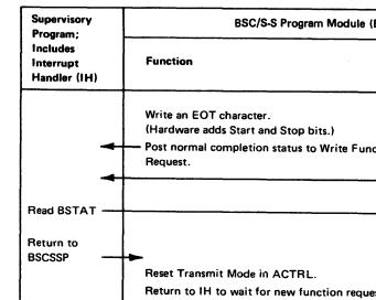
Figure CA122-6. S/S Transmit Operation
