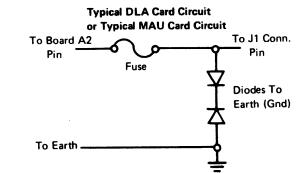
Note: When a 3277 is not attached to the 8100, the modem adapter unit (MAU) and data link adapter (DLA) cards are not used. A cable connects between A-A2Z1 and 01S-J1.
