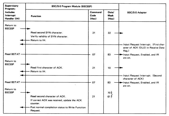
Figure CA122-4 (Part 2 of 2). BSC Transmit Operation
