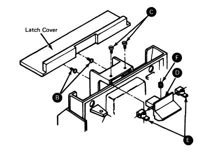
1. Remove the diskette panel cover (A) (DA520). 2. Loosen the two screws **B** and remove the latch cover.
