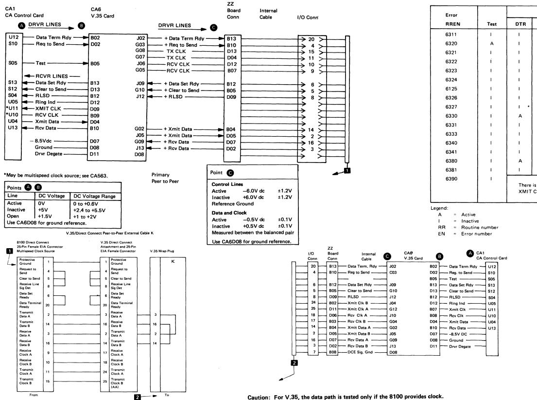
Figure CA545-4. Troubleshooting Diagram for Routine 63, V.35/Direct Connect.
