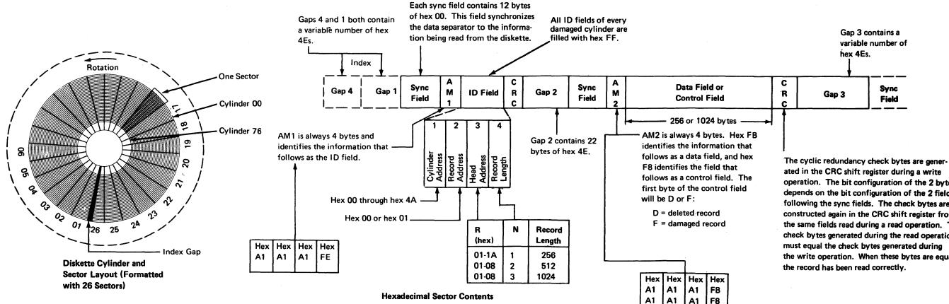
The 53FD diskette drive can record data on both sides of a diskette type 2 in FM mode, or on both sides of a diskette type 2D in either FM or MFM mode. As there are 74 usable data tracks and two tracks per cylinder, the diskette type 2D capacity in formatted
