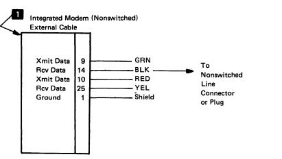
Figure CA542-1. Troubleshooting Diagram for Routine 19, Nonswitched Integrated Modem
