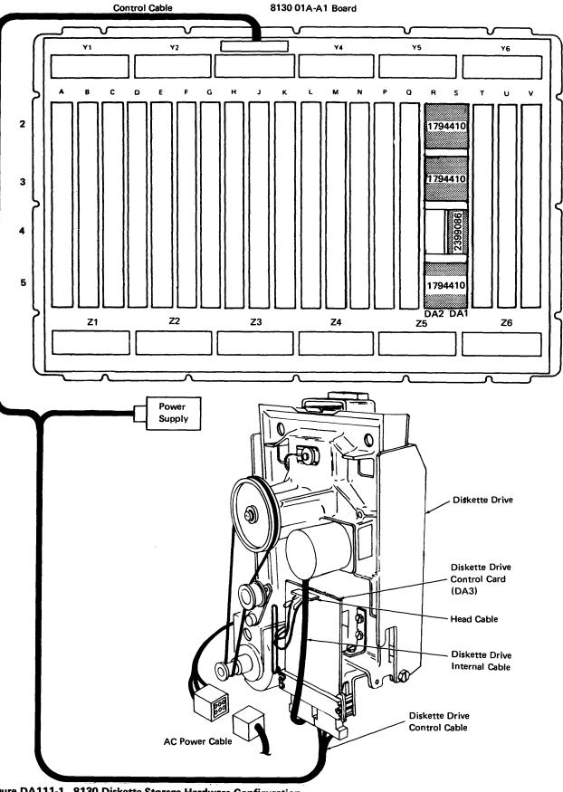
Figure DA111-1. 8130 Diskette Storage Hardware Configuration
