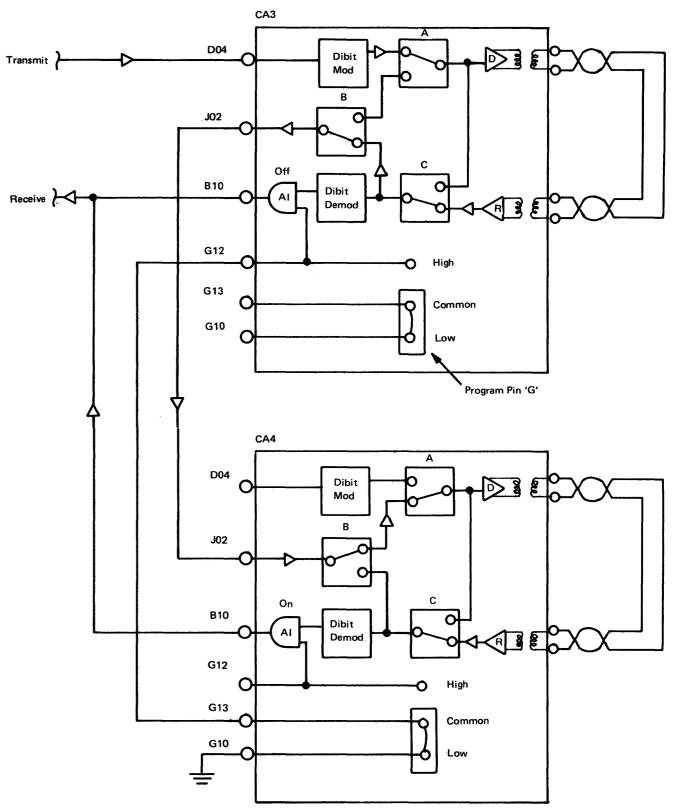
Note: Switches A and B are controlled by G10 (Lobe 2 Control). Switch C is controlled by external wrap. (All switches are logical gates; not contact switches.)
