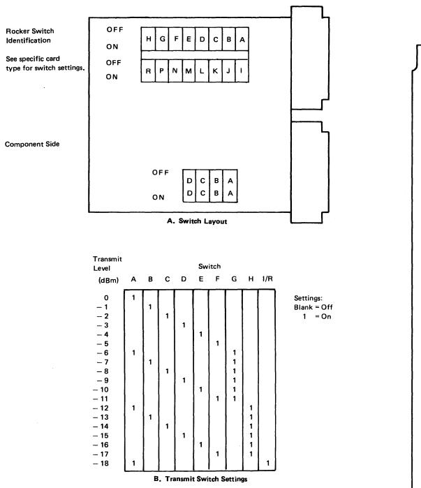
Figure CA563-2. Integrated Modem Card Type C
