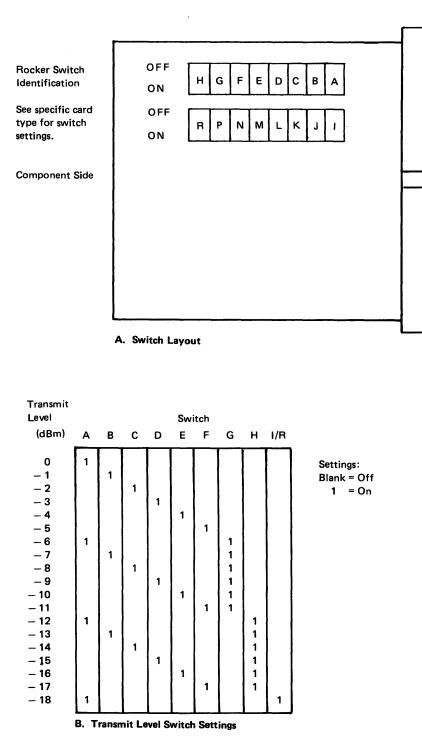
Figure CA563-1. Integrated Modem Card Type A
