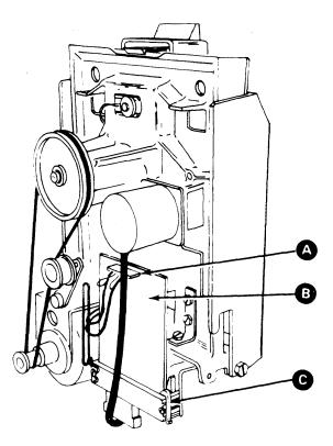
1. Carefully remove the head cable A from the DA3 card B. Remember the cable
