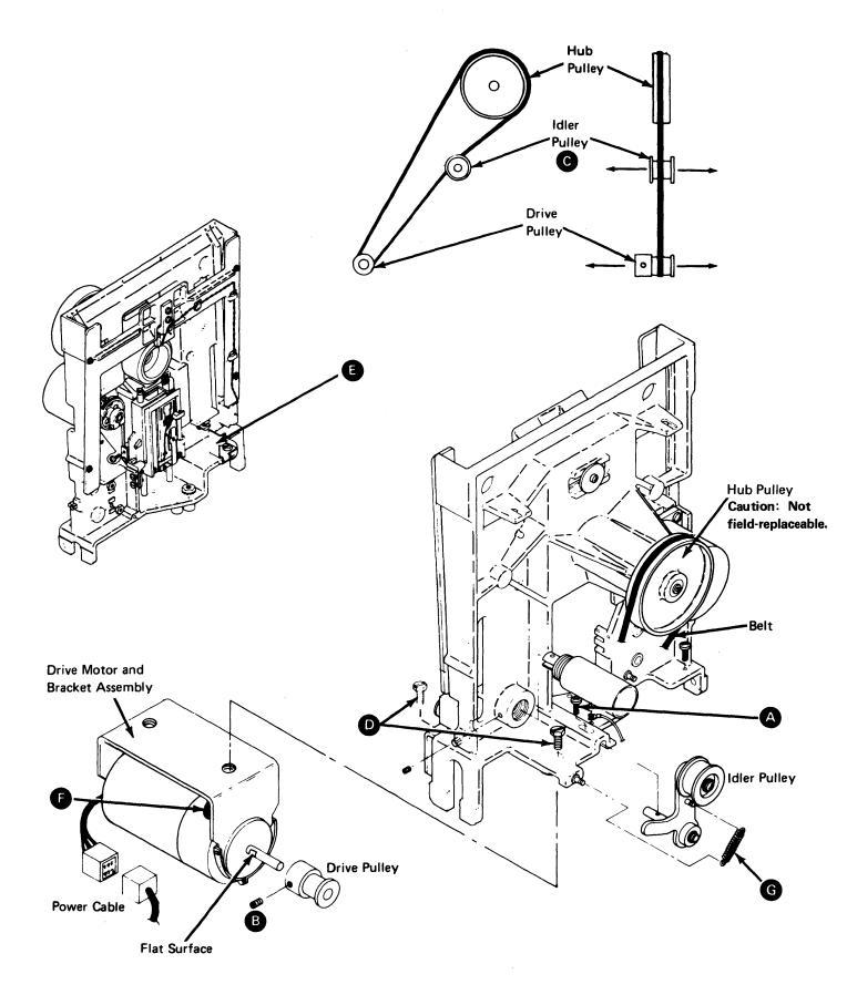
3. Remove the locking screw A and the idler assembly.
