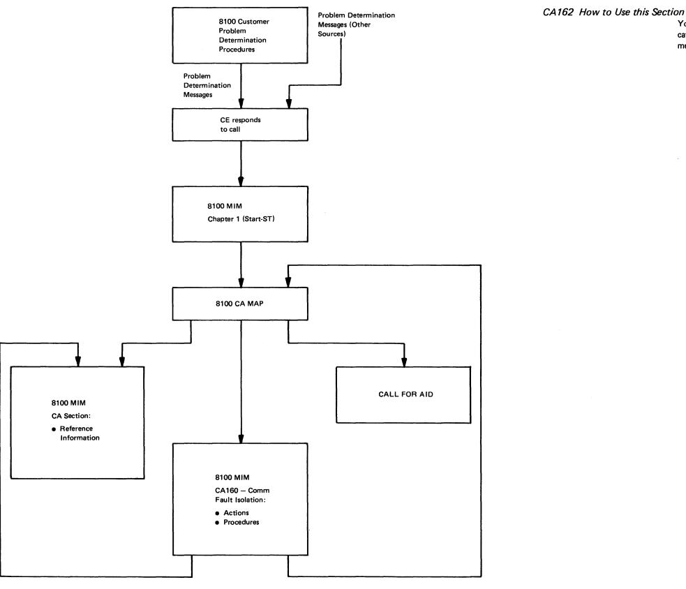
Figure CA161-1. 8100 Communications Fault Isolation Procedure
