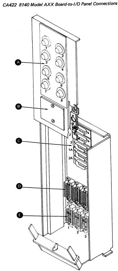
Figure CA422-1. 8140 Model AXX I/O Panel Connections (Rear View)
