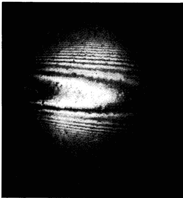
Figure 10 White light interferometric fringe pattern for a spherical head (taken from R. Tseng [11]).
