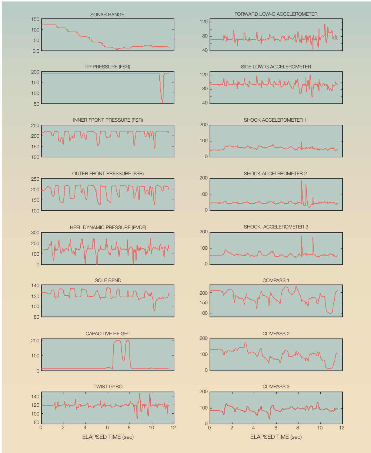
Figure 9 A sample segment of raw data showing the response of all shoe sensors for a single foot
