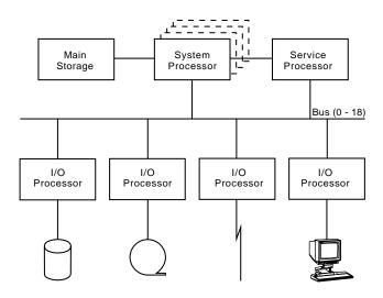
The above, simplified, drawing shows that as well as the main System Processor, there is a range of other processors, each dedicated to a particular I/O device type. What this means is that when the main System Processor encounters a request for data to be written to or read from any I/O device, that request is delegated to the particular microprocessor dedicated to that I/O device. Meanwhile, the System Processor continues with another application program.
