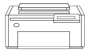
The 4232 is a heavy-duty, unattended impact dot matrix printer, capable of printing 600 characters per second (cps). It is designed for workstation printing or shared printer applications using an ASCII datastream.
