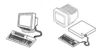
The InfoWindow II 3486, 3487, 3488 and 3489 provide a GUI–like (Graphical User Interface) capability. They also incorporate a variable split screen, calculator, an expansion cartridge enabling future IBM product enhancements or unique customer requirements to be added to the display, and both a mouse port and printer port as standard.
