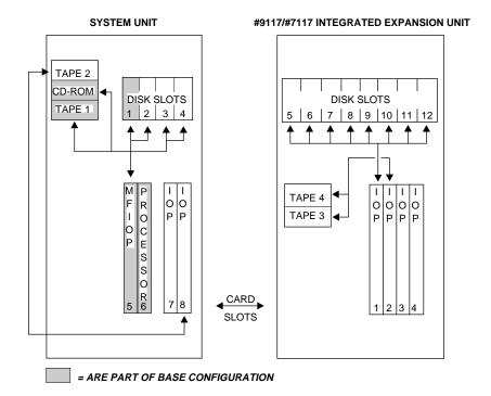
9402 Model 436 System Unit with Integrated Expansion Unit #9117/#7117.
