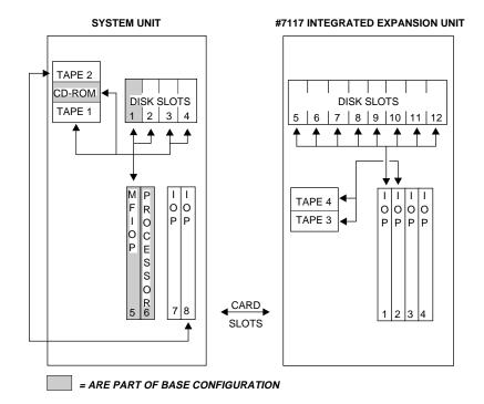
9402 Model 400 System Unit with Integrated Expansion Unit #7117.
