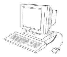
The 6250 X Terminal Family are LAN (Local Area Network) attached X terminals that connect to the AS/400 and UNIX based host platforms. They enable users to concurrently access applications and data on multiple hosts from within the X Windows\*\* environment.
