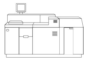
The 3829 Model 001 Advanced Function Printer is a channel attached, non-impact, all-points-addressable printer. It has 480 picture element (pel) addressability and uses an electrophotographic process to print at speeds of up to 92 pages per minute.
