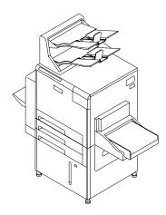
The 3130 Advanced Function Printer is a floor standing, network page-printer intended to be shared by multiple users connected to AS/400 and LANs. The 3130 will print at a maximum of 30 pages per minute, printing up to 200,000 pages per month. It also features a new high-speed RISC processor to process complex print jobs at high speed.
