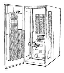
The 3494 Tape Library Dataserver is a stand-alone automated tape storage subsystem for ½" cartridges available for attachment to the AS/400. It provides an automated tape solution for automating tape operations such as save/restore, migration of data between disk and tape, and other mass-data applications.
