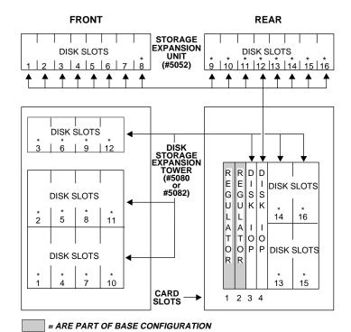
\* = ONE-BYTE DISK UNITS CANNOT BE INSTALLED IN DISK SLOT 8 THROUGH 16 OF #5052 OR SLOT 1 THROUGH 16 OF #5080 OR #5082
