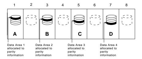
The schematic shows the eight slots available in a 9337 for disk drives. The base four disk drives are allocated to slots 1, 3, 5, and 7 and are either 1.96G or 4.19G disk drives.
