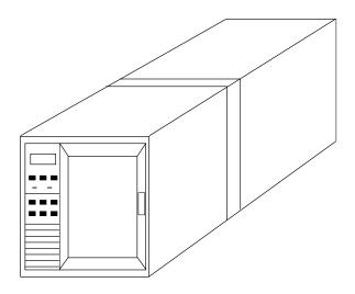
The IBM 3490E Magnetic Tape Subsystem Enhanced Capability Models E01 and E11 are reduced size rack or tabletop versions of the 3490E family of tape drives and are compatible with 3490 C10, C11, and C22 Models. They can be used as the alternate IPL device.
