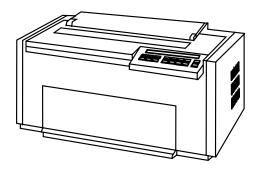
The 4230 range of printers provides heavy-duty, impact matrix printing. The six models of 4230, the 101, 111, 1S2, 102, 4S3 and 4l3 can all be twinaxially attached to an AS/400 via the 5250–type WSC (#6050). The Model 4S3 and 4l3 also offer serial and parallel attach.
