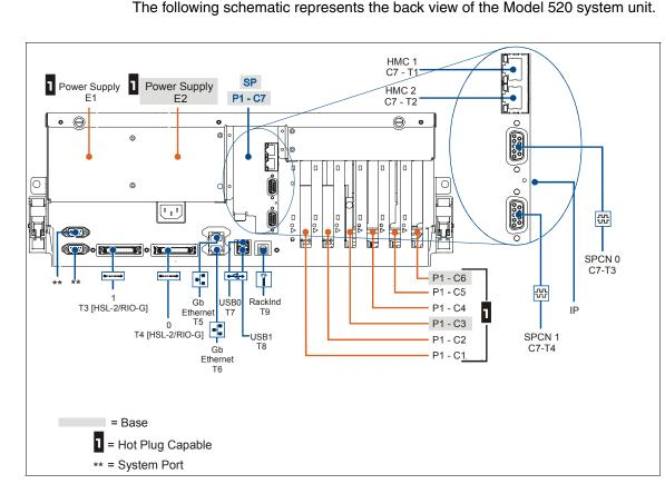
An #1827 Serial UPS Conversion Cable connects to the top system port on a rack mounted system or the right-hand system port to a deskside system.
