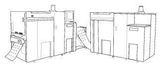
speeds from 112 to 344 impressions per minute, with the ability to perform two-up printing (8.5-by-11-inch pages) using the 17-inch print-head technology. Monthly print volumes can go up to 4.4 million impressions.
