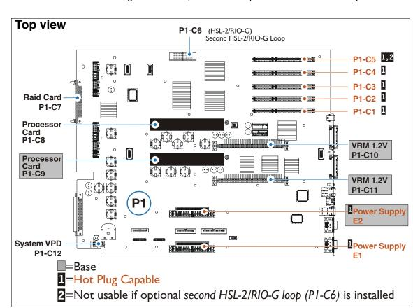
The following schematic represents the top view of the Model 550 system unit.
