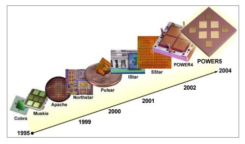
Pulsar, ISTAR, and SSTAR processors use on-chip copper-wiring technology. The Pulsar processors integrate IBM CMOS7S technology. ISTAR and SSTAR processors integrate CMOS8S technology. Previously, Northstar technology used aluminum for on-chip wiring. Copper's better conductivity permits thinner wires to be used, which enables the transistors to be packed closer together. The denser technology permits additional micro-architecture methods to improve performance.
