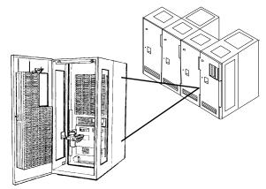
Flexible configuration choices start at a single frame configuration with up to two tape drives and up to 240 tape cartridges. Optional drives and cartridge storage can be added as needed to create an automated tape library multiple frame or tape drives, and up to 6,240 tape cartridges. Choices in tape drives for the 3494 include:
