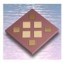
As with previous hardware technology, POWER5 technology-based processors have two load/store, two arithmetic, and one branch unit. The *processor complex* design is built in such a way that it can most efficiently execute multiple instruction streams concurrently. With simultaneous multithreading (SMT) active, instructions of two different threads can be issued per single cycle.
