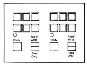
Figure 7. 3370 Operator Panel (Design Model)
