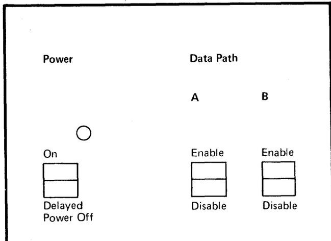
Figure 8. Controller Operator Panel
