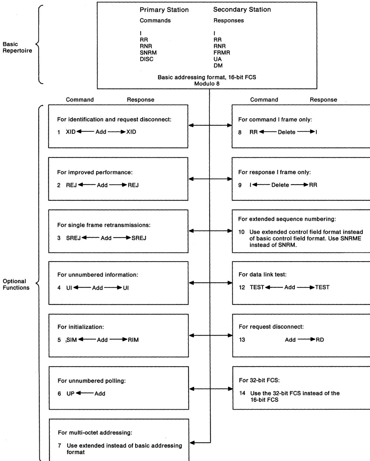
Figure 33. HDLC Unbalanced Normal Class of Procedures
