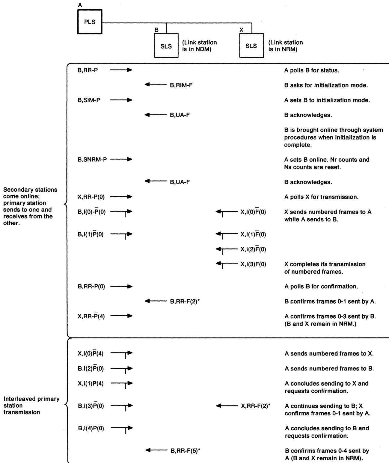
Figure 27. Two-way Simultaneous Exchanges on Nonswitched Multipoint Links
