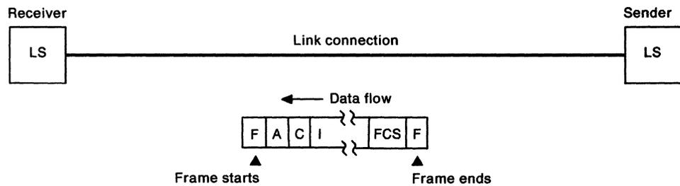
Figure 12. SDLC Transmission Frame
