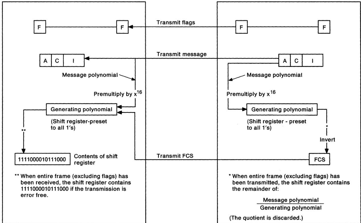
Figure 32. CRC Operation with SDLC
