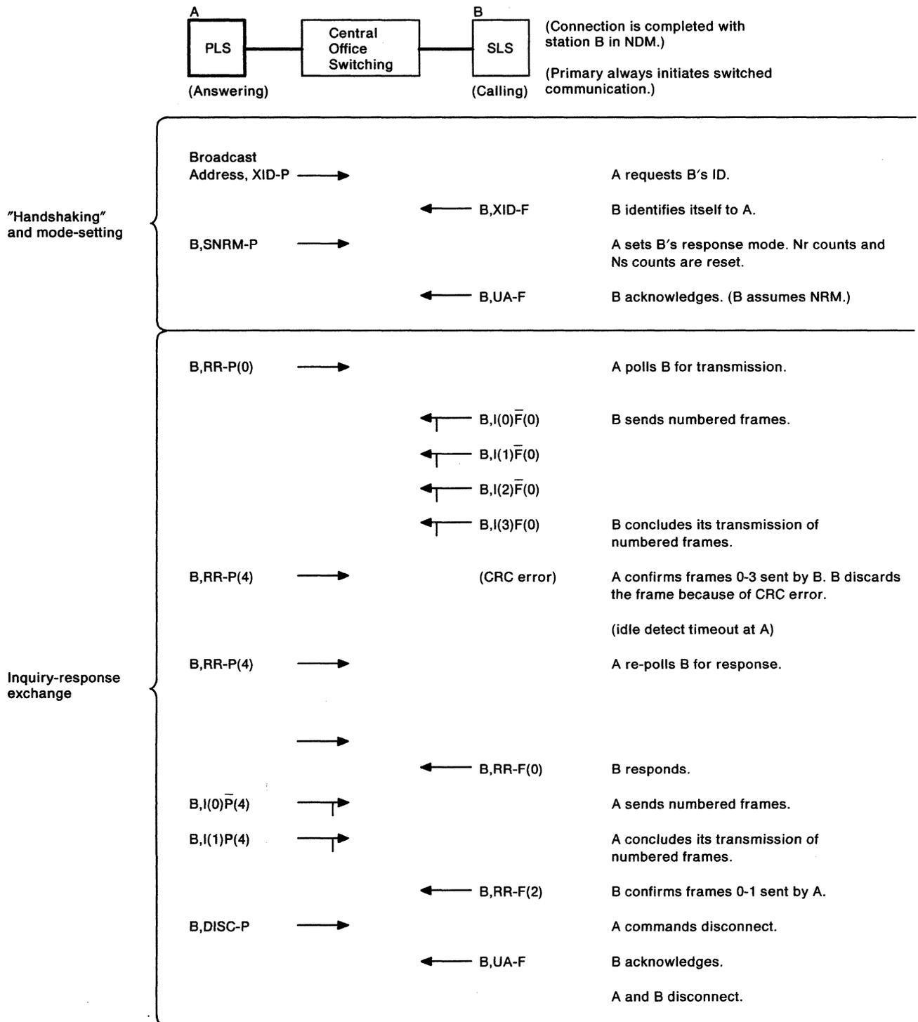
Figure 28. Two-way Alternate Exchanges on Switched Point-to-Point Links
