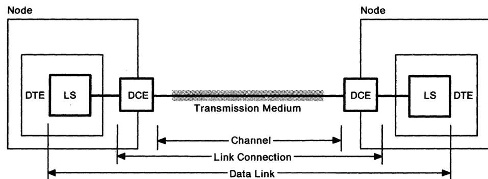
DCE Data Circuit-terminating Equipment
