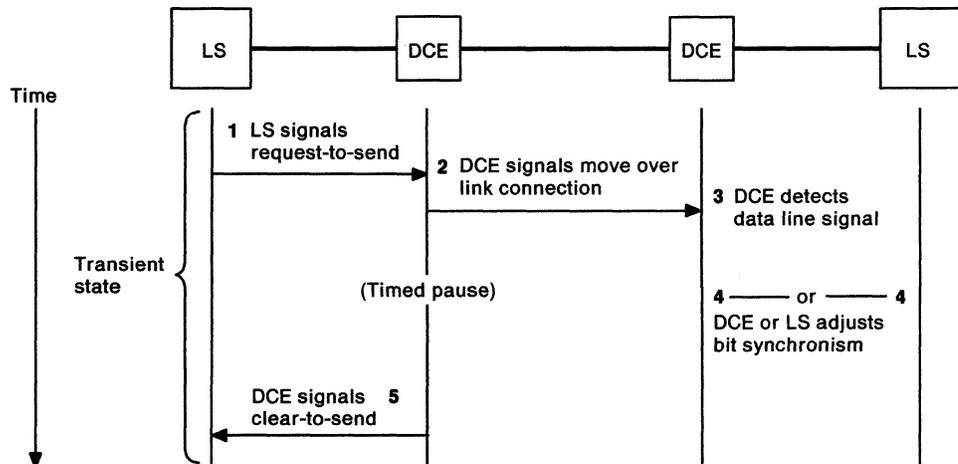
DCE Data Circuit-terminating Equipment
