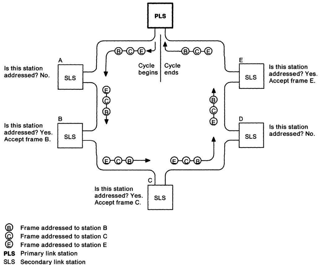
Figure 22. SDLC Loop Exchanges: Primary Station Transmitting
