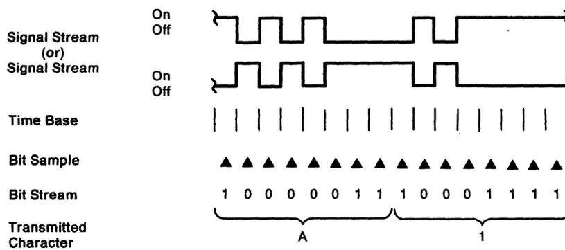
Figure 9. Invert-on-Zero Transmission Coding
