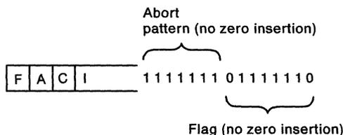
Figure 18. Transmitting Station Aborts Transmission
