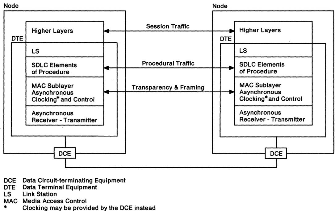
Figure 35. Asynchronous SDLC Layering
