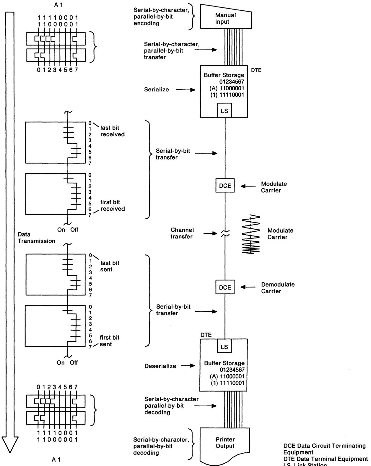
Figure 5. Data Conversion for Data Link Transfer
