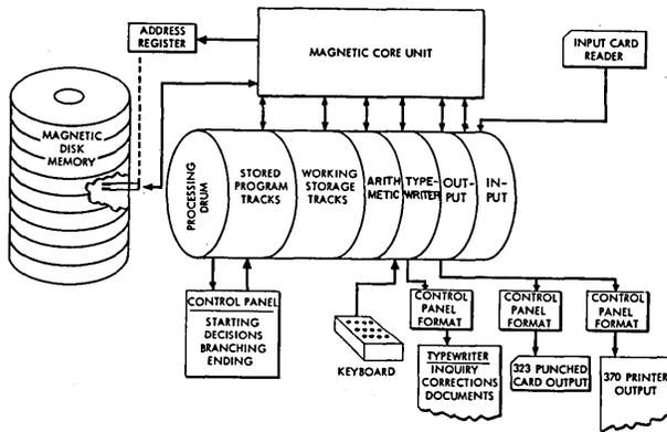
Schematic of IBM 305 RAMAC
