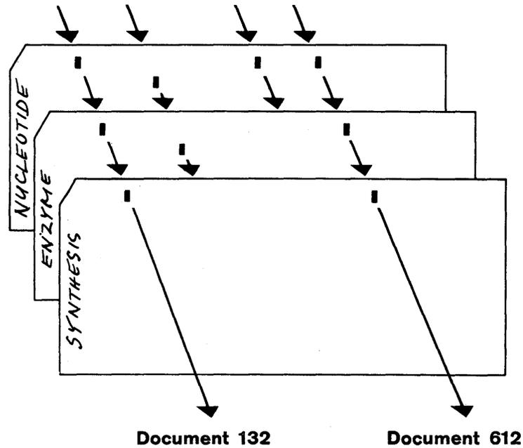
Position coding of document numbers. Where the beam from a light source shines through the selected cards, the hole represents a document indexed under the descriptors stated in query.
