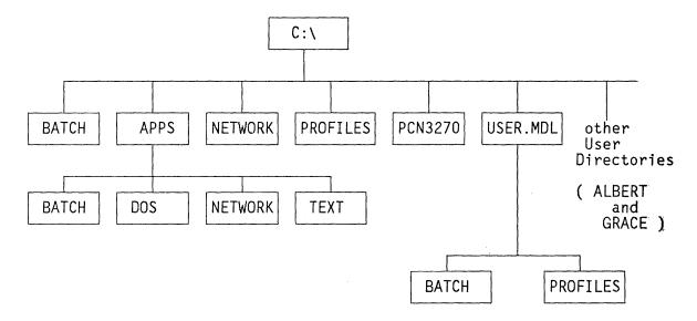
Figure 26. PC Network Server Disk Structure
