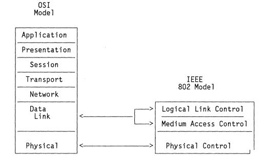
Figure 3. OSI Reference Model and IEEE 802 Local Model Relationship
