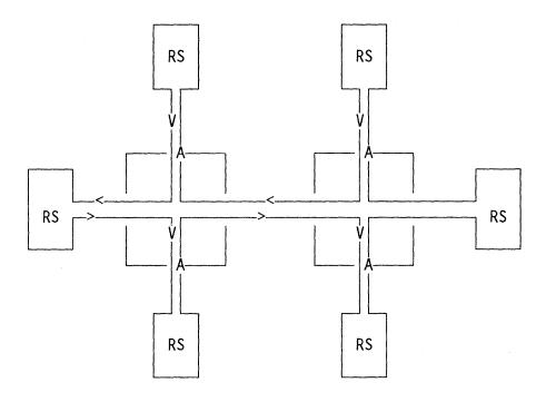
Figure 2. Star-Wired Ring with Two Wiring Concentrators.
