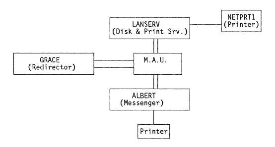
Figure 7. Sample PC Network Configuration
