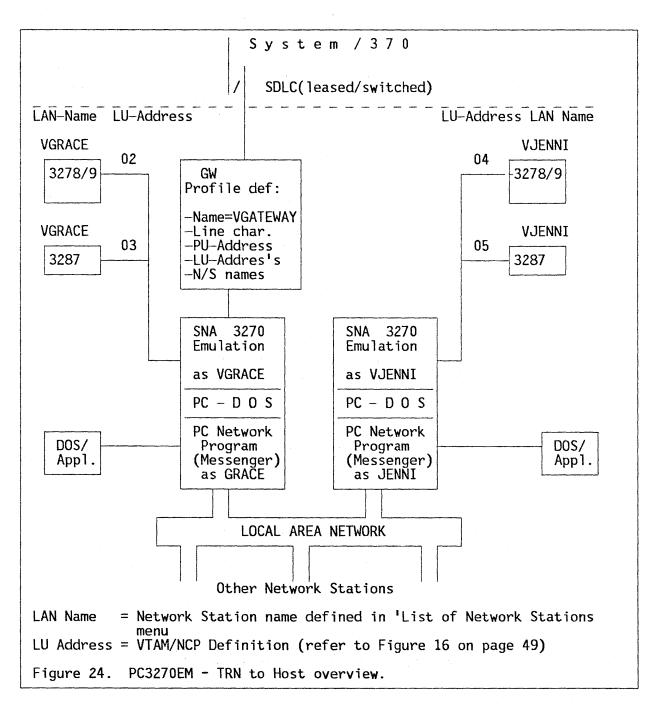
As can be seen in the figure, the gateway provides the only physical link to the Host, and controls all of the Host-LAN communications for the LAN attached N/S's. The LAN Administrator would probably want to define the gateway with the help of Host System Administrator. The various setup definitions reflect:
