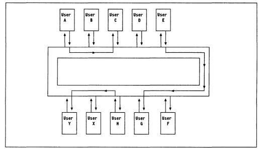
Figure 96. Multiple Simultaneous Communications on a Ring Topology
