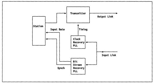
Figure 5. Clock Recovery in Primary Rate ISDN. Two PLLs are used because of the different requirements of bit stream recovery and clock recovery.
