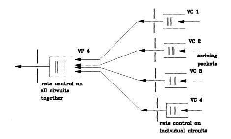
Figure 26. A Cascade of Leaky Buckets. Leaky bucket rate control is applied to individual circuits and then to the total of a logical group.
