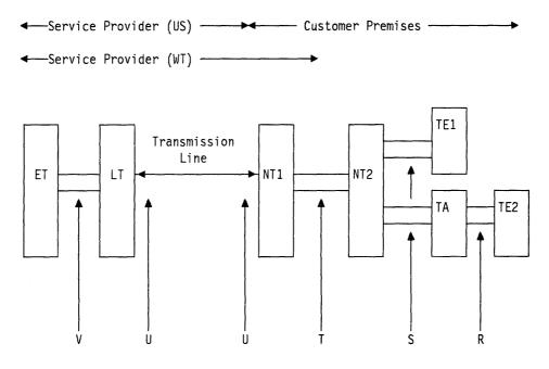
Figure 34. ISDN Reference Configuration
