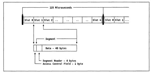
Figure 82. DQDB Frame Format as Seen by the DQDB Protocol Layer. Not shown is a 4-byte slot prefix used by the physical layer.
