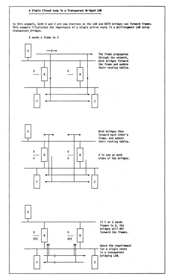
Figure 114. Closed Loops in a Transparent Bridging Environment
