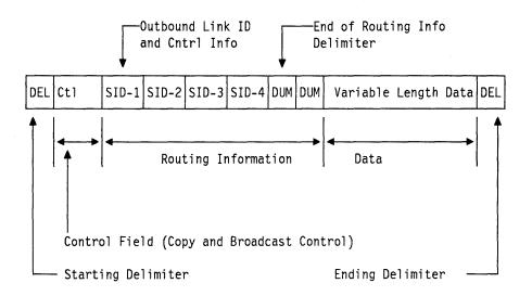
Figure 62. Data Packet Format
