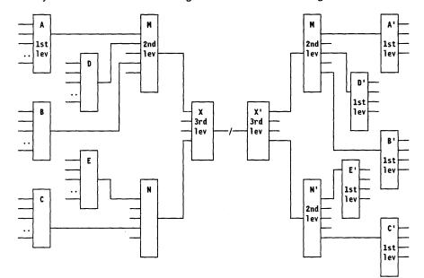
Figure 39. The Multiplexor Mountain. Each multiplexor illustrated exists as a separate physical device although many multiplexors may be mounted together on a single rack.
