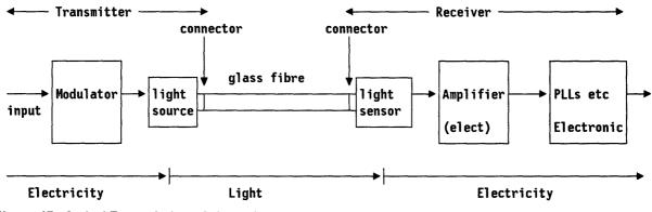
Figure 17. Optical Transmission - Schematic
