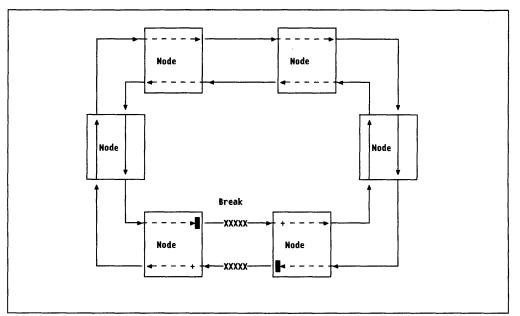
Figure 90. DQDB Reconfiguration. Each node is able to be a slot generator. Here, the bus has been broken and the two nearest nodes have taken over the role of head of bus.
