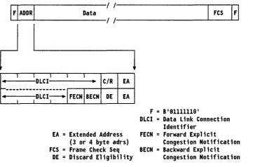
Figure 55. Frame Format. Link control fields are absent since they are ignored by the network.
