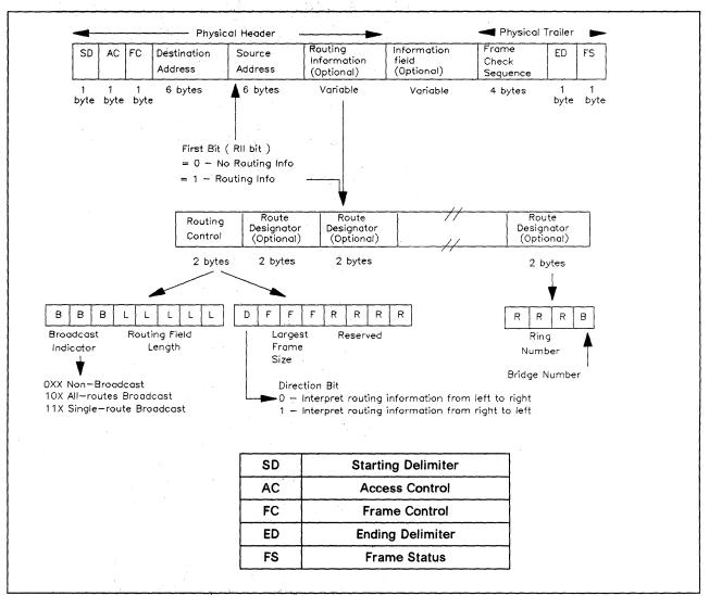
Figure 110. Routing Information of a Token-Ring Frame
