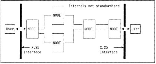
Figure 124. Schematic of a Packet Network. Each "node" (or "switch") receives a packet in full before routing it on towards it destination user. Not shown is the additional equipment necessary to manage the network.
