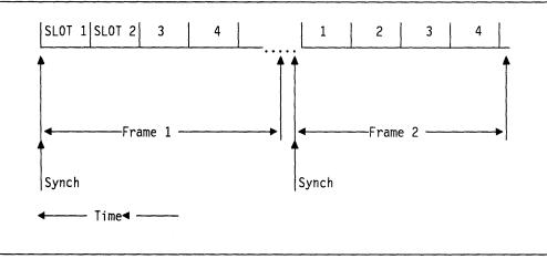
Figure 120. Time Division Multiplexing Principles
