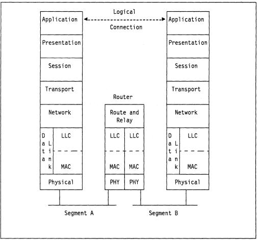
Figure 118. Model for a Router. Relationship between the OSI seven-layer model and a model for a router.
