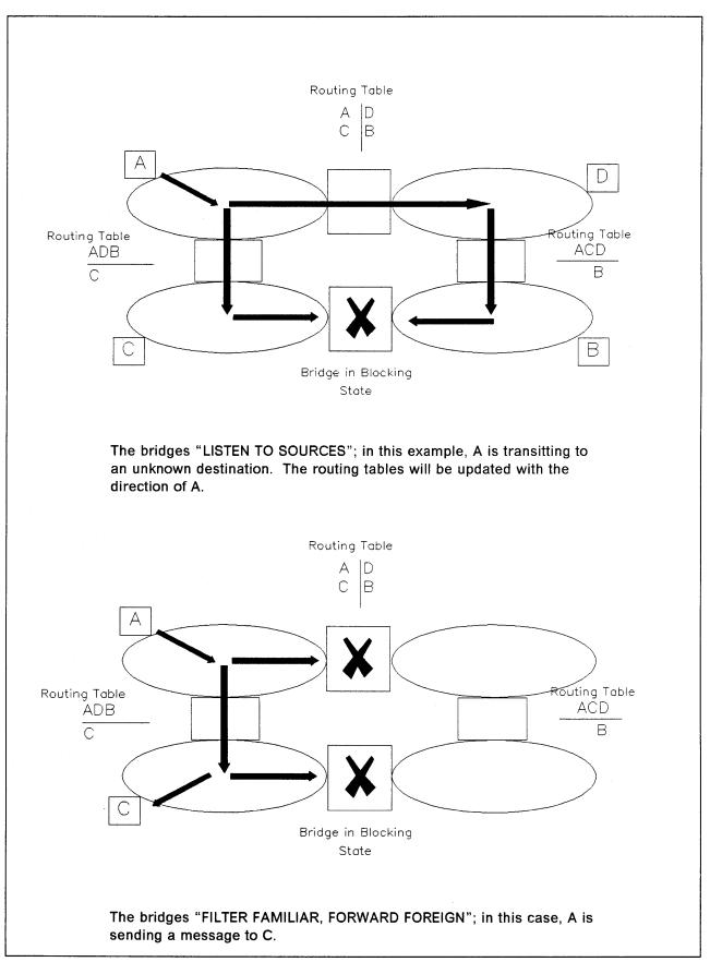
Figure 113. Routing in a Multisegment LAN Using Transparent Bridges
