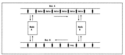
Figure 86. DQDB Fairness. Problem is propagation delay along the bus.
