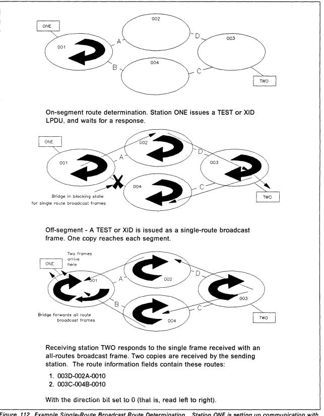
Figure 112. Example Single-Route Broadcast Route Determination. Station ONE is setting up communication with station TWO.
