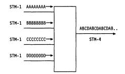
Figure 43. STM-1 to STM-4 Synchronous Multiplexing
