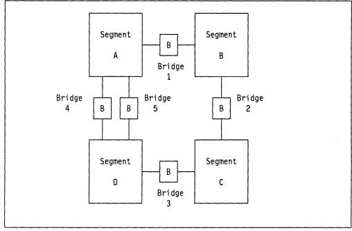
Figure 109. An Example of a Multisegment LAN
