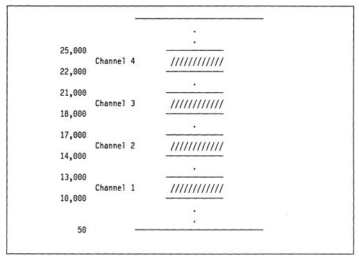
Figure 119. The Concept of Frequency Division Multiplexing. The physical carrier provides a range of frequencies called a "spectrum" within which many channels are able to co-exist. Notice the necessary "buffer zones" between frequency bands.
