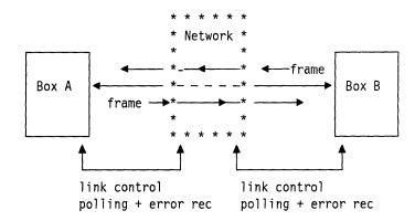
Figure 53. Frame Switching. The network viewed from Box A "looks like" Box B but polling and error recovery are handled locally and do not pass through the network.
