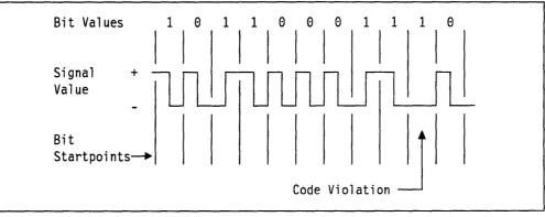
Figure 11. Differential Manchester Coding Example. The presence or absence of a transition **at the bit start point** determines whether the bit is a one or a zero. A code violation occurs when the signal state does not change at the middle of a bit time.
