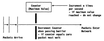
Figure 25. Leaky Bucket Rate Control
