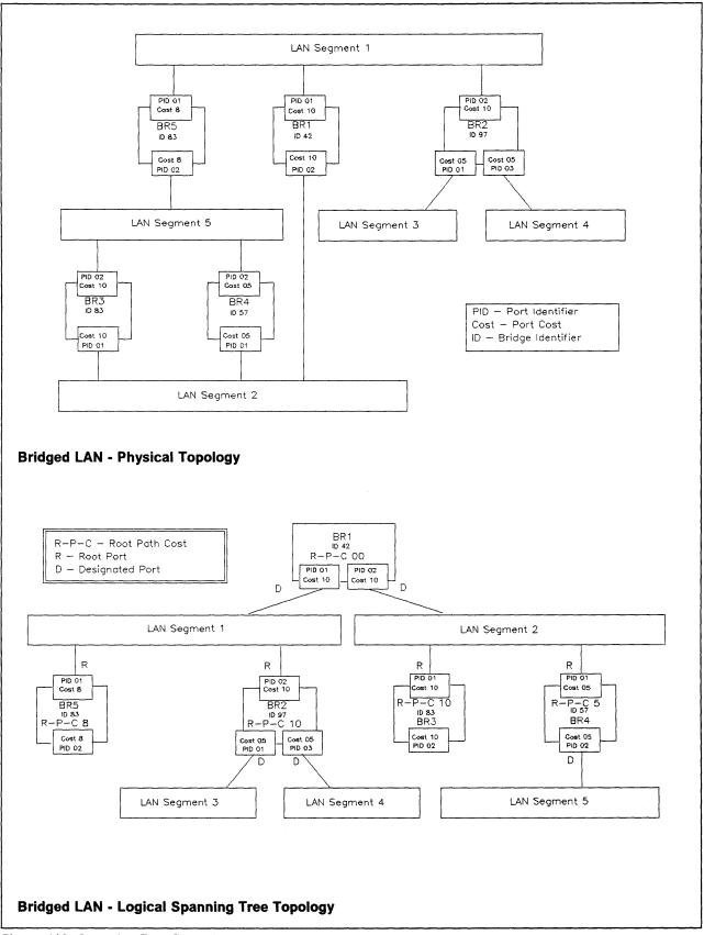
Figure 116. Spanning Tree Example
