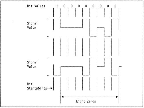
Figure 9. B8ZS Substitutions. Either of two alternative strings are used depending on the polarity of the preceding one bit.
