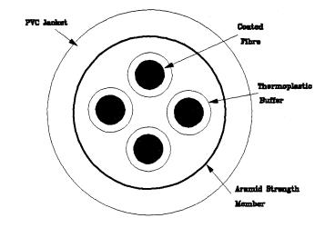
Figure 21. Typical Fibre Cable
