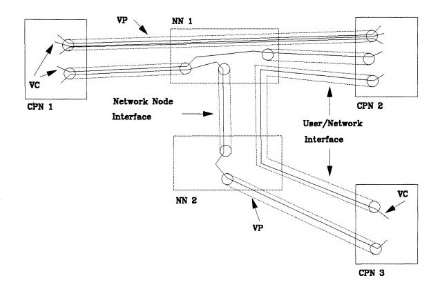
Figure 47. Routing Concept in an ATM Network. Physical links between nodes are not shown.
