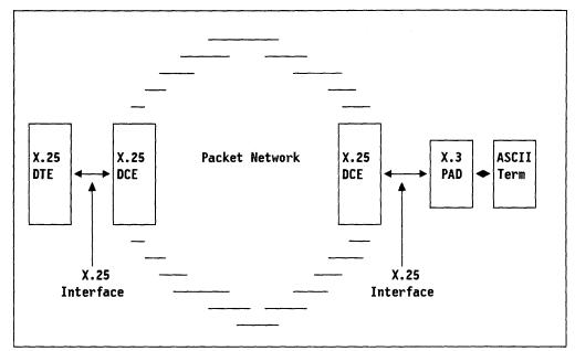
Figure 129. An "External" PAD. While described as a network function the PAD is most often implemented as an external piece of equipment.
