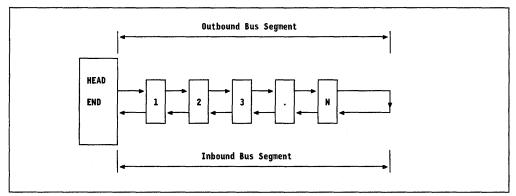
Figure 101. CRMA Folded Bus Configuration
