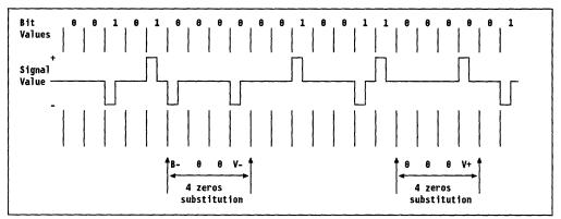
Figure 8. Zeros Substitution in HDB3
