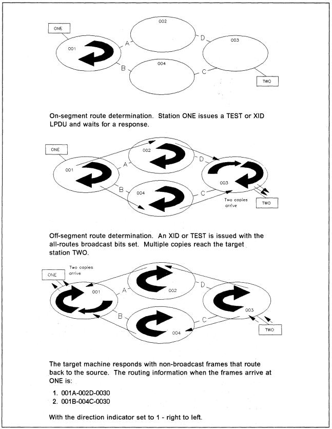
Figure 111. Example All-Routes Broadcast Route Determination. Station ONE is setting up communication with station TWO.
