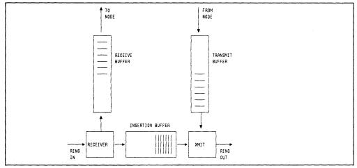
Figure 106. Principle of Buffer Insertion
