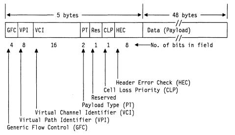
Figure 49. ATM Cell Format at User Network Interface (UNI)
