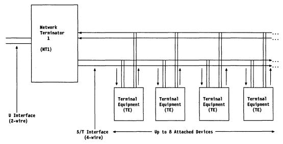
Figure 36. ISDN Basic Rate Passive Bus
