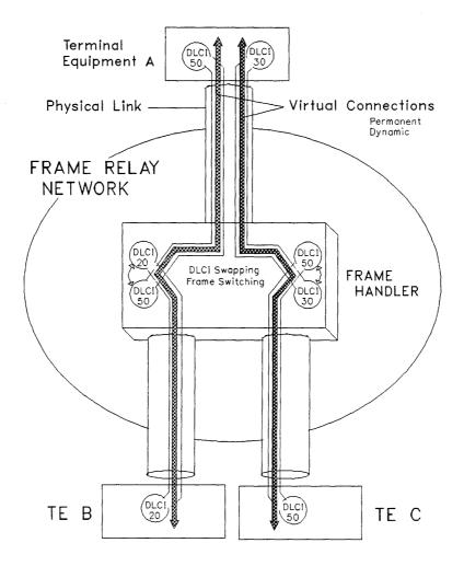
Figure 56. Frame Relay Routing Scheme
