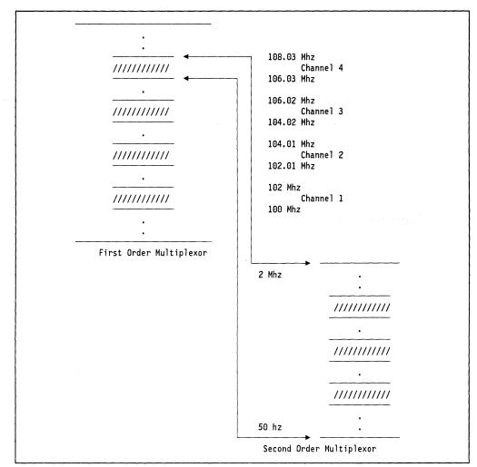
Figure 121. Sub-Multiplexing Concept. Frequency division technique used within frequency division derived channel.
