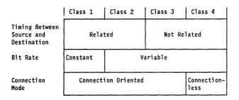
Figure 52. Characteristics of Service Classes in the ATM Adaptation Layer
