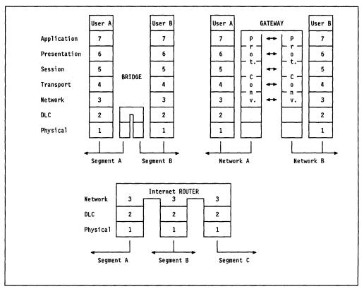
Figure 108. Network Interconnection Techniques (Based upon OSI Reference Model Layers 1 - 7)
