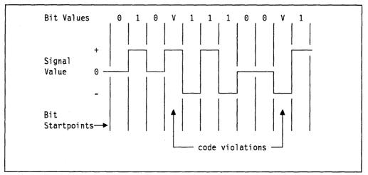
Figure 7. Code Violation in AMI Coding. A violation is a bipolar pulse of the same polarity as the preceding bipolar pulse.
