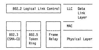
Figure 58. Frame Relay in Relation to IEEE Standards. Frame Relay functions as an alternative MAC layer which is used by the logical link control and medium access control functions.
