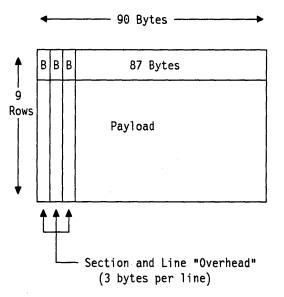
Figure 40. Sonet STS-1 Frame Structure. The diagramatic representation of the frame as a square is done for ease of understanding. The 810 bytes are transmitted row by row starting from the top left of the diagram. One frame is transmitted every 125 microseconds.
