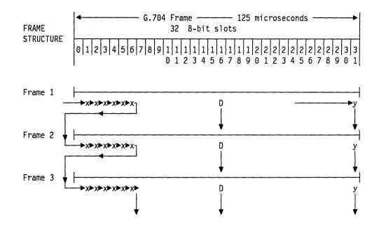
Figure 38. ISDN Primary Rate Frame Structure (Europe). Arrows show the sequence of slot concatenation for an H0 (wideband) channel, the D channel (slot 16) and a B channel (slot 31).
