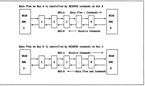
Figure 103. CRMA Dual Bus Configuration. The system is logically two separate parts. Data flow on one bus is controlled (allocated) by RESERVE commands on the other bus.
