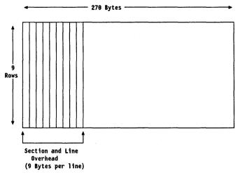
Figure 44. SDH Basic Frame Format
