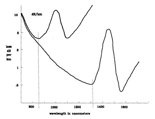
Figure 18. Typical Fibre Infrared Absorption Spectrum. The upper left-hand curve represents the characteristics of Silicon Dioxide (SiO<sub>2</sub>) glass. The lower (much better) curve shows a curve for a glass made from a mixture of Germanium Dioxide (GeO<sub>2</sub>) and Silicon Dioxide. The peak at around 1450 nm is due to the effects of traces of water in the glass.
