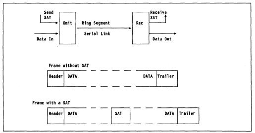
Figure 98. The SAT Control Signal
