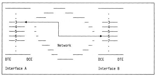
Figure 126. Virtual Circuit. Two logical channels (number 3 on interface A and number 6 on interface B) are communicating with one another. This pairing of logical channels is called a virtual circuit.
