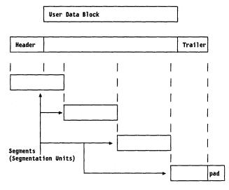
Figure 87. Segmentation of a Data Block to Fit into a Slot (Cell)
