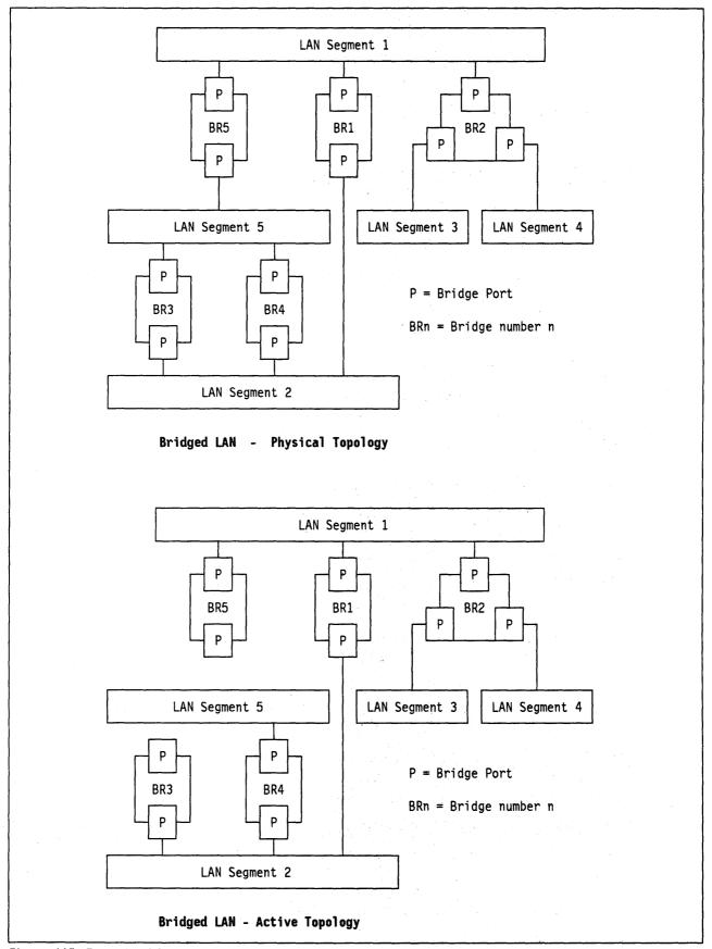
Figure 115. Example of Physical Topology and a Possible Active Spanning Tree Topology
