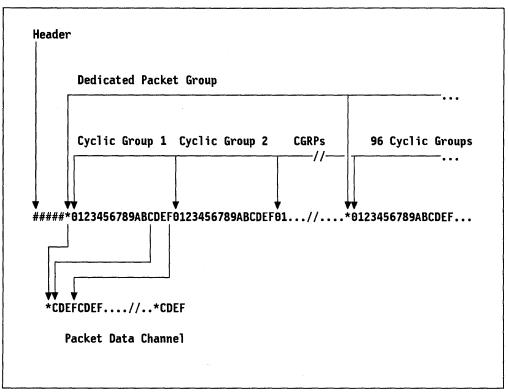
Figure 80. Derivation of Packet Data Channel from the TDM Frame. In this example WBCs 12 to 15 (labelled C, D, E and F) are concatenated with the DPG to form the packet data channel.
