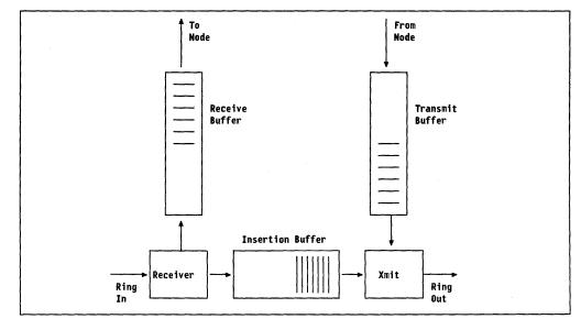
Figure 97. Buffer Insertion
