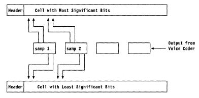
Figure 29. Assembly of Packets for Priority Discard Scheme
