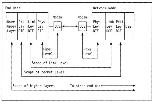
Figure 127. DTE and DCE Relationships. The scope of each layer is shown here. The relationship between DTE and DCE at each layer should be noted.
