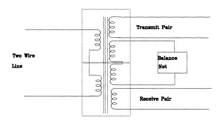
Figure 16. Hybrid Balanced Network. This device is used to convert a signal from two-wire to four-wire operation. Two transformers each consisting of at least three tightly coupled windings and an impedance balancing network are used. The balance network is adjusted to match the impedance of whatever device is connected to the two-wire line. With careful impedance matching, the device can reduce the level of the transmitted signal reaching the receive pair by as much as 50 dB.
