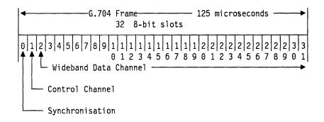
Figure 94. G.704 Frame Structure as Used by Fastpac Interface
