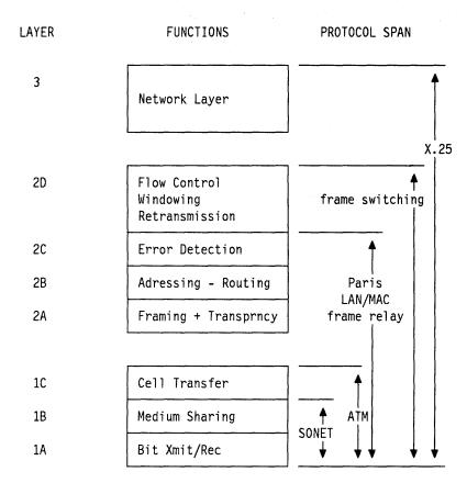
Figure 33. Protocol Span of Packet Networking Techniques
