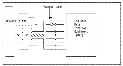
Figure 125. Elements of the X.25 Interface
