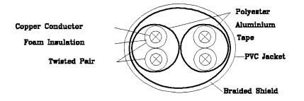
Figure 13. IBM Type 1 Shielded Twisted Pair. Each of two twisted pairs is shielded from the other by an earthed polyester aluminium tape shield. The whole is further shielded in copper braid.
