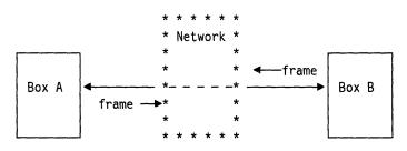
If we want to place a network between Boxes A and B as illustrated above, then there are many alternatives. Typically in the front of the user data message there will be a set of network protocol headers. We could:
