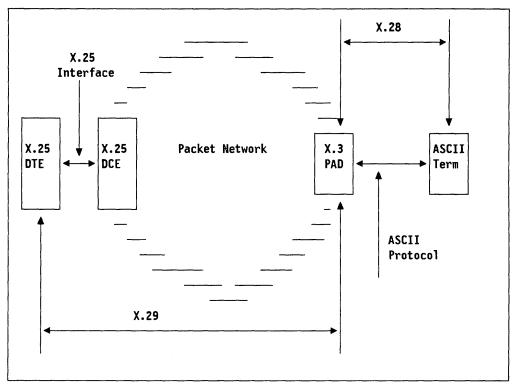
Figure 128. The ASCII "PAD". Scope of the three CCITT recommendations X.3, X.28 and X.29 is shown.
