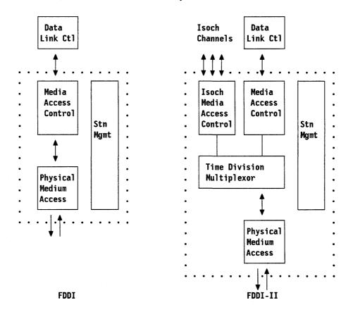
Figure 78. FDDI and FDDI-II Conceptual Structure. In FDDI-II a time division multiplexor is used to divide the LAN into multiple bit streams. For data transport one of the bit streams is mediated using FDDI access control protocols unchanged.
