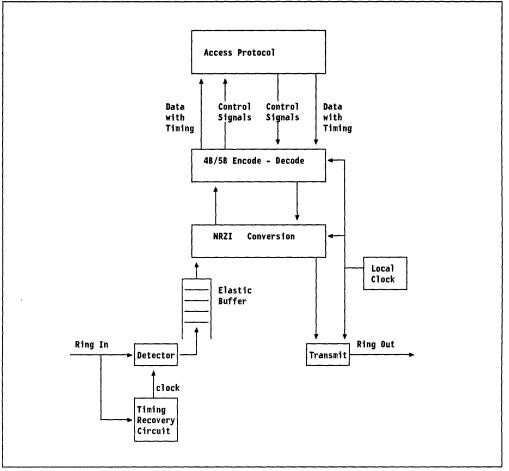
Figure 76. Physical Layer Structure
