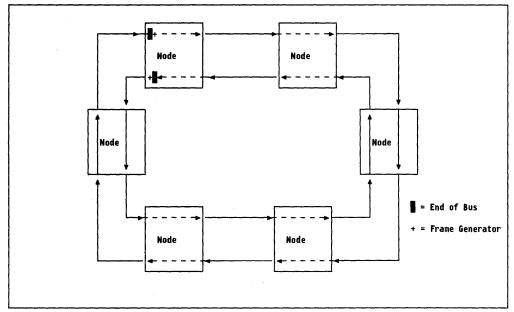
Figure 89. DQDB Looped Bus Configuration. In this configuration one node doubles as the slot generator and the busses are looped into a ring configuration.
