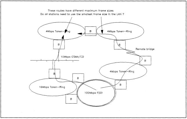
Figure 117. Maximum Frame Size Supported by Multiple Routes
