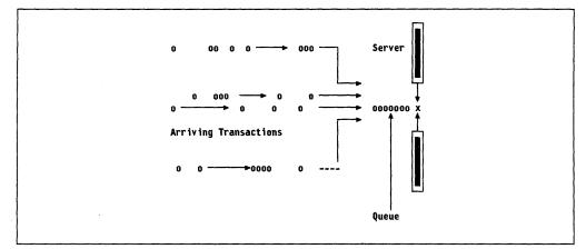
Figure 122. Schematic of a Single Server Queue
