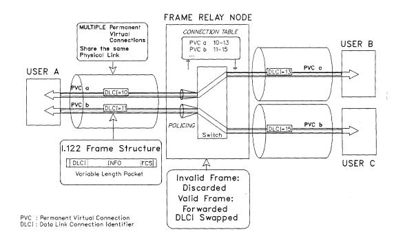
Figure 54. Frame Relay Principle
