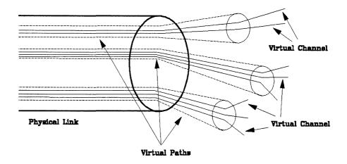
Figure 48. Link, Virtual Path and Virtual Circuit Relationship
