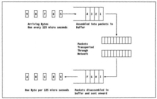
Figure 27. Transporting Voice over a Packet Network
