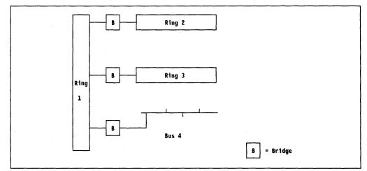
Figure 107. An Example of a Multisegment LAN
