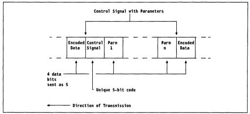
As noted above (for the SAT) and illustrated in Figure 99, control messages preempt data transmission with no loss in efficiency.
