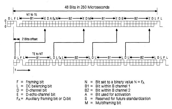
Figure 37. ISDN Basic Rate S/T Interface Frame Structure. The frame format used in the TE to NT direction is different from the one used in the NT to TE direction.
