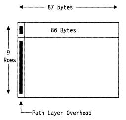
Figure 41. Sonet Synchronous Payload Envelope
