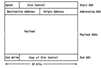
Figure 104. CRMA-II Slot Format
