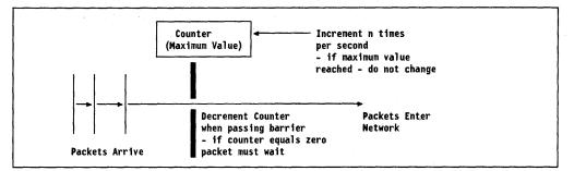
Figure 64. Leaky Bucket Rate Control
