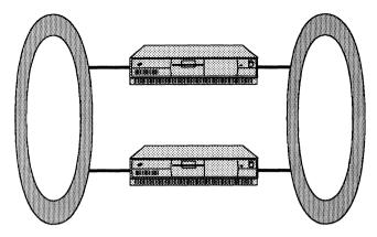
Figure 6.9 A simple parallel bridge configuration.
