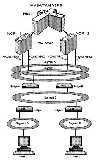
Figure 12.8 A dual ring and duplicate TIC addressing configuration.
