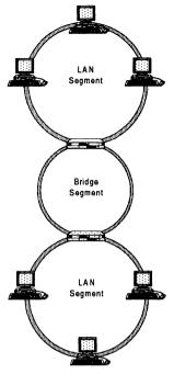
Figure 3.8 A multisegment LAN configuration.
