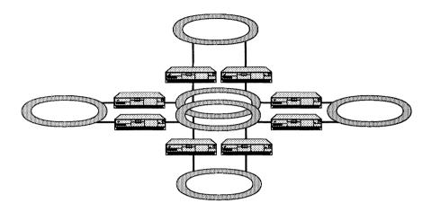
Figure 6.12 A dual ring backbone configuration.
