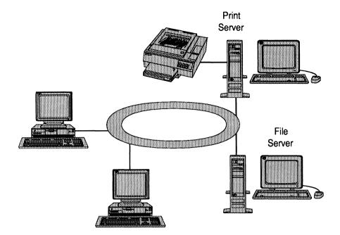
Figure 5.1 An illustration of a LAN server configuration.
