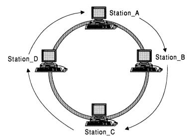
Figure 3.1 A sample Token-Ring Network and the flow of data around the ring.
