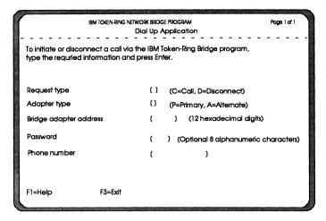
Figure 10.16 The Dial-Up Application parameter screen for remote dial support of the IBM Token-Ring Network Bridge Program.
