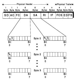
Figure 2.11 The destination and source address field formats of the MAC frame.
