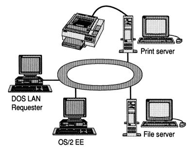
Figure 9.1 The IBM OS/2 LAN Server and Requester configuration.
