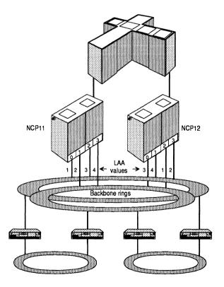
Figure 6.14 Duplicate TIC addressing using a dual ring backbone configuration.
