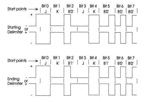
Figure C.1 Signal combinations used to determine the starting delimiter (SD) and ending delimiter (ED).
