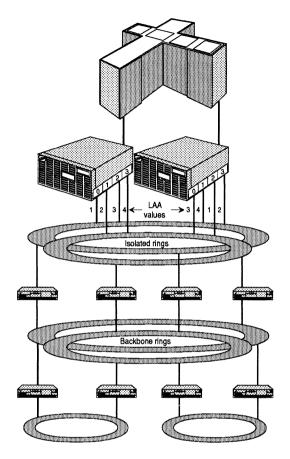
Figure 6.18 A high-availability configuration using the IBM 3172 Interconnect Controller.
