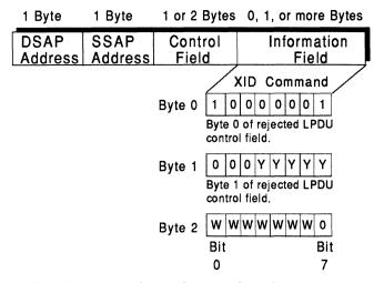
Figure 2.9 The format of the exchange identification command in an LPDU.
