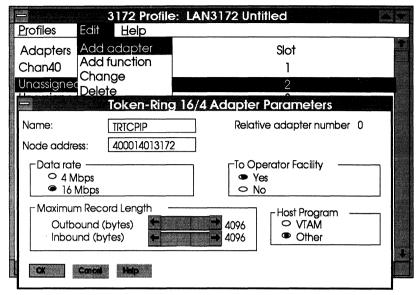
Figure 11.12 The OF/2 definiton screen for the IBM Token-Ring Adapter installed in the IBM 3172.
