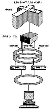
Figure 11.32 A dual-ring backup configuration using an IBM 3172.
