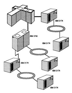
Figure 4.13 Some of the token-ring configurations that can be used with the IBM 3174.
