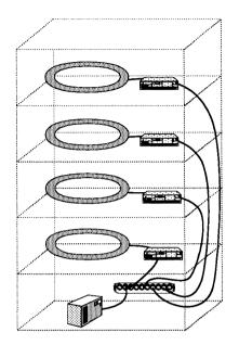
Figure 6.4 Centralized backbone configuration.
