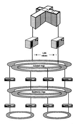
Figure 6.16 A high-availability configuration for the IBM 3174 Token-Ring Gateway Establishment Controller.
