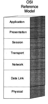
Figure 2.2 The seven layers of the OSI Reference Model.
