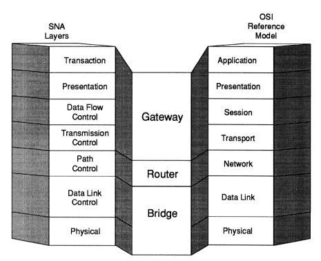
Figure 3.7 The relationship of bridge, router and gateway functions to the services provided by the OSI Reference Model and the SNA architecture.
