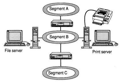
Figure 6.7 A serial LAN multisegment configuration.
