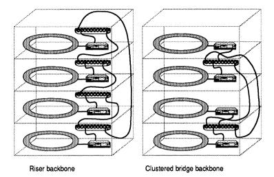
Figure 6.5 Distributed backbone configuration.
