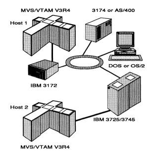
Figure 11.28 The SNA node type 4 connectivity to an SNA mainframe through an IBM 3172.
