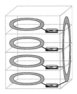
Figure 6.2 A single ring backbone configuration.
