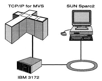
Figure 11.23 A sample token-ring environment for TCP/IP connectivity to the mainframe using the IBM 3172.
