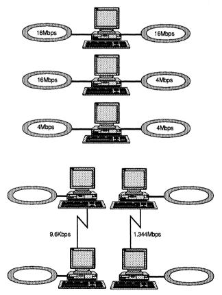
Figure 4.10 The IBM Token-Ring Network Bridge configurations.
