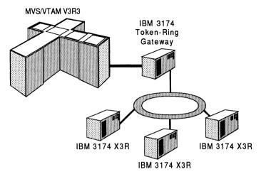
Figure 12.10 The local IBM 3174 Token-ring gateway configuration.
