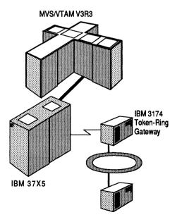
Figure 12.12 The remote IBM 3174 Token-Ring Gateway configuration.
