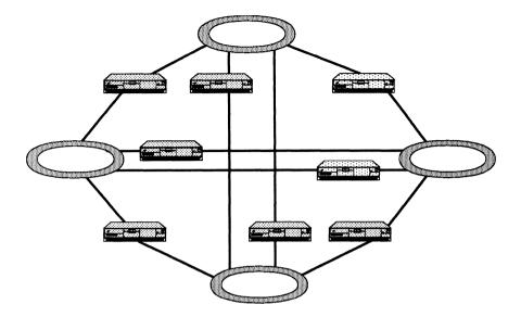
Figure 6.10 A token-ring mesh configuration.
