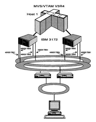
Figure 11.33 A dual-ring dual-3172 configuration.
