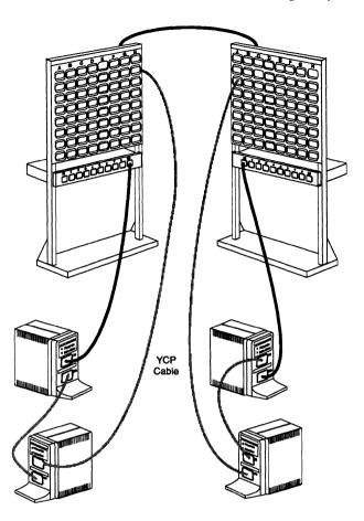
Figure 4.4 Illustrating the use of an IBM 8218.
