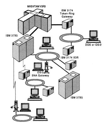
**Figure 12.1** A token-ring configuration featuring the three SNA tokenring gateways: the IBM 3174, IBM 3745 and IBM OS/2 SNA Gateway.
