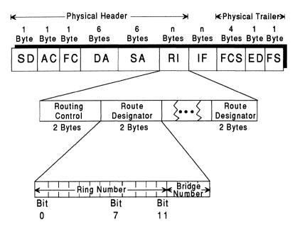
**Figure 2.14** The route designator field of the routing information field of the MAC frame.
