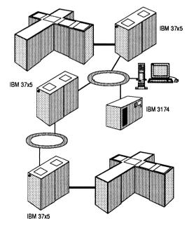
**Figure 4.14** Some of the connectivity options available when using token-ring connections on communications controllers.
