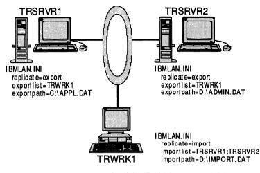
**Figure 9.11** The definitons in the OS/2 LAN Server and OS/2 workstation to support the replicate feature.
