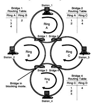
Figure 3.12 Transparent bridging and the use of the filtering database.
