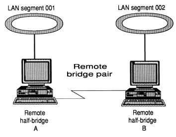
Figure 10.7 Diagram depicting the remote bridge configuration.
