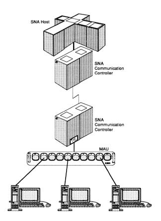
**Figure 1.4** The local area network connectivity to an SNA network using a token-ring architecture to create a Wide Area Network (WAN). The token-ring is comprised of the workstations and their connectivity to the MAU and the SNA communications controller and its connection to the MAU.
