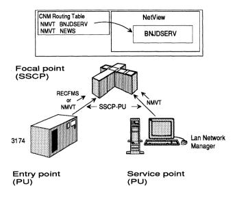
Figure 7.2 A typical ONM flow using SNA network management services.
