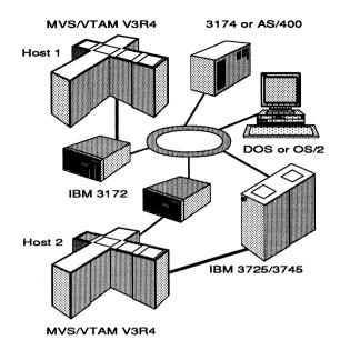
Figure 11.30 The SNA node type 5 configuration with two IBM 3172s devices.
