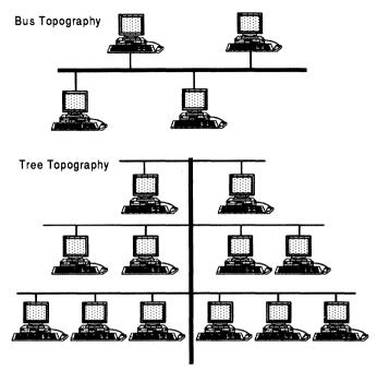
Figure 3.4 An example of a bus and a tree network.
