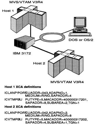
Figure 11.31 A shared token-ring adapter configuration and definitions.
