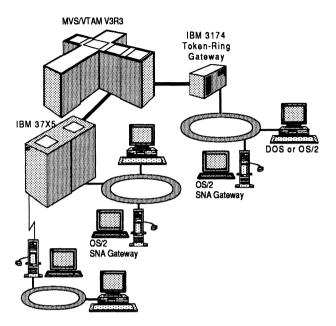
Figure 12.14 The IBM OS/2 SNA Gateway configuration.
