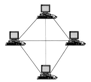
Figure 3.2 An example of a mesh network.
