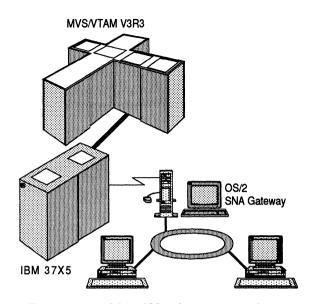
Figure 12.15 The remote OS/2 SNA Gateway configuration using an IBM 3745 Token-Ring Gateway.
