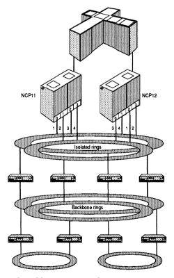
Figure 6.15 An isolated host-ring configuration.
