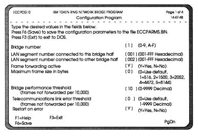
Figure 10.8 Screen 1 of the IBM Token-Ring Bridge Program remote bridge configuration.
