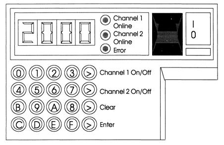
Figure 11.19 The operator display area for the IBM 3172.
