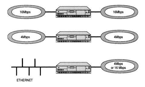
Figure 4.11 Three possible configurations for an IBM 8209.
