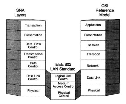
Figure 2.3 The IEEE 802 LAN Standard and the relationship to SNA and OSI.
