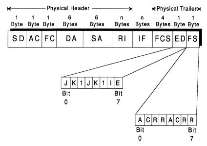
**Figure 2.15** The end delimiter and the frame status field formats of the MAC frame.
