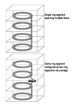
Figure 6.1 A simple multiple floor token-ring configuration.
