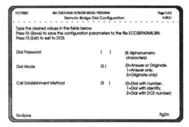
Figure 10.15 Remote dial configuration screen.
