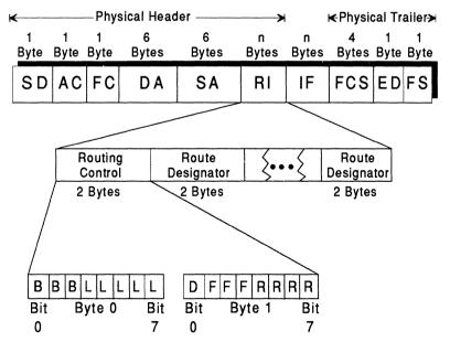
**Figure 2.12** The routing information field and the routing control sub-field.
