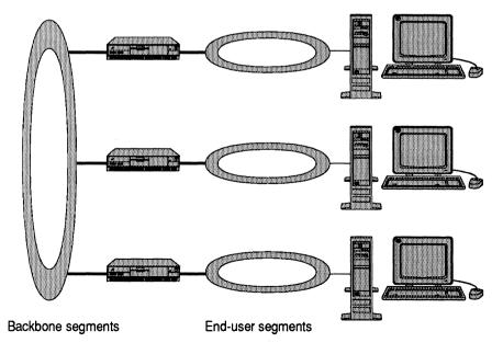
Figure 5.2 A sample end-user and backbone ring configuration.
