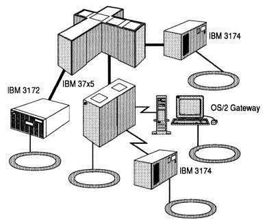
Figure 5.3 Token ring to mainframe connectivity.
