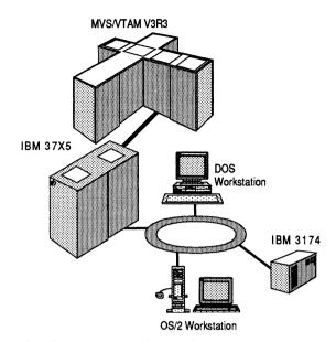
Figure 12.5 The downstream physical unit configuration to an IBM 3745 Token-ring LAN gateway.
