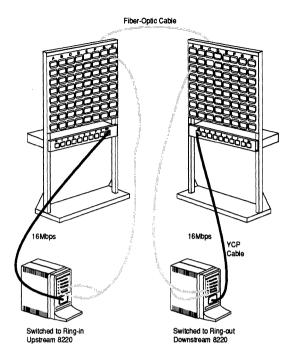
Figure 4.7 Two IBM 8220s are connected together to form the 8220 Fiber Optical Converter Subsystem.
