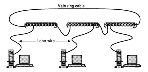
Figure 4.3 A small token-ring network using interconnected multistation access units.
