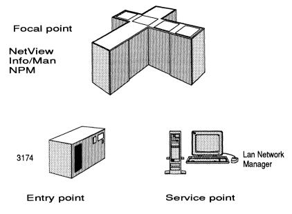
Figure 7.1 The three-tiered structure of ONM.
