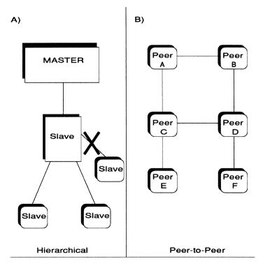
Figure 1.1 In diagram A, a master-slave relationship is depicted. New resources cannot enter the network until the master defines their address. In diagram B, a peer network is depicted. As new peers connect to the network, information about the connecting peers is exchanged. Peer D notifies Peer F of connecting routes to peers A, B, C and E and the network resources found on each. Likewise, if Peer F had peers attached to it, it would notify Peer D in the same fashion.
