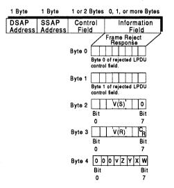
Figure 2.8 The frame reject information field format in an LPDU.
