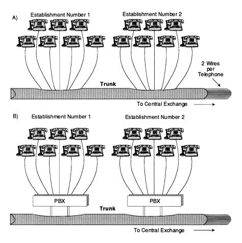
**Figure 1.3** Diagram A illustrates telephone connectivity before the use of PBXs. Diagram B illustrates the use of PBXs.
