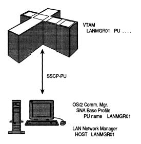
Figure 8.2 The network management flow requirements between VTAM and LAN Network Manager.
