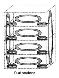
Figure 6.6 A dual ring backbone configuration.
