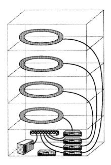
Figure 6.3 A collapsed backbone ring configuration.
