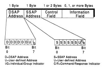
Figure 2.5 The format of the LPDU and a break out of the destination and Source Access Point fields.
