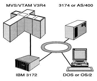
Figure 11.26 An SNA node type 2.0 and 2.1 token-ring connectivity configuration to the SNA mainframe using an IBM 3172.
