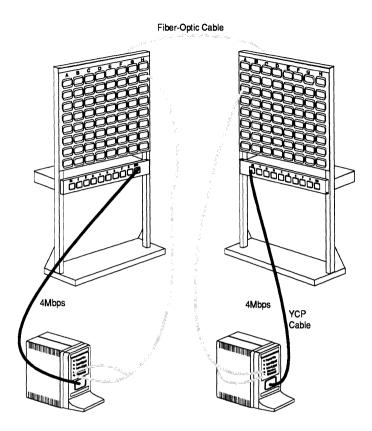
Figure 4.6 IBM 8219 repeaters connect two wiring closets.
