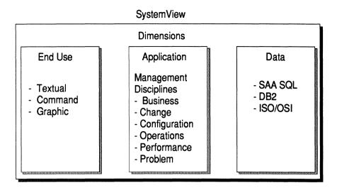
Figure 7.6 IBM's SystemView architecture, dimensions and disciplines.
