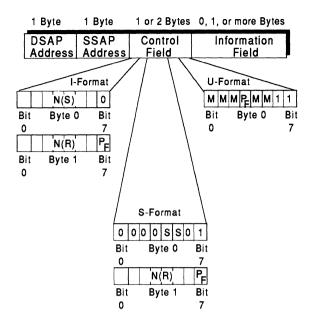
Figure 2.6 The three formats of the LPDU control field.
