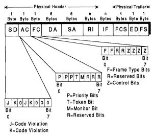
Figure 2.10 The medium access control frame format.
