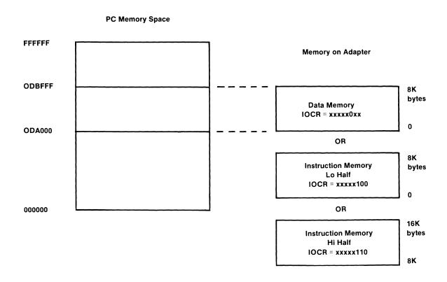
The same jumpers used to select the I/O address also select the base memory address that is used to map the adapter's memory to the PC memory bus. These values are:
