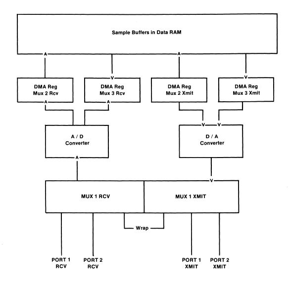
The basic sampling rate of the A/D and D/A converter can be set by SP code to either 8000Hz or 9600Hz (the SP control program always sets this to 9600Hz). Within each cycle, four digital samples are processed: two through the D/A converter and two through the A/D converter. The four samples being multiplexed by Multiplexer (Mux) 1 are from the two ports represented by Mux 2 and Mux 3. Where the samples are located in data memory is controlled by four Dynamic Memory Addressing
