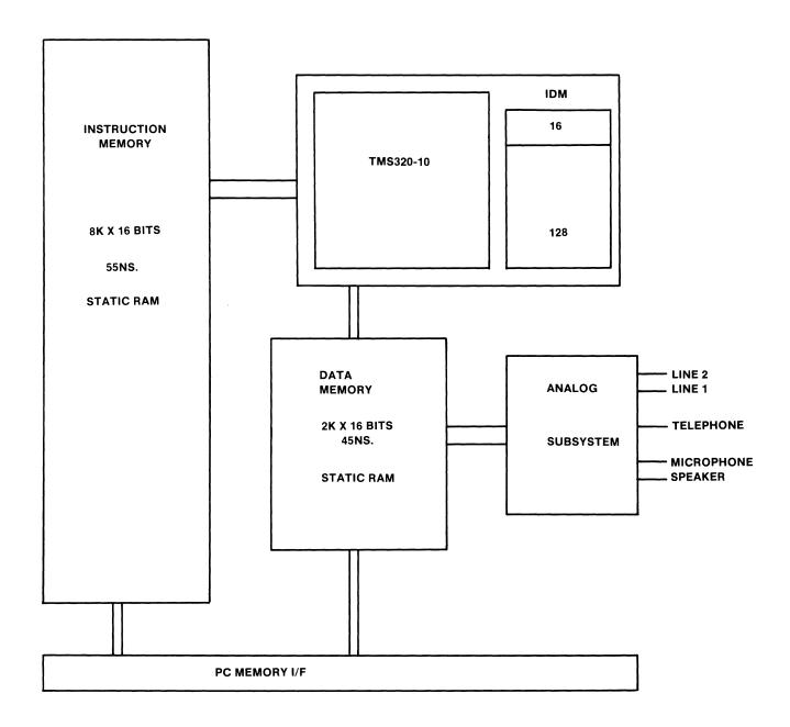
Internal Data Memory (IDM) on the TMS320 chip consists of 144 words; 16 of which are reserved for the control program and 128 for use by the partitions.
