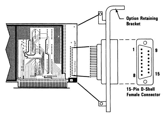
The following example shows how a 15-pin, D-shell, female connector is attached to a prototype card.
