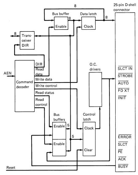
The following is a block diagram of the printer adapter portion of the Monochrome Display and Printer Adapter.
