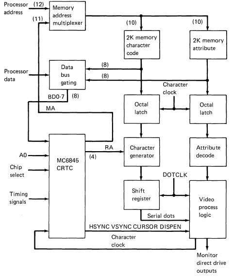
The following is a block diagram of the monochrome display adapter portion of the IBM Monochrome Display and Printer Adapter.
