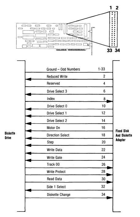
**Note:** Connection is through a 2-by-17 Berg connector. Pin 5 is reserved to polarize the connector.
