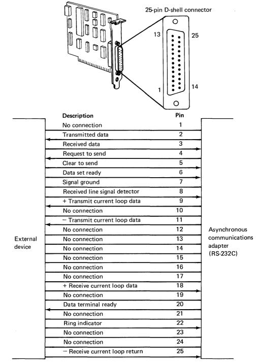
The following page shows the connecter pin assignments and specifications for the Asynchronous Communications Adapter.
