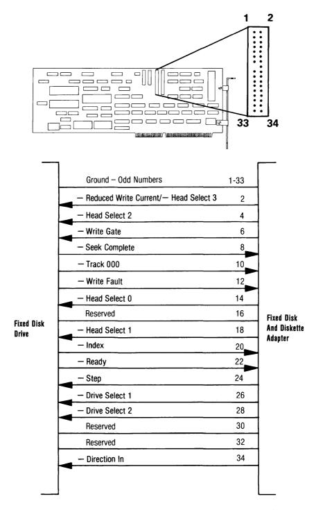
**Note:** Connection is through a 2-by-17 Berg connector. Pin 15 is reserved to polarize the connector.
