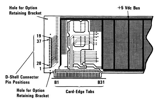
The pin side has a + 5-Vdc bus, 1.27 millimeters (0.05 inch) wide, screened onto it, and card-edge tabs that are labeled B1 through B31.
