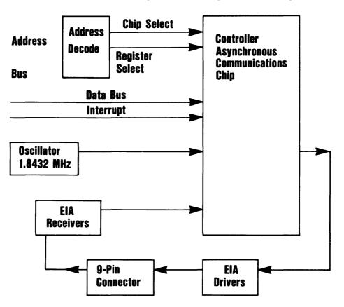
The following figure is a block diagram of the serial portion of the adapter.
