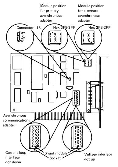
If the adapter is to be installed in expansion slot 8, a jumper is required on connector J13.
