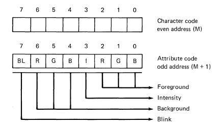
The adapter decodes the character attribute byte as defined above. The blink and intensity bits may be combined with the foreground and background bits to further enhance the character attribute functions listed below:
