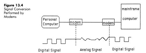
of analog line connections. Although an analog transmission medium for a transmission path between modems can be a direct connect, leased, or switched line, modems are directly connected (hard wired) to direct connect and leased lines, whereas they are interfaced to a switched facility. Thus, a terminal user can only communicate with the one distant location on a leased line, but he or she can communicate with many devices when he or she has access to a switched line.
