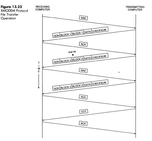
error. Then the receiving station will transmit an NAK character that serves as a request to the transmitting station to retransmit the previously transmitted block.
