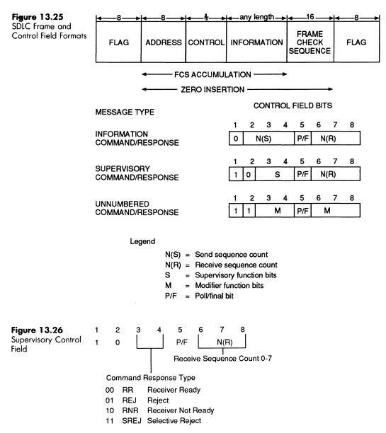
Using an 8-bit control field, the N(S)/N(R) count ranges from 0 to 7. Using a 16bit control field the count can range from 0 to 127. The P/F bit is a poll/final bit. It is used as a poll by the primary (set to 1) to obtain a response from a secondary station. It is set to 1 as a final bit by a secondary station to indicate the last frame of a sequence of frames.
