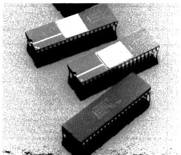
**Figure 1.5** Three Intel Math Coprocessors (Photograph courtesy of Intel Corporation)
