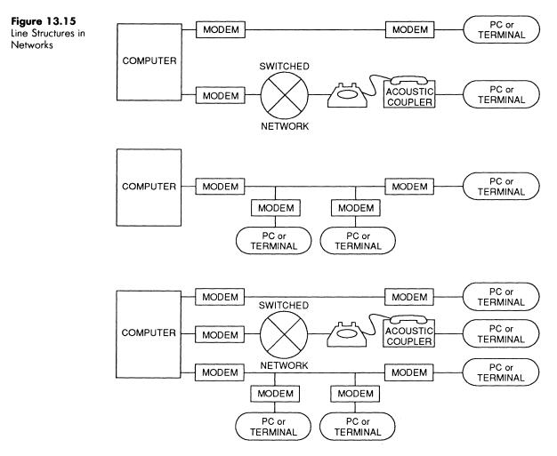
the message recipients. In some systems a "broadcast" address permits all devices connected to the same multidrop line to receive a message at the same time. When you use multidrop lines, overall line costs may be reduced, because common portions of the line are shared for use by all devices connected to that line. To prevent data transmitted from one device from interfering with data transmitted from another device, a *line discipline* or control must be established for such a link.
