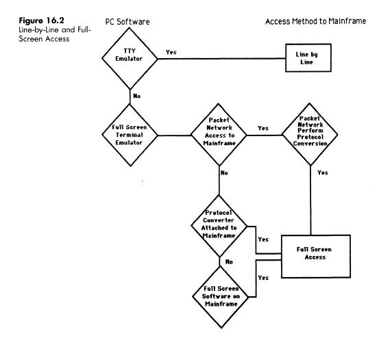
converter attached to the organization's mainframe or a software program on the mainframe to operate in conjunction with the software operating on the personal computer.
