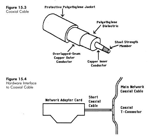
lectric employed; and the type of protective jacket and material used to provide strength to the cable, which allows it to be pulled through conduits without breaking.
