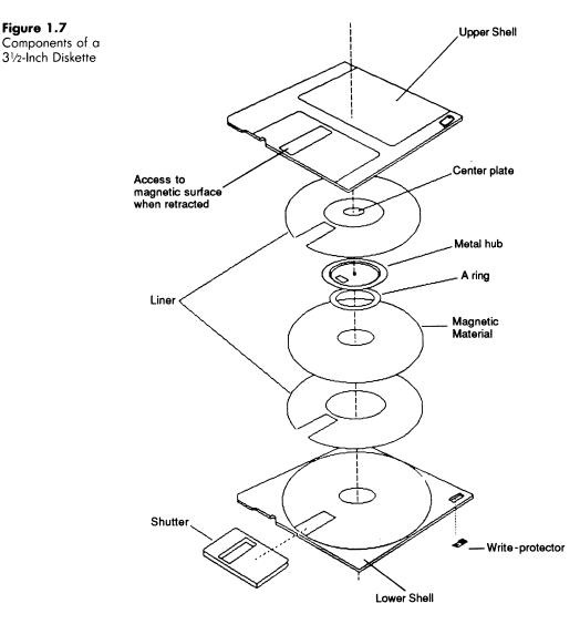
diskette to store 720K bytes of data, or you can use high-capacity diskettes to double the data-storage capacity. If you use  $3\frac{1}{2}$ -inch high-capacity diskettes, you can format the diskette to store 18 sectors per track. The storage capacity of this diskette then becomes 2 sides times 80 tracks per side times 18 sectors per side times 512 bytes per sector, yielding 1,474,560 bytes (1.44M bytes) of information.
