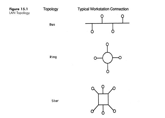
be viewed as functioning similar to a telephone switchboard, because access from one station to another station on the net can only occur through the central device.
