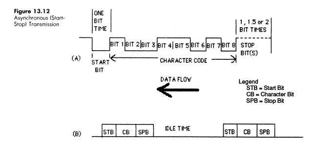
character, and synchronization is maintained on a character-by-character basis. Asynchronous transmission normally is used for transmission at speeds up to 9600 bps over the switched telephone network, whereas data rates up to 19,200 bps are possible over a direct connect cable whose distance is limited to 50 feet. Such transmissions can also occur on conditioned leased lines.
