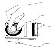
7. Replace the cover on the mouse with the **open** arrow aligned with the slot in the roller ball cavity.
