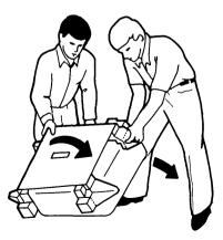
6. Tilt the unit to the other side, putting the other packing pad in place.
