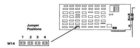
**Position 1** Interrupts every 9.1 ms **Position 2** Interrupts every 18.3 ms **Position 3** Interrupts every 36.6 ms **Position 4** Interrupts every 73.2 ms
