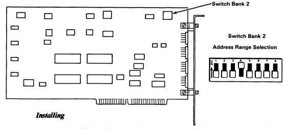
You may install this adapter in slots 2, 4, 5, 7, or 8 in the IBM 6150 and in slots 2 through 5 in the IBM 6151. See the system unit diagram to locate the adapter slots.
