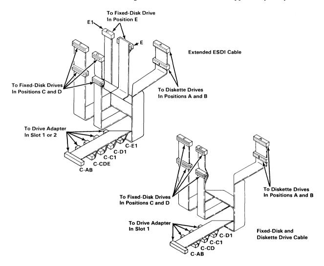
C-AB and C-CD or C-CDE are connected to the 34-pin connectors on the drive adapter, and C-C1 is connected to the 20-pin connector.
