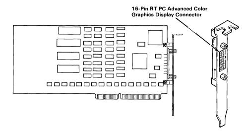
Installing: You can install this adapter in adapter slot 2, 4, 5, 7, or 8 in IBM 6150 and in slot 2, 3, 4, or 5 in IBM 6151, whichever is available. See the system unit diagram for the correct adapter slot.
