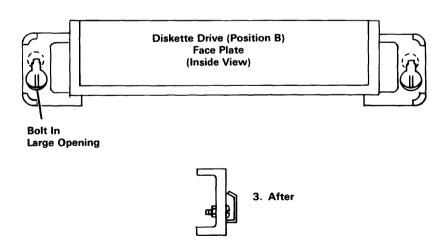
c. Pull the faceplate off the two bolts holding it in place.
