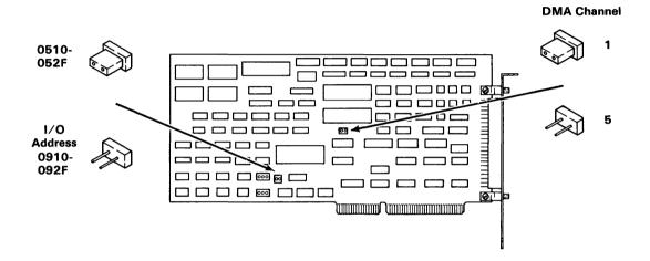
Installing: You can install this adapter in slots 2, 4, 5, 7, or 8 in IBM 6150 and in slots 2, 3, 4, or 5 in IBM 6151, whichever is available. See the system unit diagram for the correct adapter slot.
