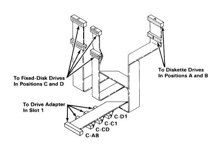
11. Connect C-C1 on the cable bundle to the 20-pin connector on the drive adapter.
