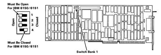
The illustration above shows the normal Switch Bank 1 configuration. Use the following table to set Switch Bank 1 if your configuration requirements differ.
