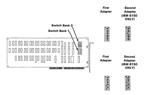
Warning: Do not install this adapter in slot 8 in IBM 6150 or in slot 5 in IBM 6151.
