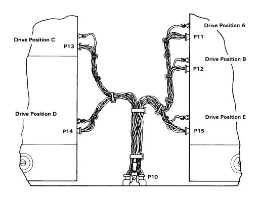
9. Connect P14 on the power cable to the 4-pin connector on the rear of the fixed-disk drive in position D. Connect the ground wire from the power cable to the ground tab on the drive.
