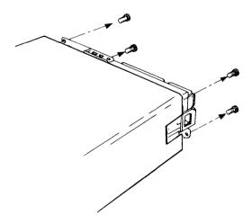
8. Face the front of the unit and pull forward on the cover, sliding it off the system unit.
