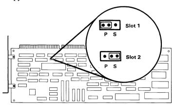
14. Put whichever drive adapter your system uses back in the appropriate slot as shown below, and replace the screw.
