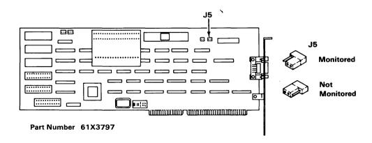
**Installing:** You may install this adapter in slots 2, 4, 5, 7, and 8 in Model 25 and in slots 2 through 5 in Model 10, whichever is available. See the system unit diagram for slot locations.
