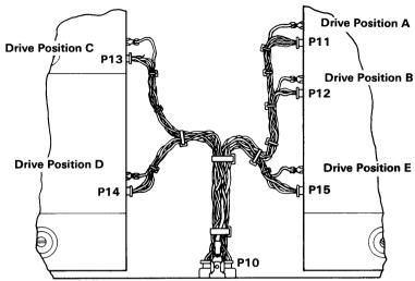
5. Connect P15 on the power cable to the 4-pin connector on the rear of the fixed-disk drive. Connect the ground wire to the ground tab on the drive.
