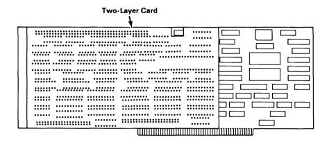
Warning: This option replaces the IBM RT PC Floating-Point Accelerator, if installed, and must be located in slot B of the system board.
