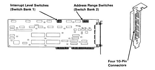
With the IBM RT PC 4-Port Asynchronous RS422A Adapter and the correct cables, you can connect a system unit to ASCII terminals located up to 1212 meters (3963 feet) from the system unit.
