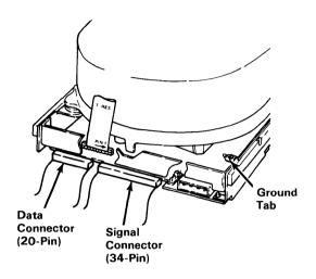
7. Facing the rear of the unit, release the plastic latches holding the drive in place and carefully remove the drive from position C.
