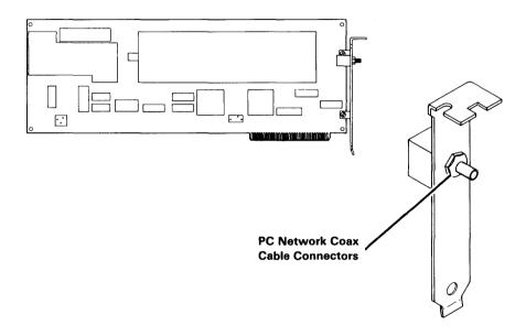
The jumpers on this adapter can be set to either interrupt level 3 or 9. If vou have the IBM PC Enhanced Graphics Adapter or the IBM Personal Computer 3278/79 Emulation Adapter, ensure that the interrupt level on the IBM PC Network Adapter is set to 3, since these other two adapters use 9. To set the interrupt level to 3, set jumper W4 as shown. To set the interrupt level to 9, set the same jumper (called W3 when set at 9) as shown in the illustration below.
