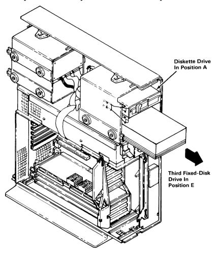
8. If drive is to be reinstalled in drive position C, see "Installing a Fixed-Disk Drive in Position C" for installation of the drive and replacement of the cooling fan.
