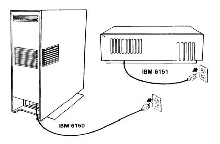
3. If connected, unplug the display power cable and system unit power cable from the system unit.
