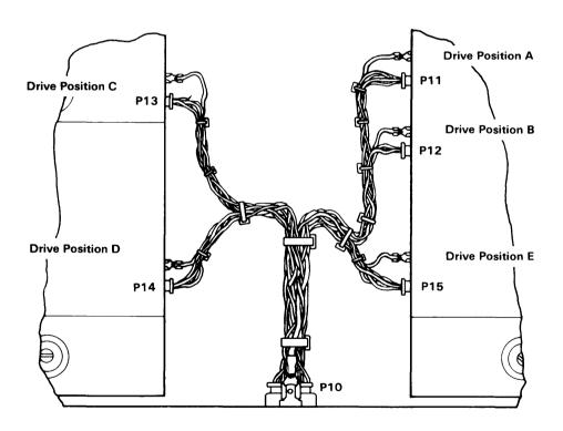
9. Connect P13 on the power cable to the 4-pin connector on the rear of the fixed-disk drive in position C. Connect the ground wire from the power cable to the ground tab on the drive.
