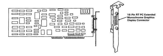
**Installing:** You can install this adapter in adapter slot 2, 4, 5, or 7 in IBM 6150 and in slot 2, 3, or 4, in IBM 6151, whichever is available. See the system unit diagram for the correct adapter slot.
