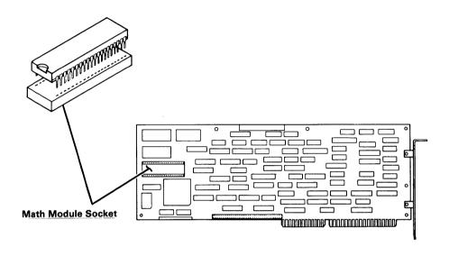
**Warning:** You must install the IBM RT PC Personal Computer AT Coprocessor Option in adapter slot 8 in IBM 6150 and in adapter slot 5 in IBM 6151.
