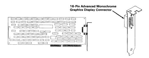
**Installing:** You can install this adapter in adapter slot 2, 4, 5, 7, or 8 in IBM 6150 and in slot 2, 3, 4, or 5 in IBM 6151, whichever is available. See the system unit diagram for the correct adapter slot.
