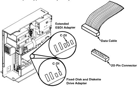
13. If your system uses the IBM RT PC Extended ESDI Magnetic Media Adapter, set Jumper J6 according to which slot the adapter will occupy.
