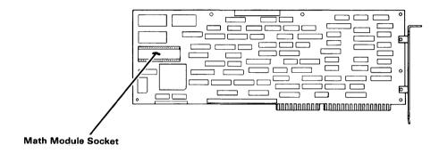
To install the IBM Personal Computer AT Math Co-Processor, align the pins on the module with the connector on the IBM RT PC Personal Computer AT Coprocessor Option. Align the notch on the module with the notch on the connector. Press the module into place.
