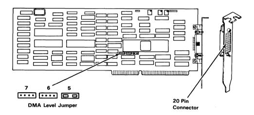
**Installing:** You may install this adapter in slots 2, 4, 5, 7, or 8 in an IBM 6150. See the system unit diagram to locate the adapter slots.
