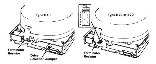
3. Check the drive selection jumper or switches for the correct setting and make sure the terminating resistor is present on the drive.
