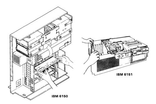
8. Align the screw holes and ensure that the adapter bracket is even with the frame.
