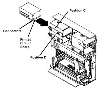
5. Facing the rear of the unit, place the drive on the side rails and slide it into drive position C. Push the drive in until the plastic latches snap into position, holding the drive in place.
