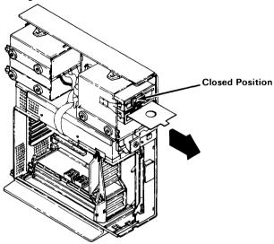
11. Replace the cooling fan assembly. See "Cooling Fan Replacement" on page 2-7.
