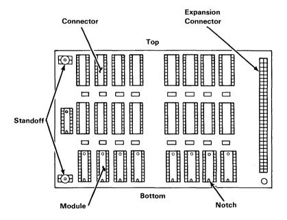
2. Install each module with the notch facing the bottom edge of the card, as shown in the following drawing:
