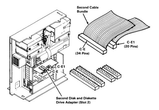
If you are installing an E70 fixed-disk drive, connect C-E1 (C-CDE is already connected) to the IBM RT PC Extended ESDI Magnetic Media Adapter as shown.
