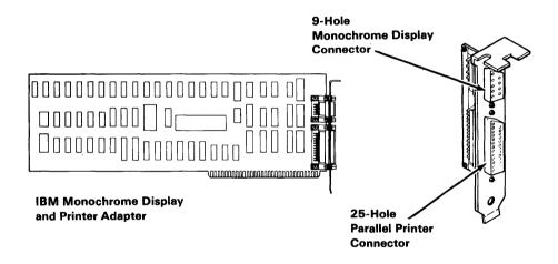
Warning: You must install this adapter in adapter slot 3 in IBM 6150 and in slot 1 in IBM 6151.
