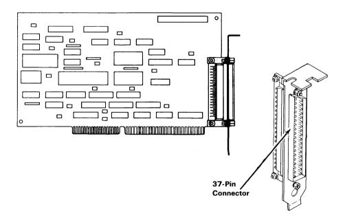
Installing: You can install this adapter in slot 2, 4, 5, 7, or 8 in IBM 6150 and in slots 2 through 5 in IBM 6151, whichever is available. See the system unit diagram for the correct adapter slot.
