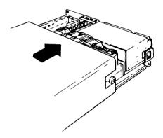
2. Fit the rear cover plate in place. Tighten the screws.
