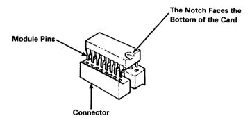
3. Align the pins of each module with the connector on the card and press each of the 16 modules in place.
