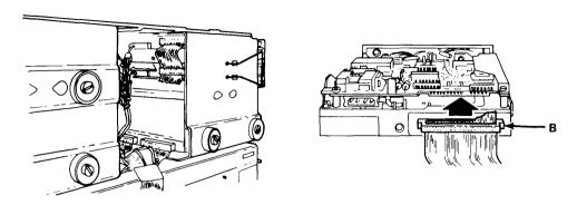
9. Connect P12 on the power connector to the 4-pin connector on the rear of the diskette drive. (See page 2-25 for a diagram of the power cable and connectors.) Connect the ground wire to the ground tab on the second diskette drive.
