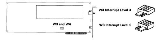
Installing: You can install this adapter in slots 2 through 8 in IBM 6150 and in slots 1 through 5 in IBM 6151, whichever is available. See the system unit diagram for the correct adapter slot.
