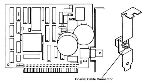
**Note:** The connector extends beyond the bracket. Rotate or tilt the adapter to install it.
