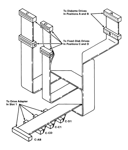
7. Connect C on the cable to the 34-pin connector on the rear of the drive in position C. Connect C1 to the 20-pin connector on the drive.
