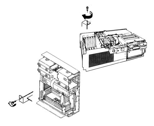
Adapters in system board slots B, C, and D have no screws or brackets. Slide these adapters into the slots as in Steps 6 and 7.
