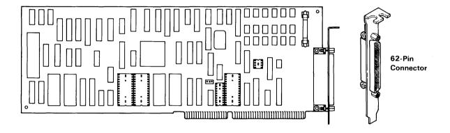
**Installing:** You may install this adapter in slots 2 through 8 in the IBM 6150 and in slots 2 through 5 in the IBM 6151. See the system unit diagram in Appendix A to locate the adapter slots.
