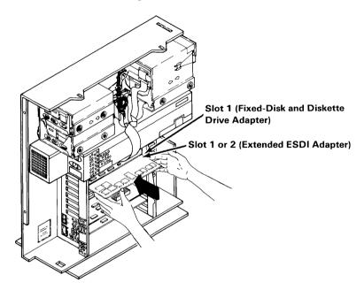
15. If this is the last drive to be installed, replace the cooling fan assembly. See "Cooling Fan Replacement" on page 2-7.
