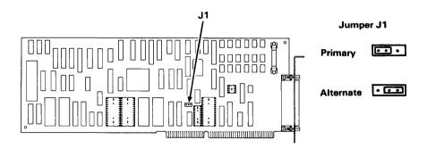
The following table shows the address ranges provided by jumper J1. If two IBM RT PC SCSI Adapters are used, one must be configured in the Primary J1 position and the other in the Alternate J1 position. A single adapter may be configured for either address range.
