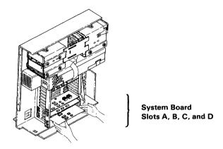
In IBM 6151, the plastic option retainers hold the adapters in place. Open the retainers, slide the adapters into the slots as in Steps 6 and 7, and close the retainers.
