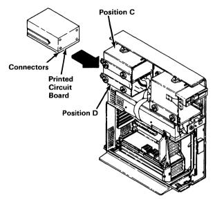
5. Facing the rear of the unit, place the drive on the side rails and slide it into drive position D. Push the drive in until the plastic latches snap into position, holding the drive in place.
