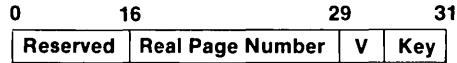
Figure 11-33. TLB Real Page Number, Valid, and Key Bits (One of Sixteen Per TLB)
