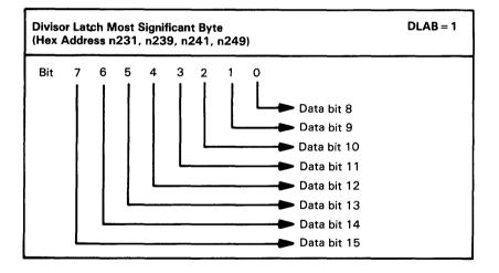
Figure 15. Divisor Latch Most Significant Byte
