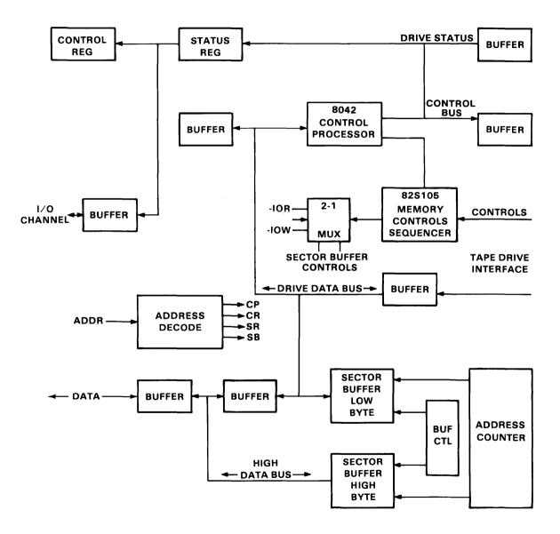
Figure 1. Streaming Tape Adapter Block Diagram
