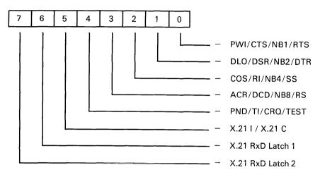
The Port 2 modem input register is identical to the port 1 register except it includes the RS366 and X.21 control signals.
