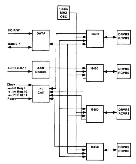
Figure 1. 4 Port Asynchronous RS232C Adapter Block Diagram
