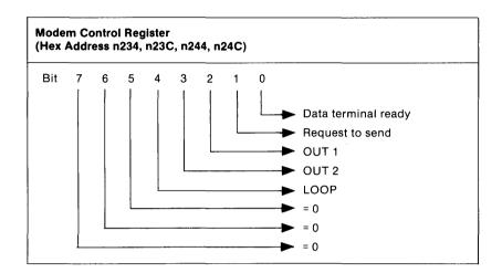
This 8-bit register controls the interface with the modem or data set (or other peripheral device). The contents of the modem control register are described below:
