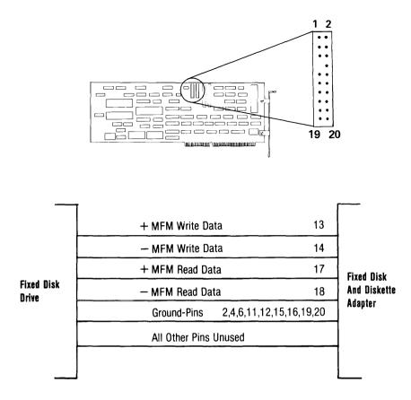
**Note:** Connection is through a 2-by-10 Berg connector. Pin 8 is reserved to polarize the connector.
