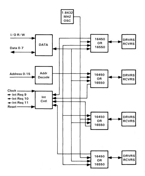
Figure 1. 4-Port Asynchronous RS-422A Adapter Block Diagram
