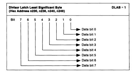
Figure 14. Divisor Latch Least Significant Byte
