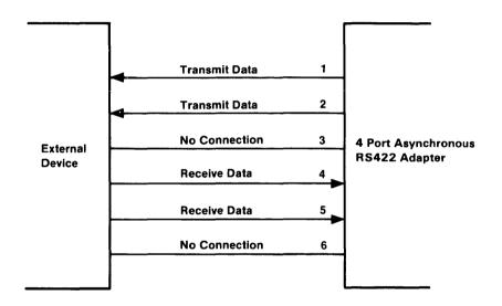
Figure 17. Connector Specifications
