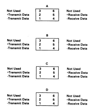
Figure 9. 6 Pin Interface Signals Connector (as viewed from rear of adapter)
