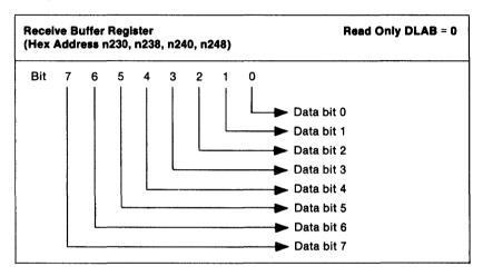
Bit 0 is the least significant bit and is the first bit serially received.
