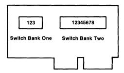
Figure 2. 4-Port Asynchronous RS-422A Adapter Switches
