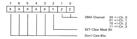
Each DMA channel has a mask bit which disables the incoming DMA request signal on that channel. Each channel's mask bit is automatically set when that channel's terminal count is reached if that channel is not in autoload mode. After reinitialization of the appropriate channel address and count registers to prepare for the next DMA transfer, the mask register is cleared to reenable that channel's DMA request.
