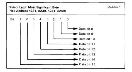
Figure 15. Divisor Latch Most Significant Byte
