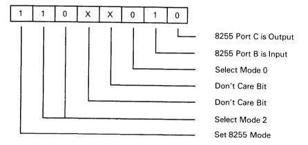
Execution of an I/O write with data H'C2' to address H'0523' or H'0923' (depending on adapter address jumpers) is necessary to initialize the I/O interface to the 8051 adapter controller. This is accomplished by setting up the operating modes for the 8255 peripheral interface module.
