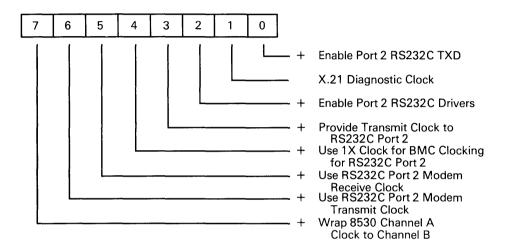
Execution of an I/O write to address H'052F' (or H'092F', as appropriate) allows the system device driver code to manipulate various enables and clock sourcing controls associated with the adapter Port 2.
