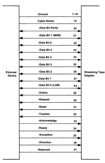
Figure 2. IBM RT PC Streaming Tape Drive Adapter Interface Specifications
