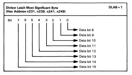
Figure 15. Divisor Latch Most Significant Byte
