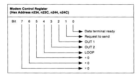
**Bit 0** This bit controls the data terminal ready (-DTR) output. When bit 0 is set to a logical 1, the -DTR output is forced to a logical 0. When bit 0 is reset to a logical 0, the -DTR output is forced to a logical 1.
