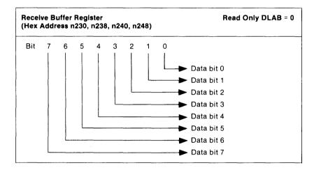
Bit 0 is the least significant bit and is the first bit serially received.
