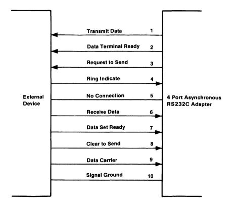
Figure 17. Connector Specifications
