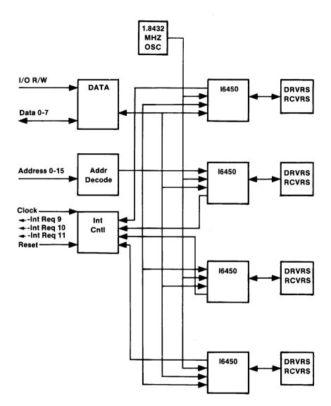
Figure 1. 4 Port Asynchronous RS422 Adapter Block Diagram
