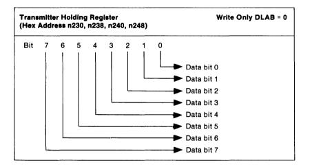
Bit 0 is the least significant bit and is the first bit serially transmitted.
