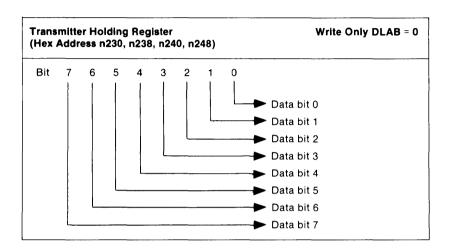
The transmitter holding register contains the character to be serially transmitted and is defined below:
