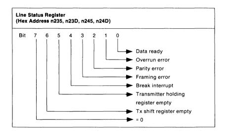
This 8-bit register provides status information to the processor concerning the data transfer. The contents of the line status register are described below:
