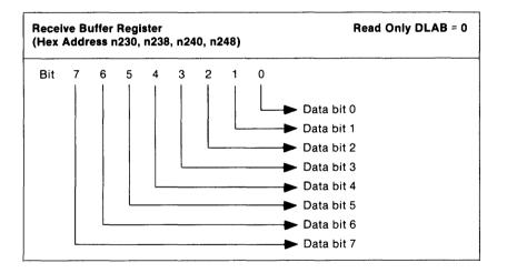
Bit 0 is the least significant bit and is the first bit serially received.
