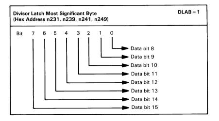
Figure 15. Divisor Latch Most Significant Byte
