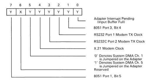
Execution of an I/O Read from address H'0521' or H'0921' (depending on adapter address jumpers) provides the adapter status register 1 to the system processor.
