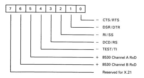
The Port 1 modem input register can only be read by the 8051. It contains the status of the control lines from the DCE to the DTE. These registers are updated on the leading edge of the 8051 read pulse and should be debounced by the user supplied microcode program.
