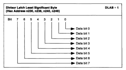
Figure 14. Divisor Latch Least Significant Byte
