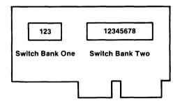
Figure 2. 4-Port Asynchronous RS-232C Adapter Switches
