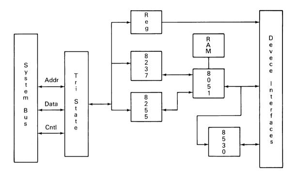
Figure 1. Multiprotocol Adapter Block Diagram
