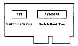
Figure 2. 4 Port Asynchronous RS422 Adapter Switches
