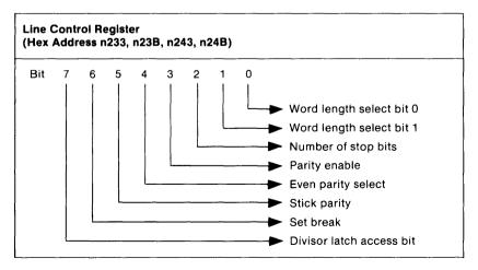
**Bits 0, 1** These two bits specify the number of bits in each transmitted or received serial character. The encoding of bits 0 and 1 is as follows:
