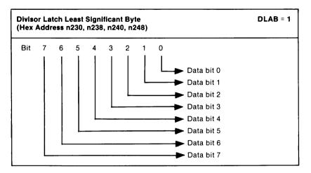
Figure 14. Divisor Latch Least Significant Byte
