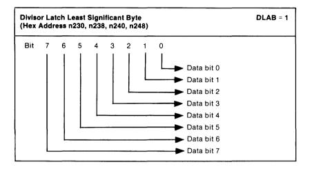
Figure 14. Divisor Latch Least Significant Byte
