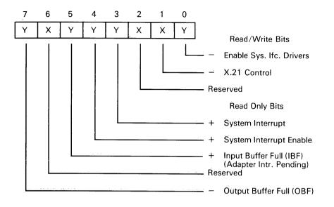
Execution of I/O to address H'0522' (or H'0922', as appropriate) allows the system device driver code to manipulate various adapter interface enables. Proper operation of this adapter control register is dependent on prior initialization of the 8255 mode register as described subsequently.
