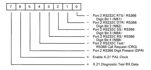
Output control signals for the adapter Port 2 can drive either an RS232C modem or an RS366 autocall device. Consequently, each Port 2 output has two possible definitions, only one of which is valid at any time.
