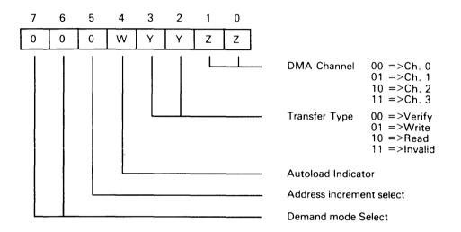
Each of the four available DMA channels has a 6-bit mode register associated with it. Initialization of these registers is required to define the characteristics of the DMA transfer that is to take place on that channel. The significance of the variable data bits in these initializations is as follows:
