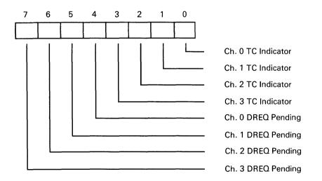
The status register is read by the system processor. It contains the status of the four DMA channels. The TC indicator bit indicates that the specified channel has progressed to terminal count
