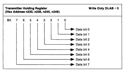
The transmitter holding register contains the character to be serially transmitted and is defined below:
