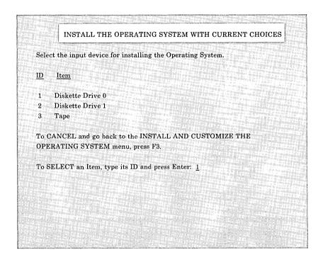
To work properly, diskette drive 1 (item 2) must be a 1.2M-byte drive.
