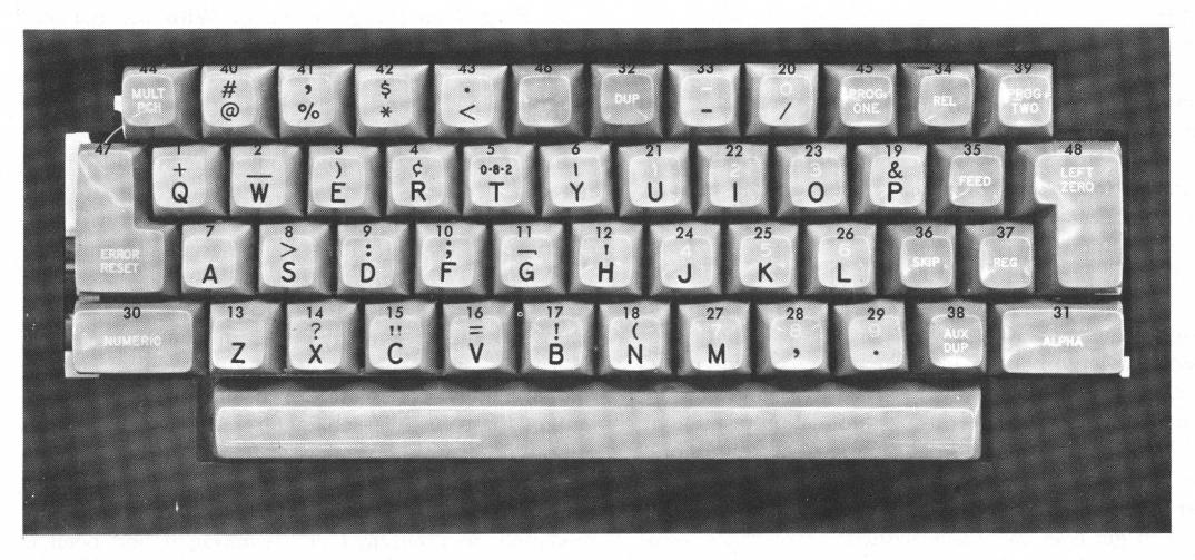
Figure 28. Keys—Combination Keyboard
