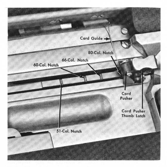
Figure 17. Latch-Type Card Pusher
