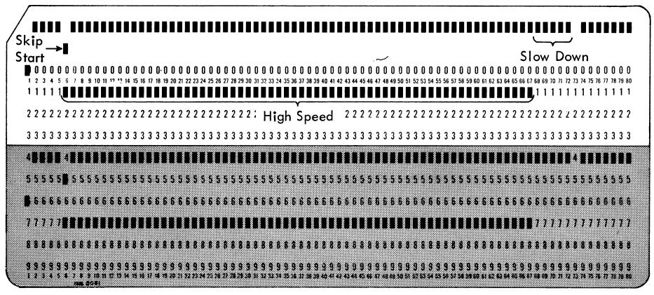
Figure 15. High-Speed Skip Program Card
