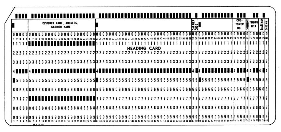
Figure 11. Alphabetic and Numeric Punching—Program One and Program Two
