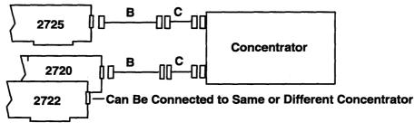
2725 FDDI-STP Single-Ring and 2726 FDDI-STP Dual-Ring Attach to a Concentrator
