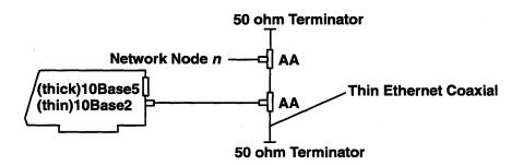
**Note:** *n* is a maximum of 30 nodes per segment (maximum of five segments with each segment connected by a repeater).
