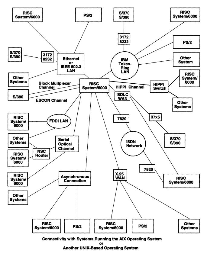
**Note:** The RISC System/6000 system, the PS/2, and the System/370 shown in this figure are running the AIX operating system.
