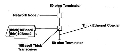
**Note:** *n* is a maximum of 100 nodes per segment (maximum of 5 segments with each segment connected by a repeater).
