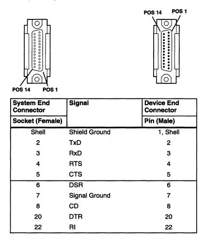
For applications where the Multiprotocol Adapter/A will be used, the following additional pins are required.
