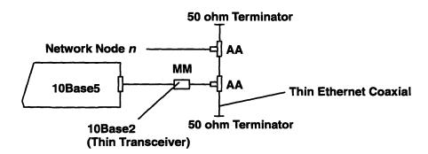
**Note:** *n* is a maximum of 30 nodes per segment (maximum of five segments connected by a repeater).
