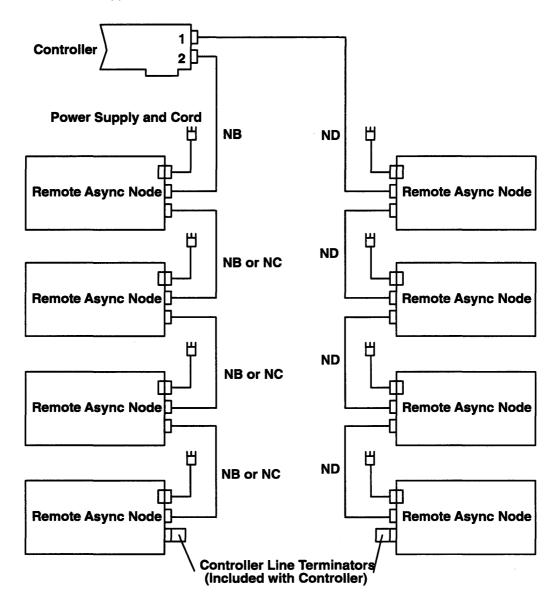
The 128-Port Async Controller supports up to four Remote Async Nodes on each controller line using the following attachment options:
