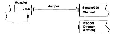
**Note:** The ESCON jumper cable can connect to any ESCON channel, trunk, or ESCON director.
