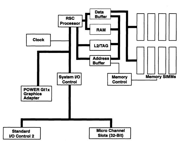
Block diagram showing a RISC single chip (RSC) processor module with supporting memory and I/O modules.
