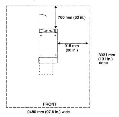
The amount of space needed by the unit during normal operation is indicated by broken lines on the footprint.
