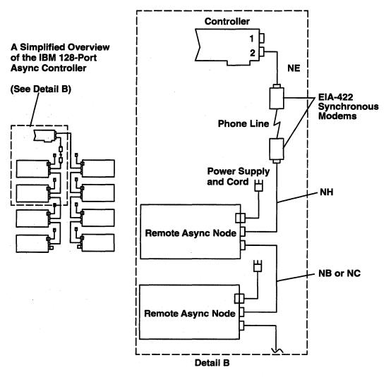
A choice of cables can be attached to any of the 16 Remote Async Node ports, as shown in the following illustration. These ports are labeled 0 through 15 and accept 4-, 6-, 8-, and 10-pin RJ-type connectors.
