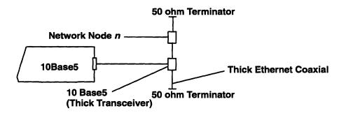
**Note:** *n* is a maximum of 100 nodes per segment (maximum of five segments with each segment connected by a repeater).
