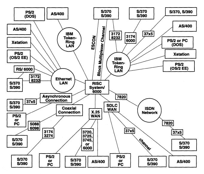
Connectivity with IBM Systems Running a Non-UNIX-Based Operating System
