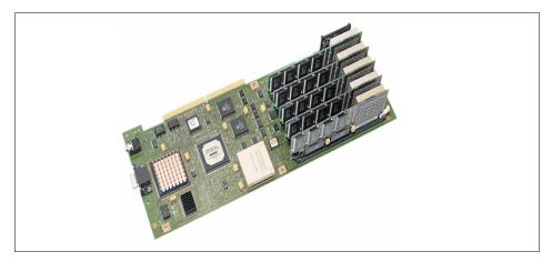
Figure 5. The IBM GXT800P Graphics Accelerator
