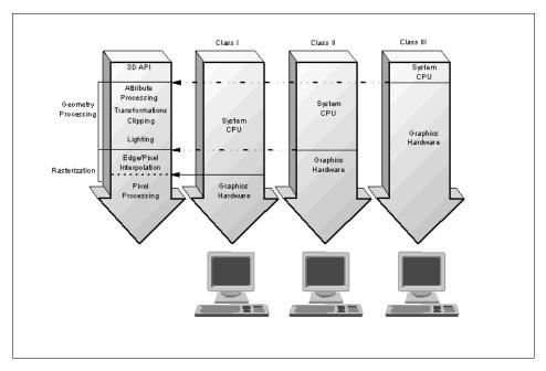
Figure 2. The Three Classes of Graphic Adapters
