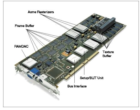
Figure 1. The IBM GXT3000P Graphics Accelerator (without Shields)
