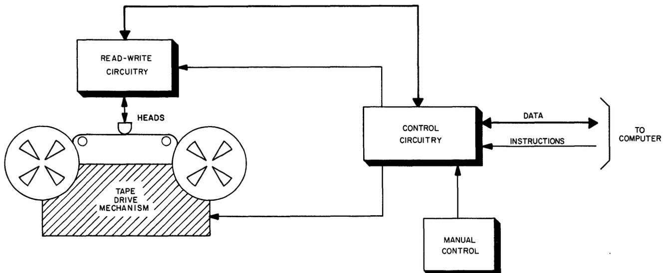
Figure 3-84. Basic Tape Storage Arrangement
