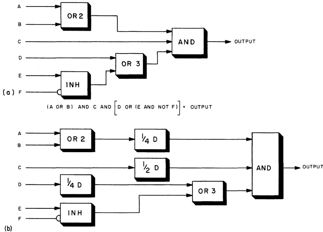
Figure 3-22. Sample Logic Circuit Combination
