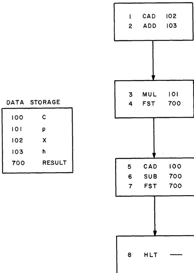
Figure 5-2. Flow Chart, Coded Straight-Line Program
