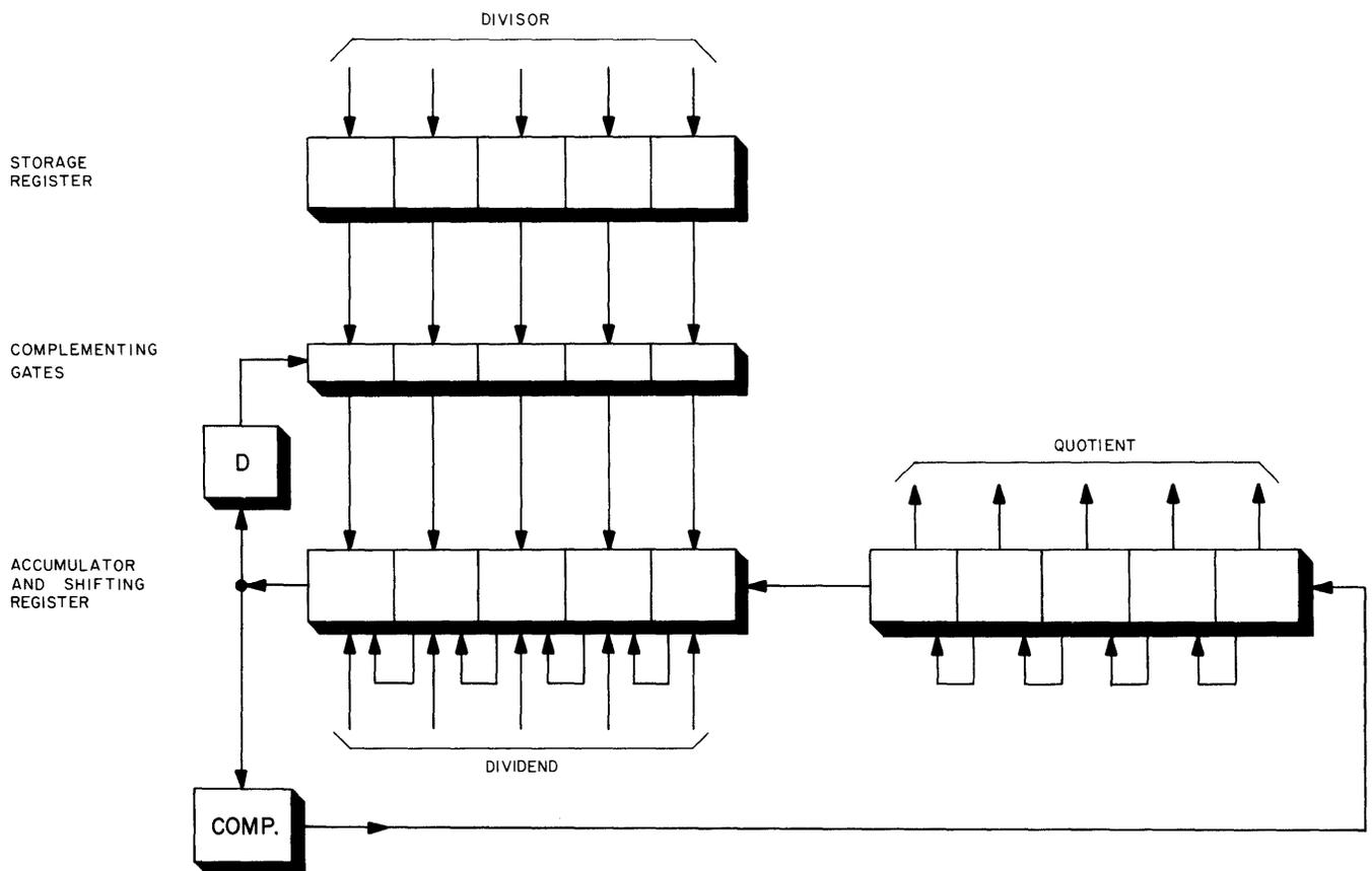
Figure 3-78. Shifting Accumulator Used for Division
