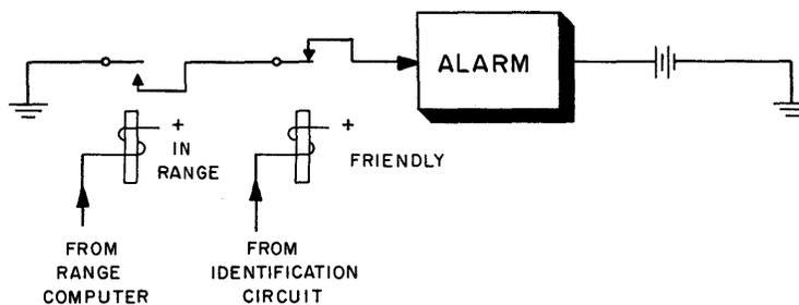
Figure 3-16. Relay AND NOT Circuit
