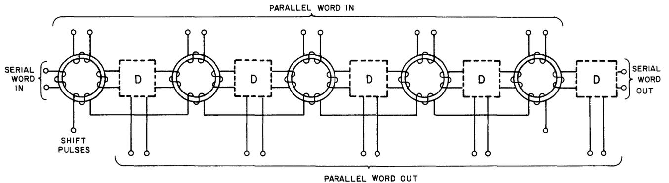
Figure 3-54. Core Shifting Register
