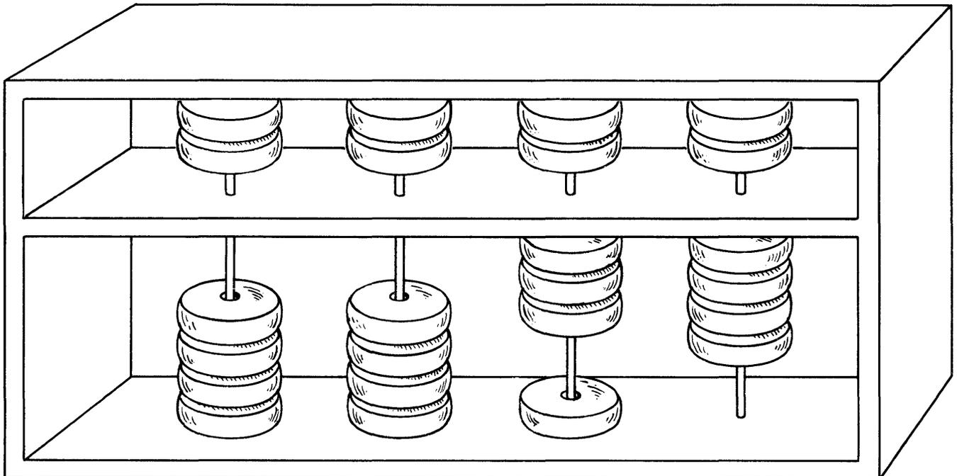
**Figure 1-4. The Abacus – The Number Represented by the Position of the Beads is 34**
