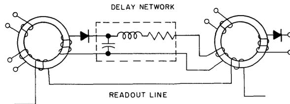
Figure 3-35. Interconnection of Magnetic Cores
