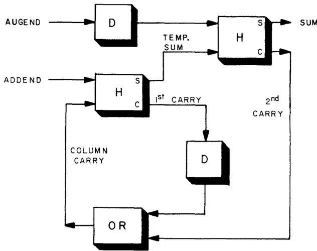
Figure 3-66. Full Adder for Serial Operation
