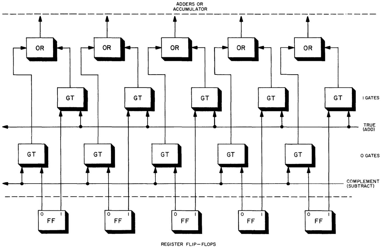
Figure 3-70. Arrangement for Transfer of True or 1's Complement Number
