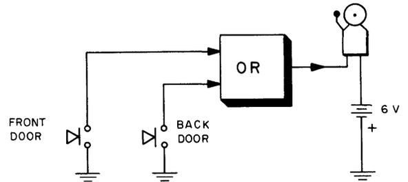
Figure 3-12. Doorbell Circuit, Showing Logic
