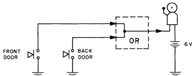
Figure 3-13. Complete Doorbell OR Circuit
