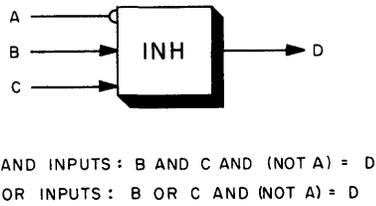
Figure 3-10. Inhibit Function
