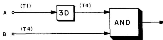
Figure 3-20. Use of Compensating Delay
