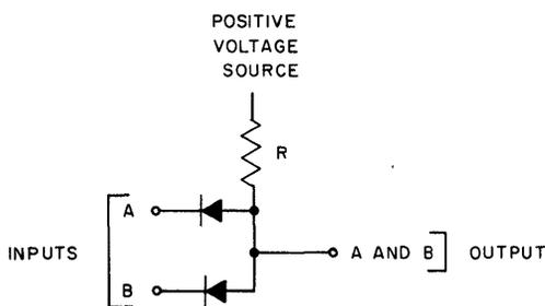
Figure 3-19. Diode AND Circuit
