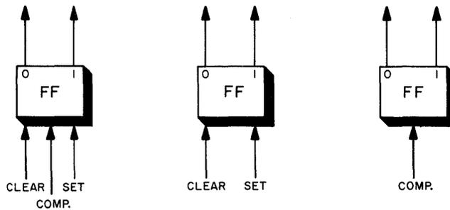
Figure 3-43. Flip-Flop Circuit Symbols
