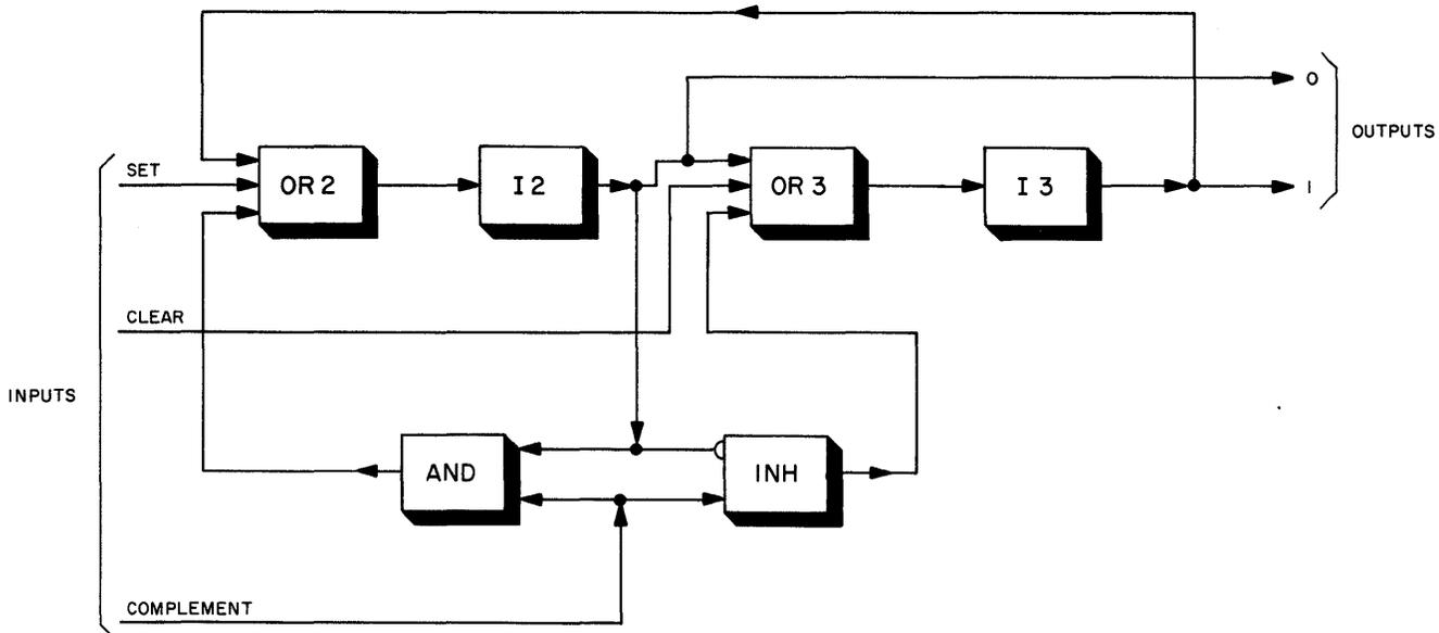
Figure 3-42. Complete Logic Circuit Flip-Flop
