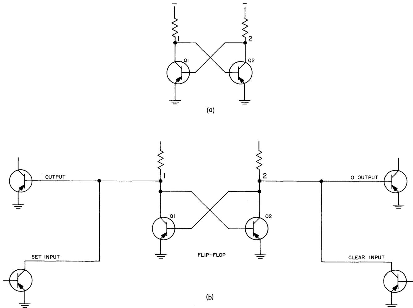
Figure 3-46. Transistor Flip-Flop
