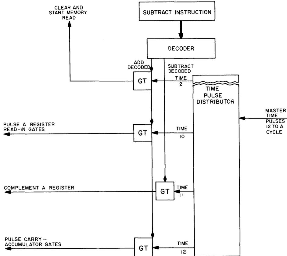
Figure 4-17. Subtract Instruction Arithmetic Control (Operate Time)
