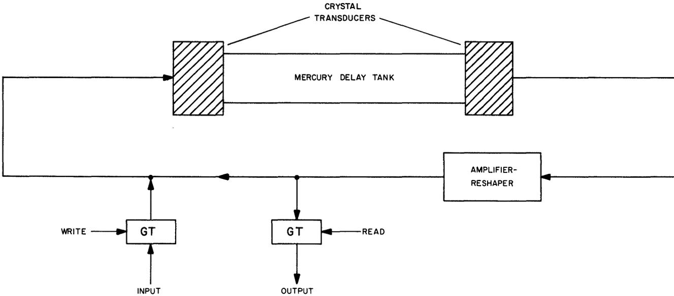
Figure 3-90. Acoustic Delay Line
