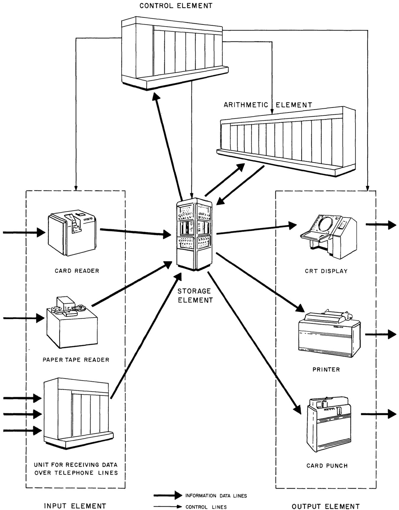
Figure 1-11. Organization of a Typical Digital Computer
