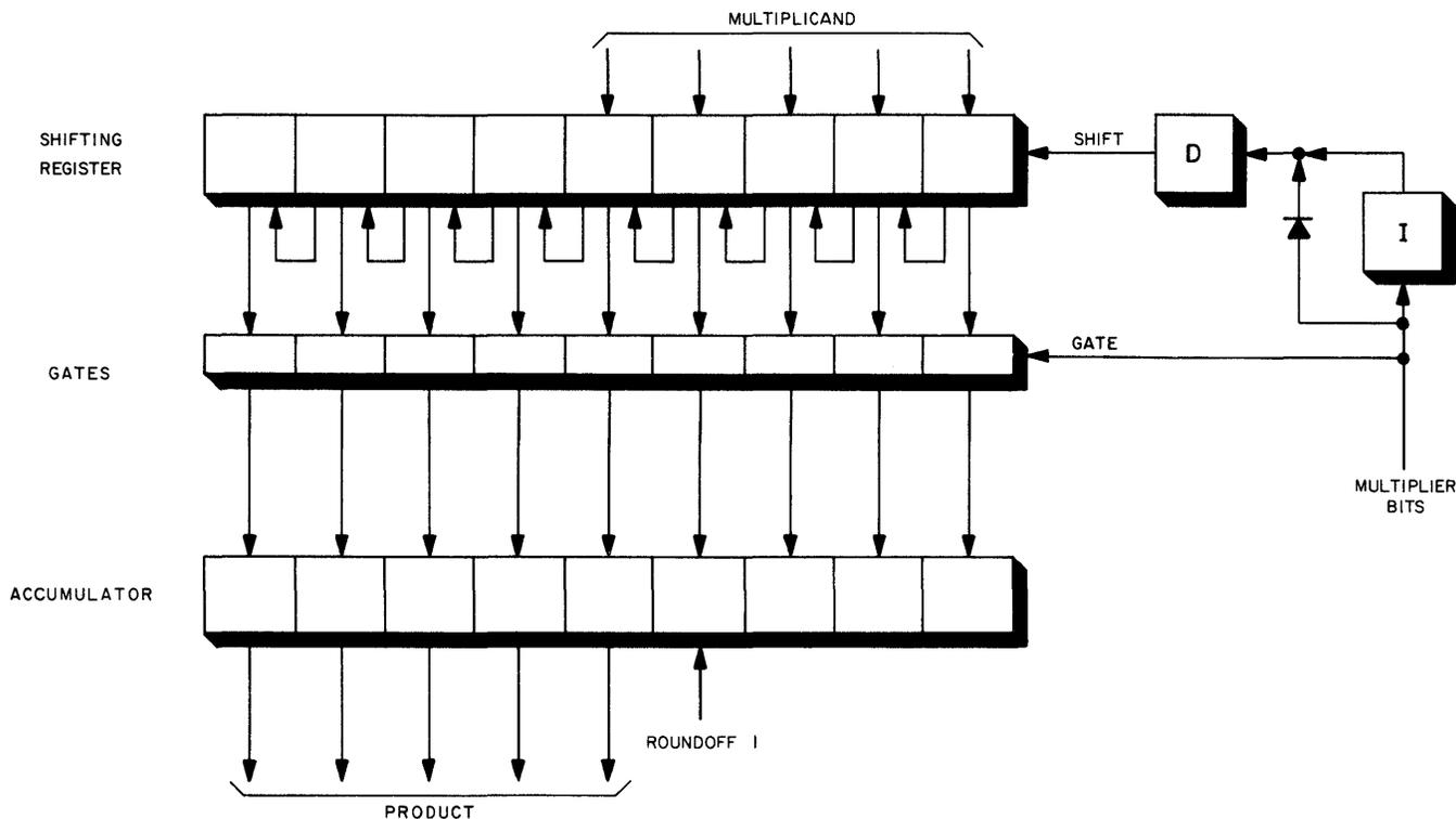
Figure 3-71. Shifting Register Feeding Accumulator for Multiplication
