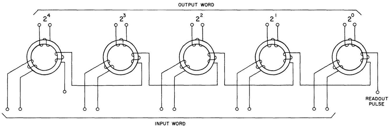
Figure 3-51. Parallel Core Register
