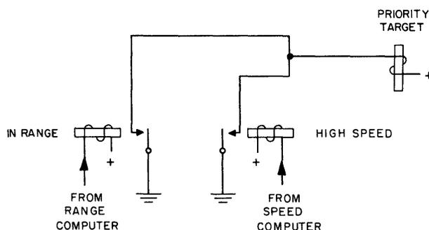
Figure 3-14. Relay OR Circuit
