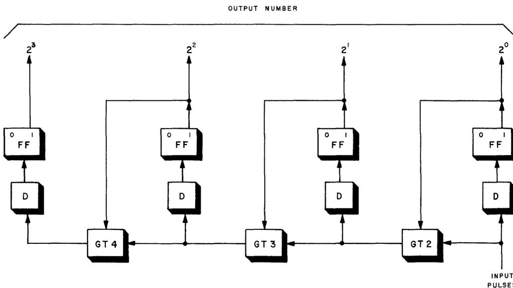
Figure 3-60. Higher Speed Counting Register
