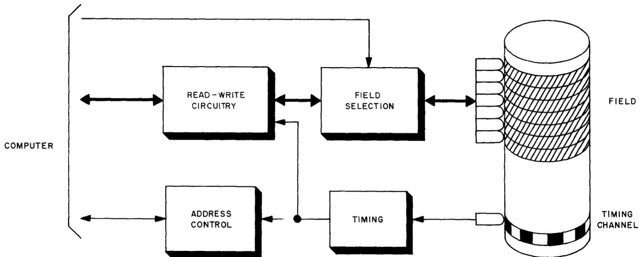
Figure 3-86. Address Selection of Drum Registers
