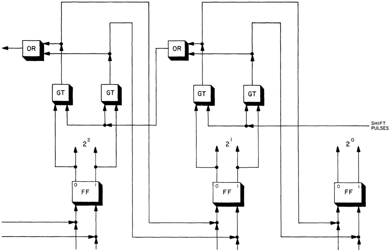
Figure 3-56. Register Using Ripple Shift
