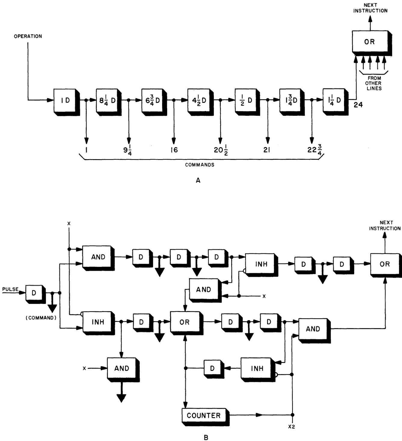
Figure 3-82. Delay Lines for Asynchronous Control
