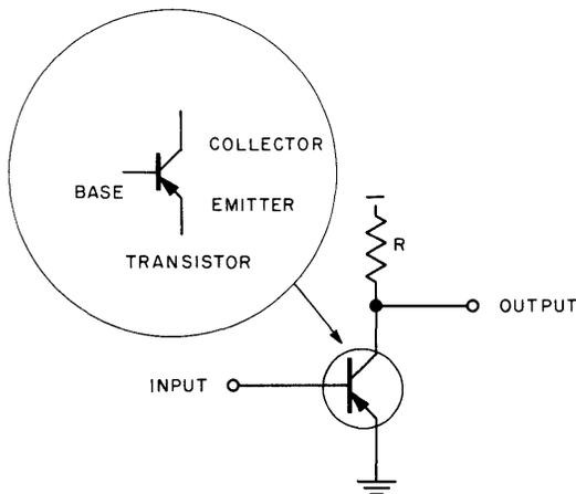
Figure 3-28. Basic Transistor Switch
