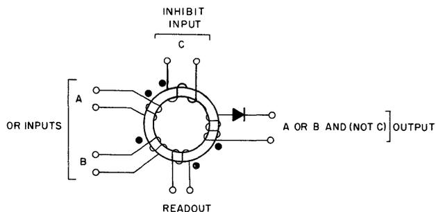
Figure 3-36. Magnetic Core Inhibit Arrangement
