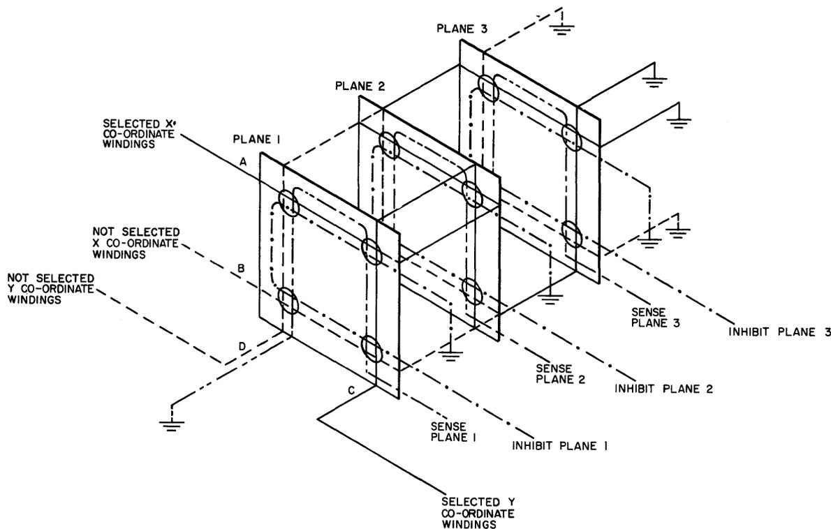
Figure 4-4. 4-Location 3-Bit Register Core Array
