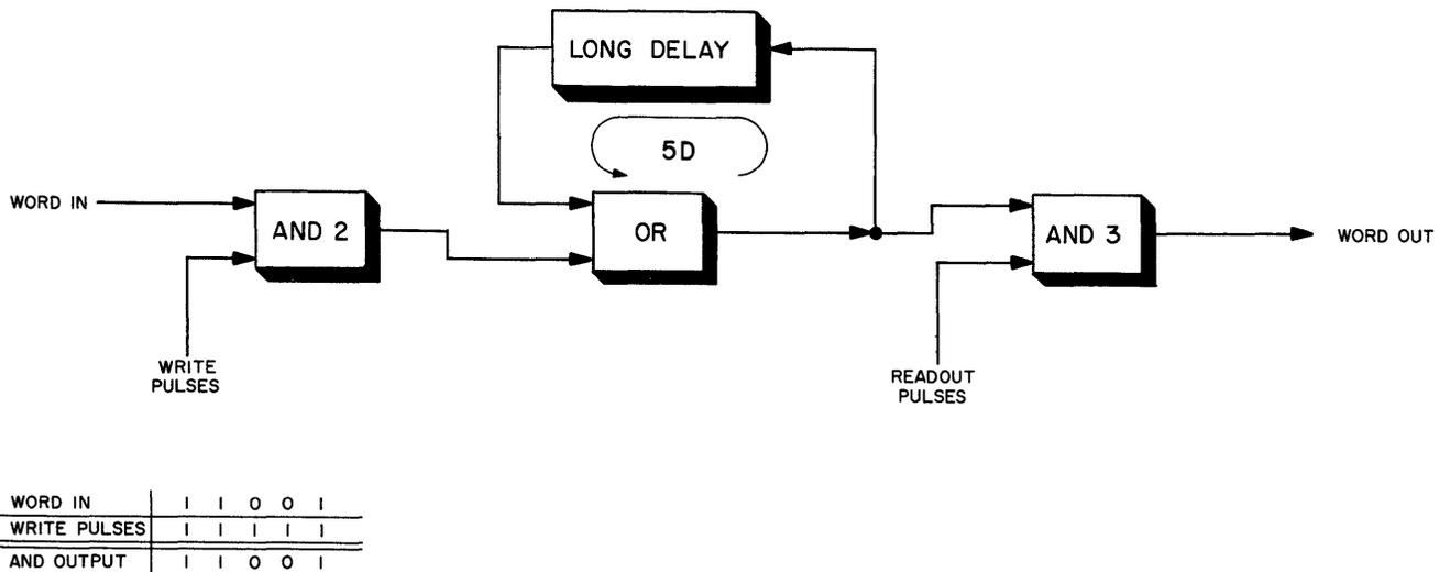
Figure 3-52. Circulating Register for Serial Words
