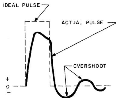
Figure 3-57. Typical Pulse in Computer Circuitry
