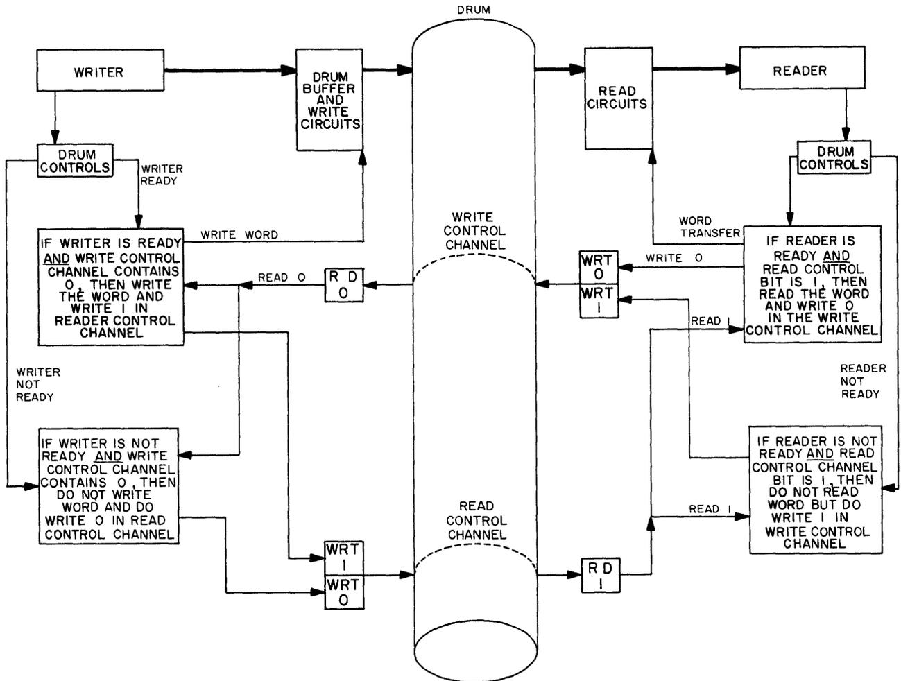
Figure 4-20. Status Control of Drum
