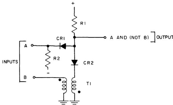
Figure 3-21. Diode Inhibit Circuit for Pulse Signals
