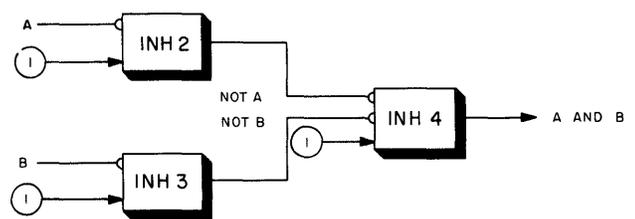
Figure 3-38. Magnetic Core AND Circuit
