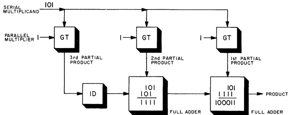
Figure 3-77. Serial-Parallel Multiplication
