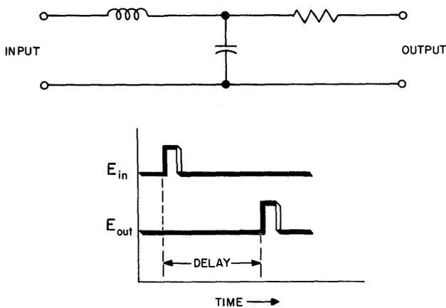
Figure 3-49. Basic Delay Line Section
