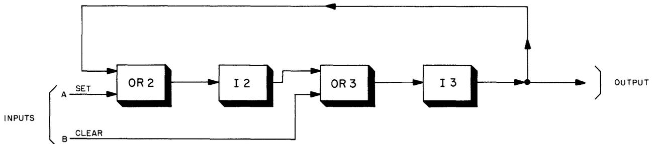
Figure 3-41. Basic Bistable Storage Circuit
