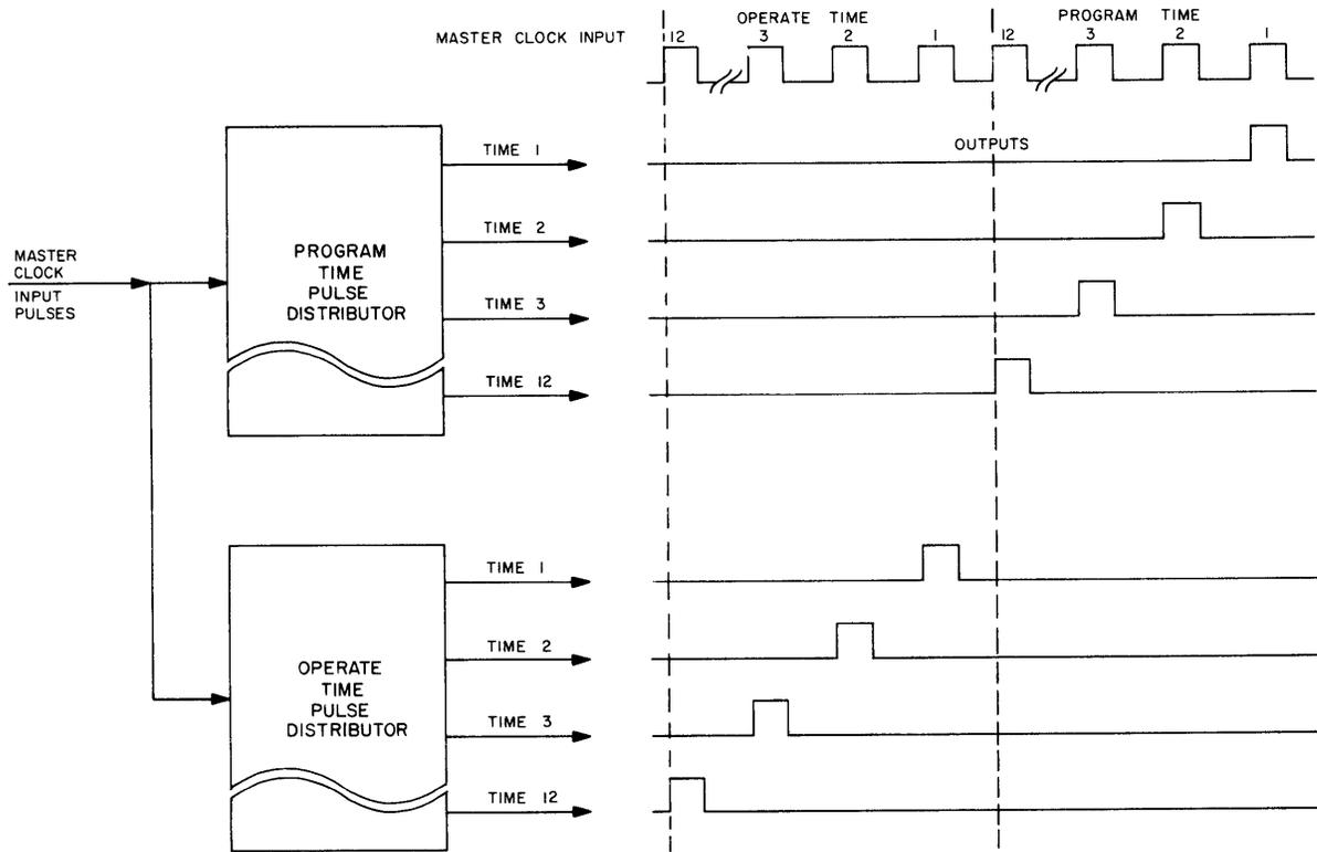
Figure 4-9. Program Time: Operate Time, Pulse Distributor Operation
