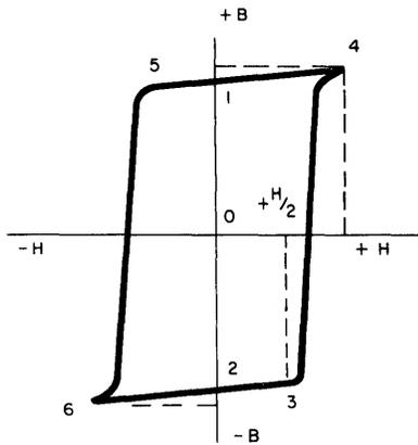
Figure 3-33. Magnetic Core and Hysteresis Loop
