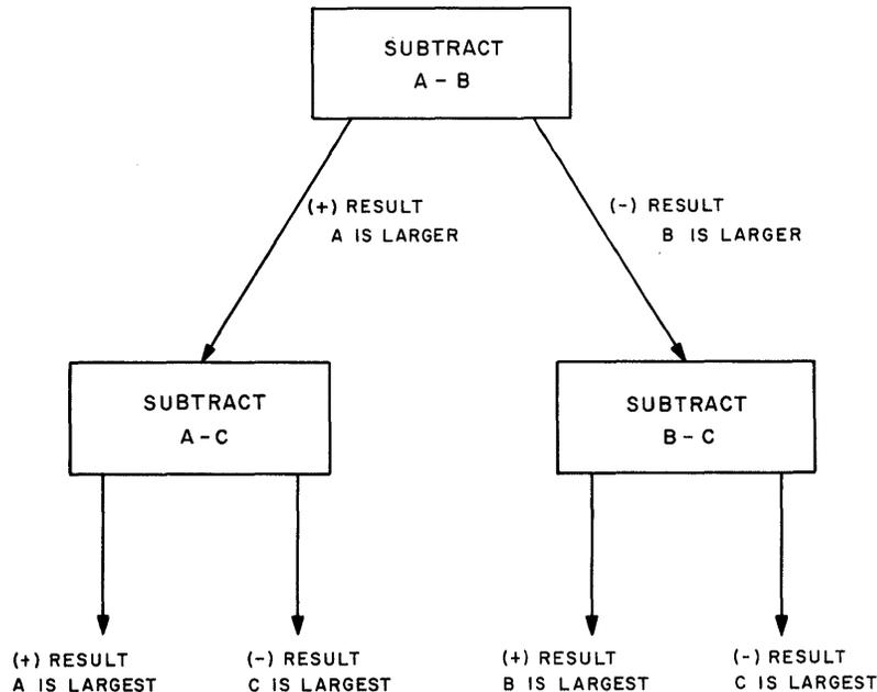
Figure 1-2. Data Processing — Finding the Largest of Three Numbers, A, B, and C
