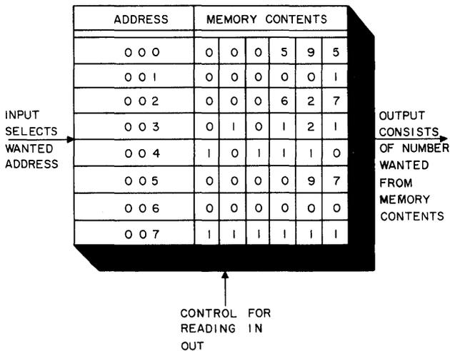
Figure 1-9. Storage Element - Possible Address and Contents Correlation
