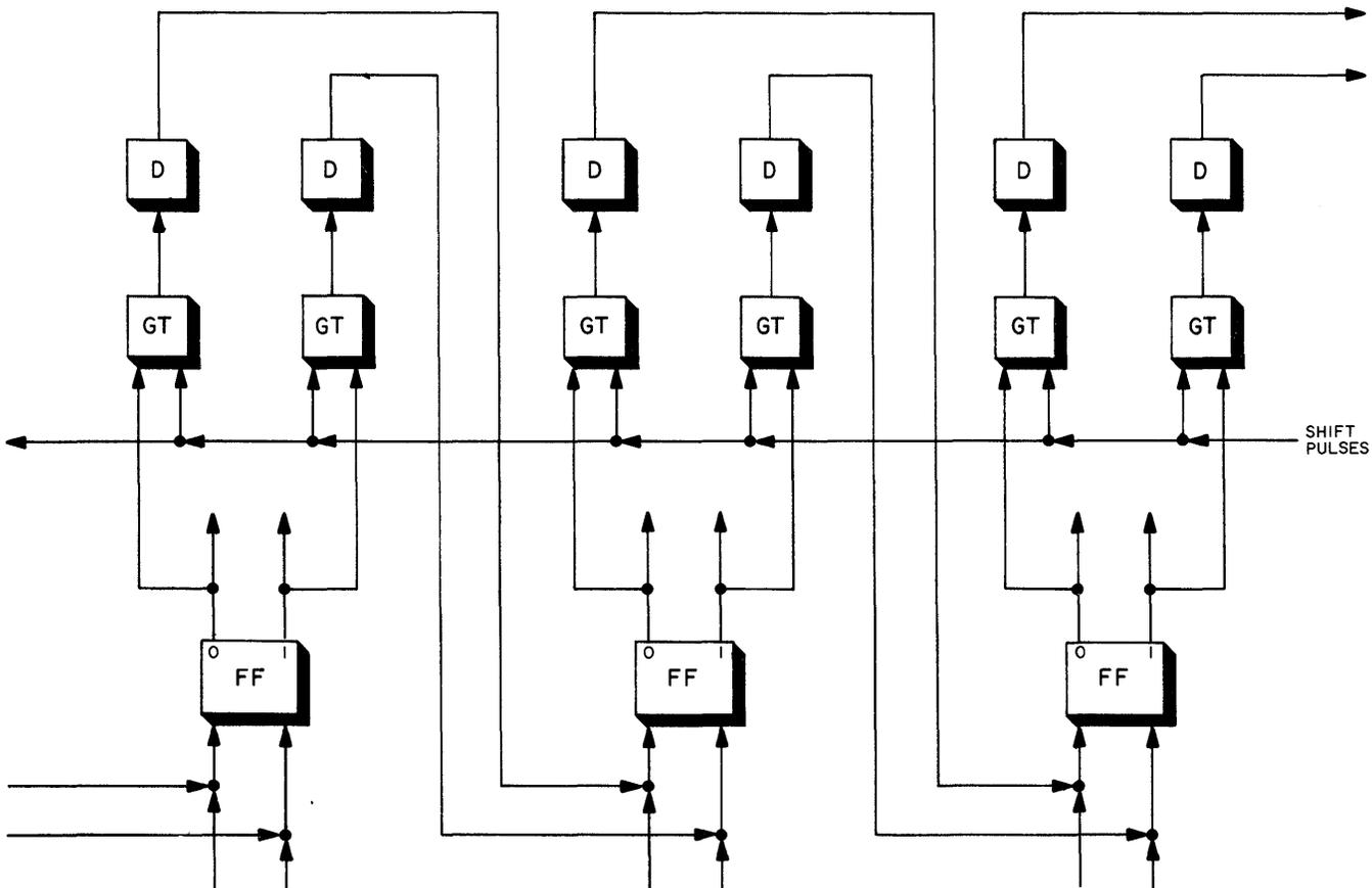
Figure 3-55. Flip-Flop Shifting Register
