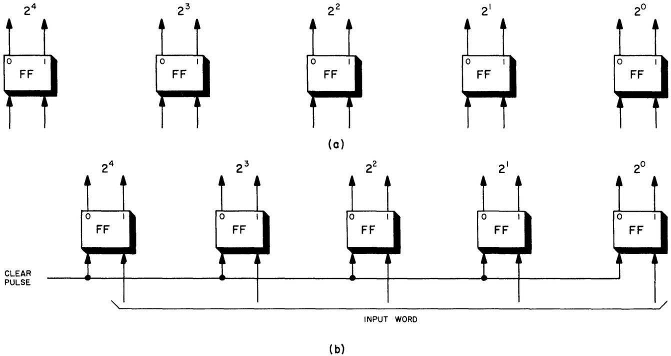
Figure 3-50. Parallel Flip-Flop Storage Register
