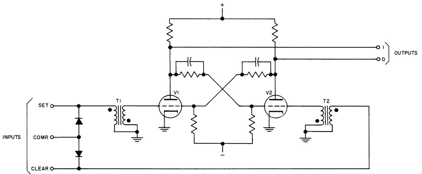
Figure 3-45. Basic Vacuum Tube Flip-Flop
