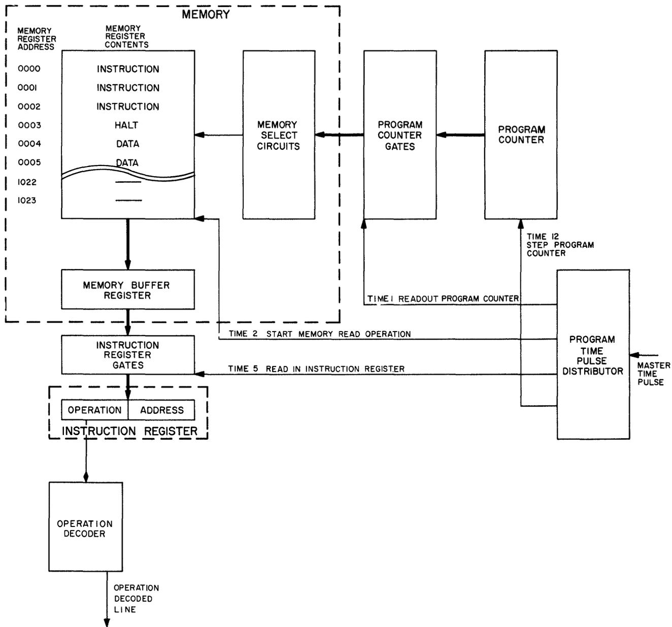
Figure 4-10. Instruction Selection, Readout, and Decoding (Program Time)
