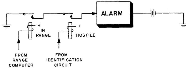
Figure 3-15. Relay AND Circuit
