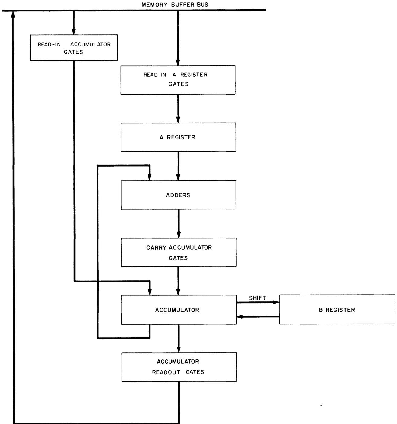
Figure 4-15. Arithmetic Element Information Flow
