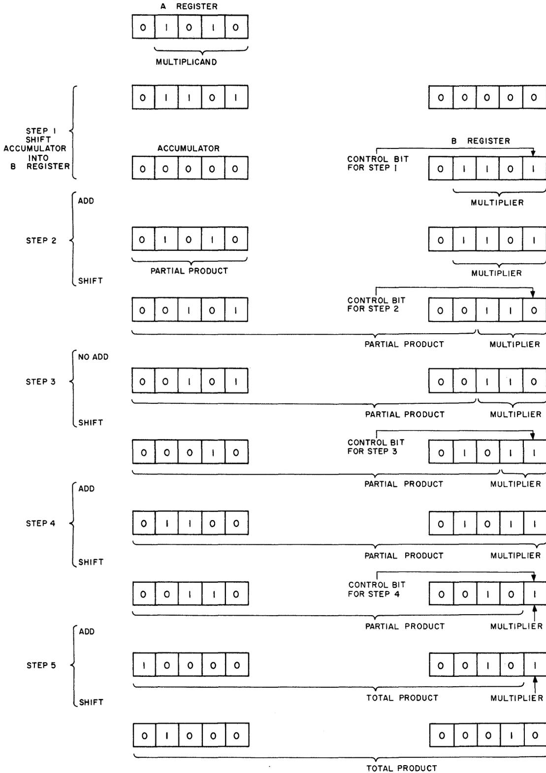
Figure 4-18. Contents of A-Register, B-Register, and Accumulator During Multiplication
