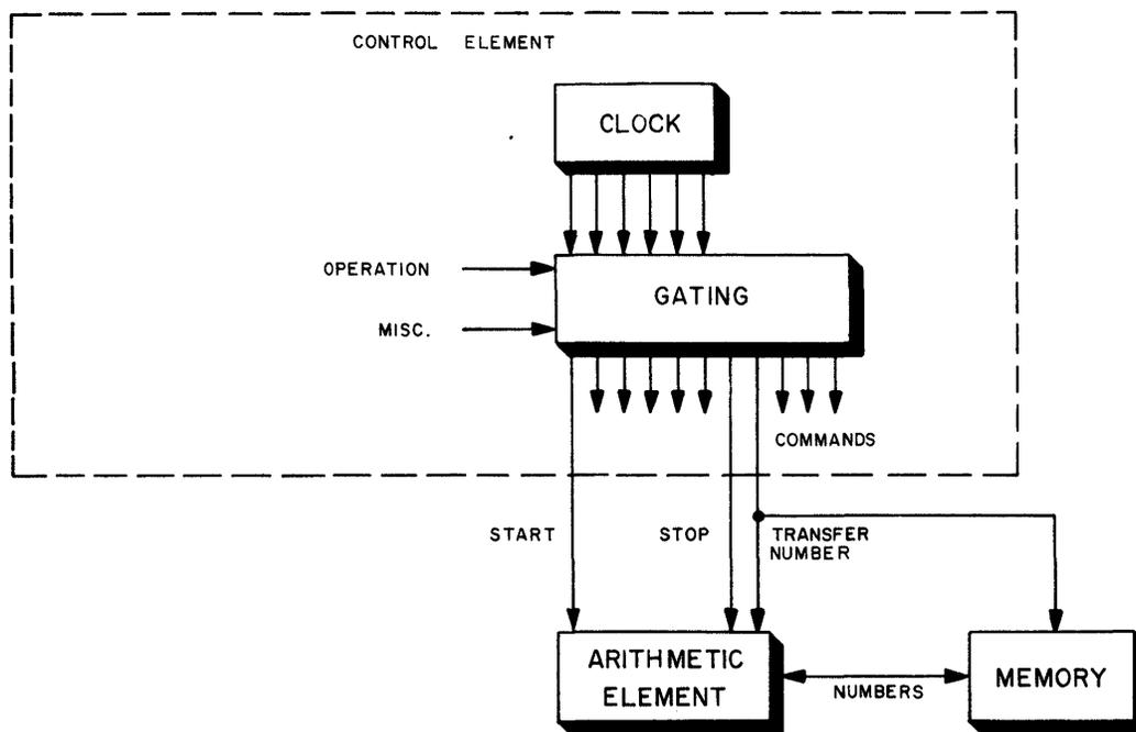
Figure 3-80. Synchronous Control of Operations
