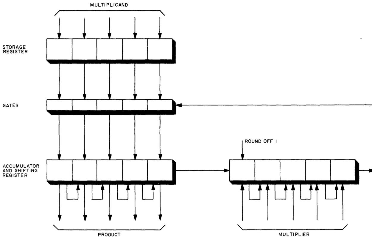
Figure 3-73. Shifting Accumulator Used for Multiplication
