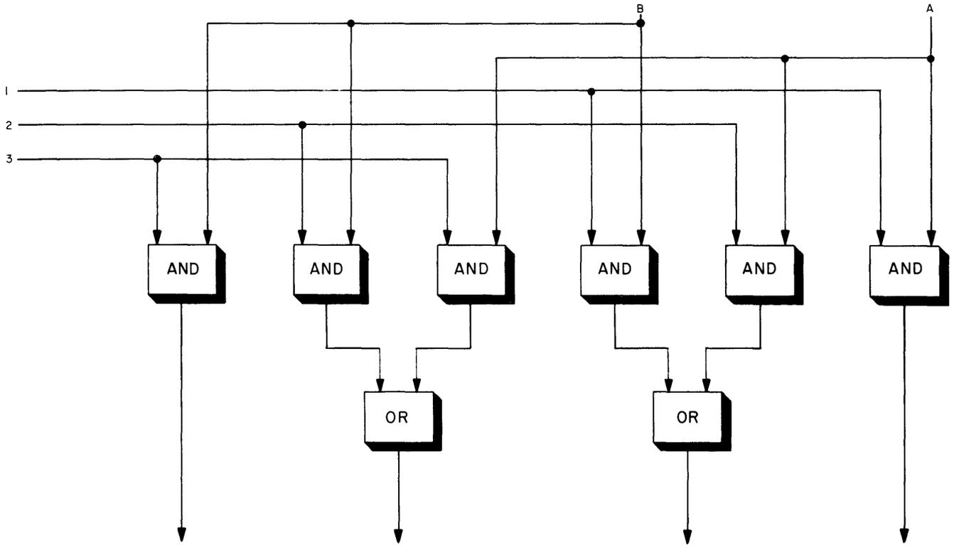
Figure 3-72. Gating and Shifting by Switching
