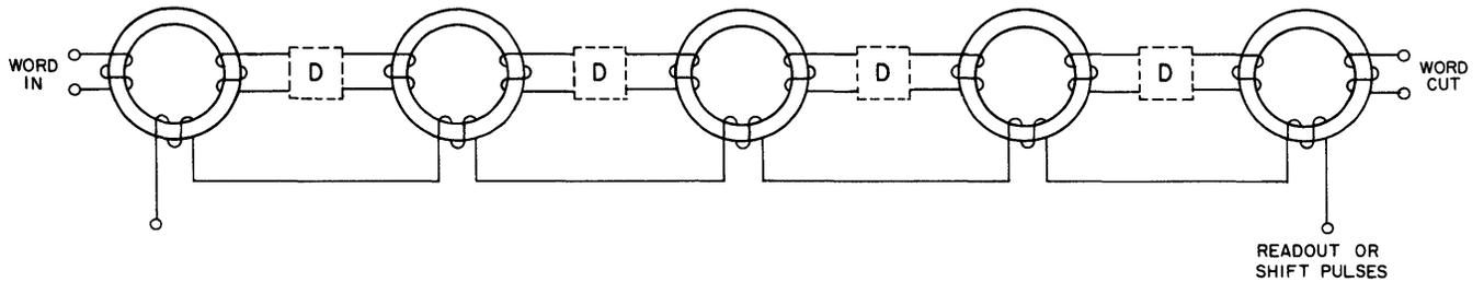
Figure 3-53. Core Register for Serial Words
