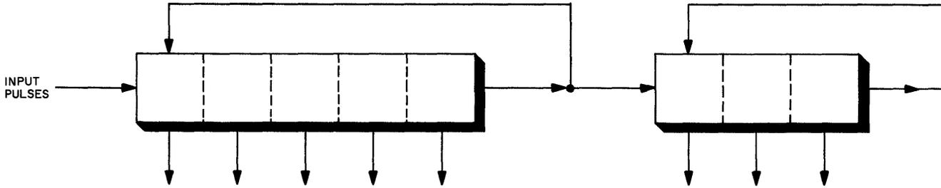
Figure 3-62. Using Ring Counters in tandem
