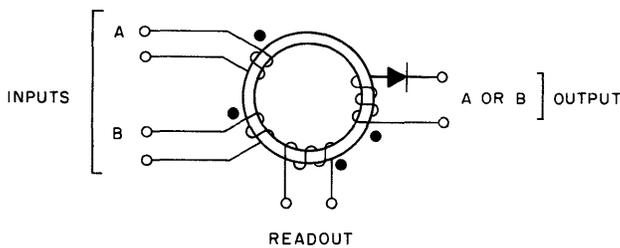
Figure 3-34. Magnetic Core OR Arrangement
