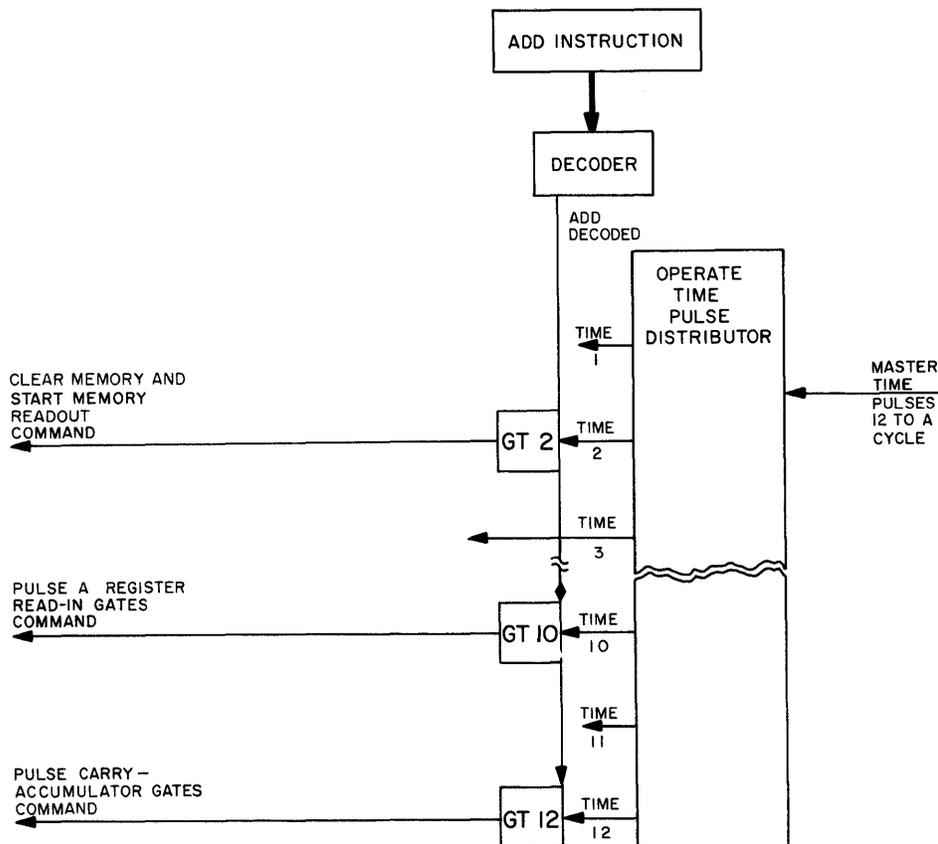
Figure 4-16. Add Instruction Arithmetic Control (Operate Time)
