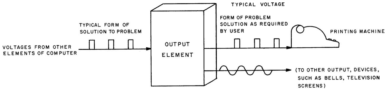
**Figure 1-7. Output Element — This Element Converts Computer's Answer to the Problem into Form Usable by External Output Devices**
