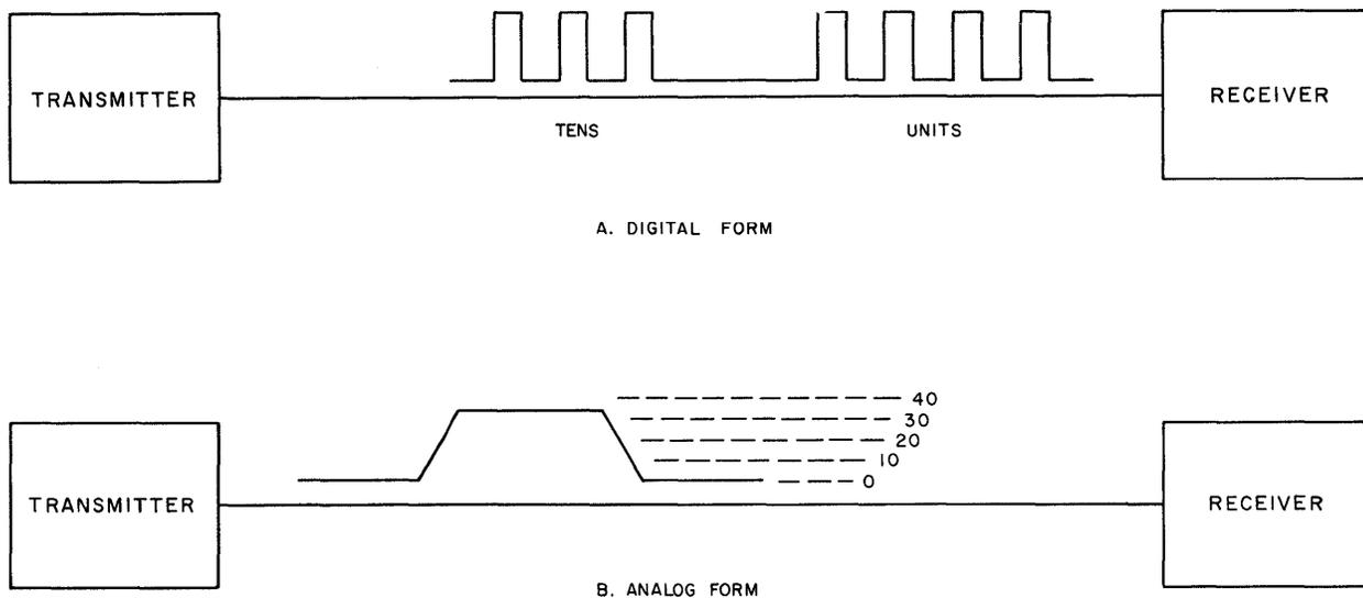
Figure 1-3. Digital and Analog Representations of the Number 34
