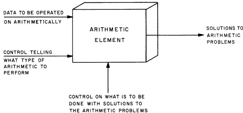
**Figure 1-8. Arithmetic Element — Data Enters and Is Processed by this Element**
