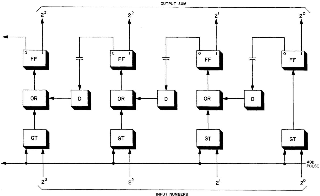
Figure 3-68. Parallel Accumulator
