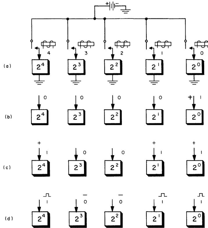
Figure 3-2. Parallel Transmission of Numbers
