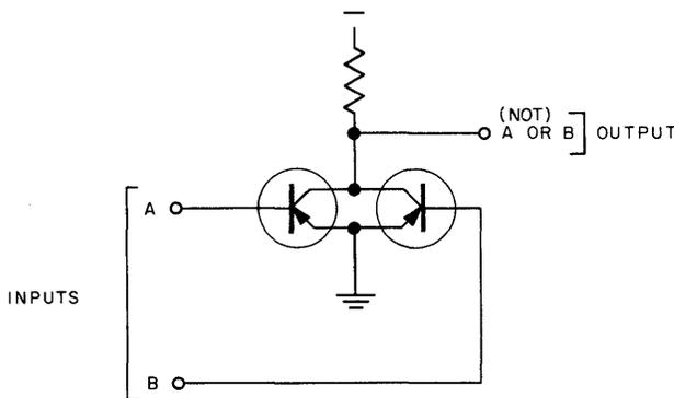
Figure 3-29. Transistor OR Circuit
