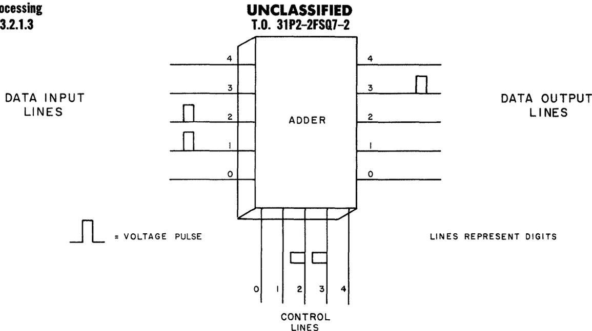
Figure 1–5. Numbers and Control Instructions Represented in the Form of Voltages
