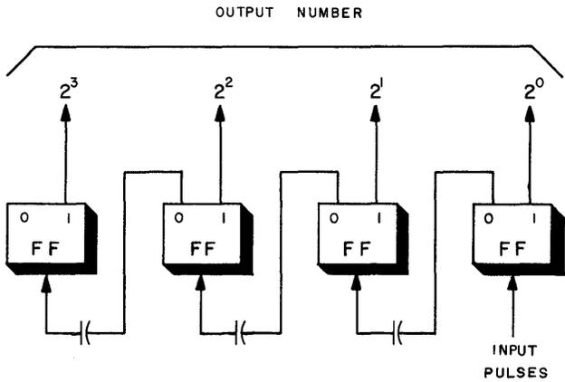
Figure 3-59. Basic Flip-Flop Counter
