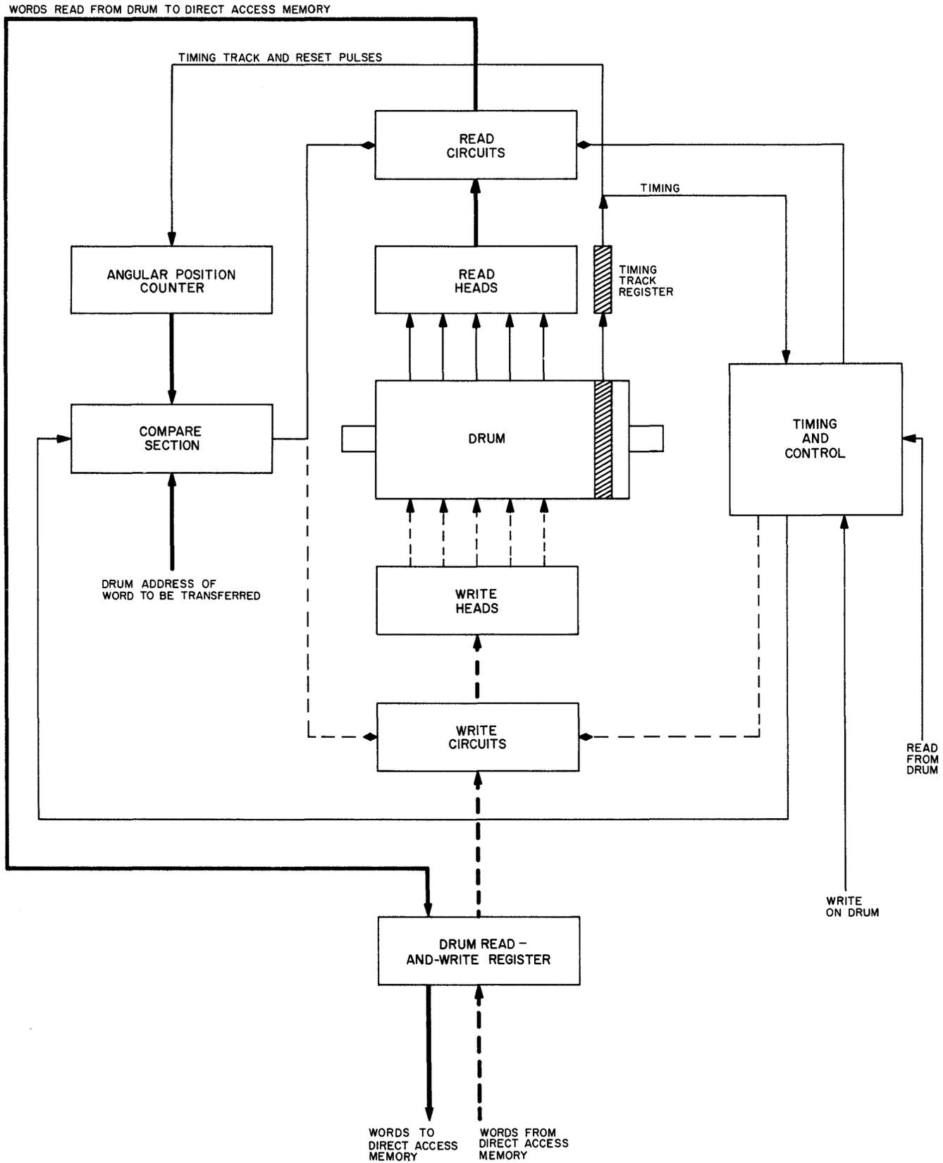
Figure 4-8. Auxiliary Memory Drum System Operation
