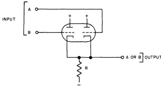
Figure 3-24. Vacuum Tube OR Circuit
