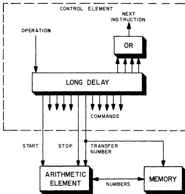
Figure 3-81. Asynchronous Control of Operations
