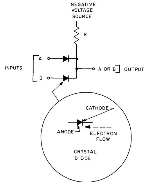
Figure 3-18. Diode OR Circuit
