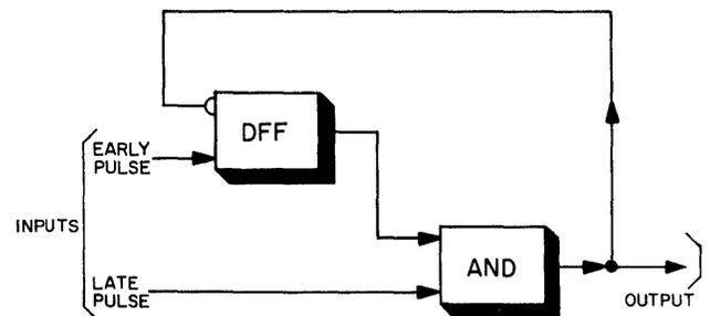
Figure 3-48. Use of Dynamic Flip-Flop
