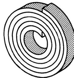
Figure 3-32. Tape Core Construction
