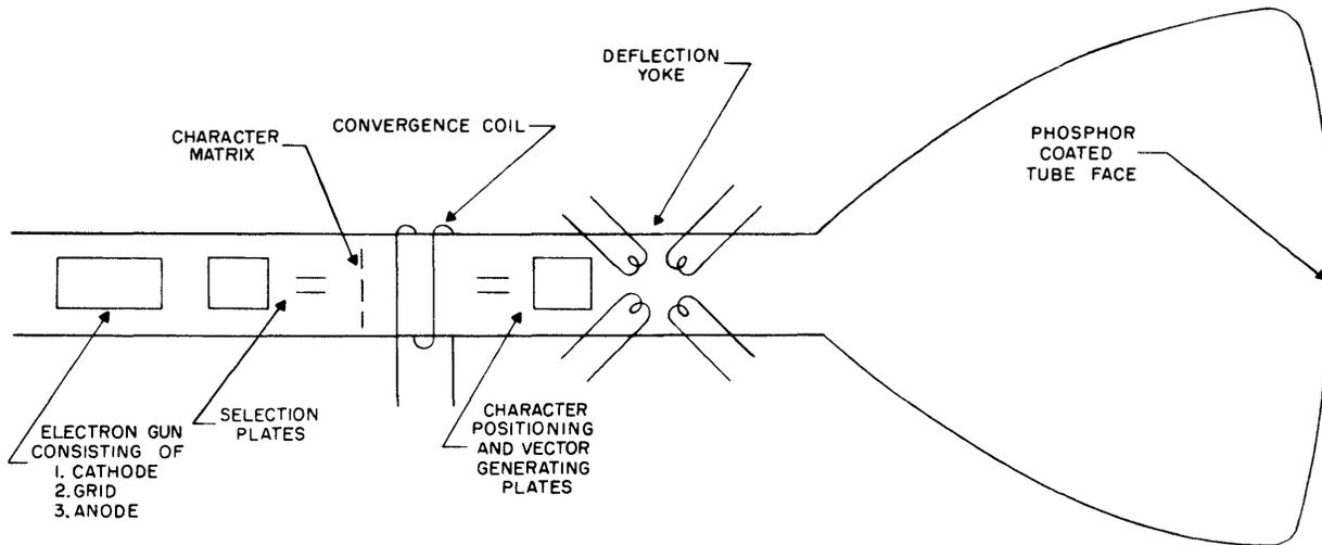
Figure 3-100. Display Tube, Simplified Diagram
