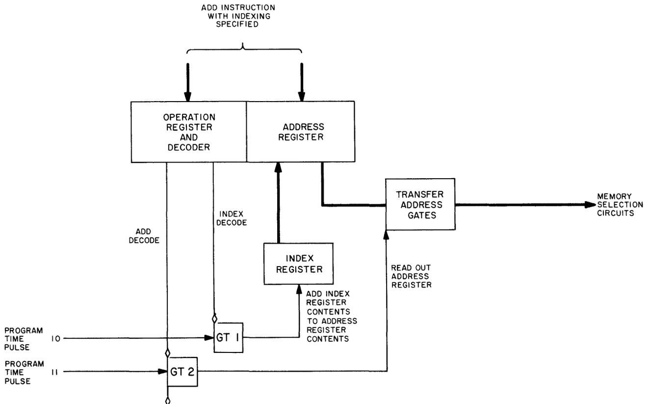
Figure 4-14. Address Modification by Index Register
