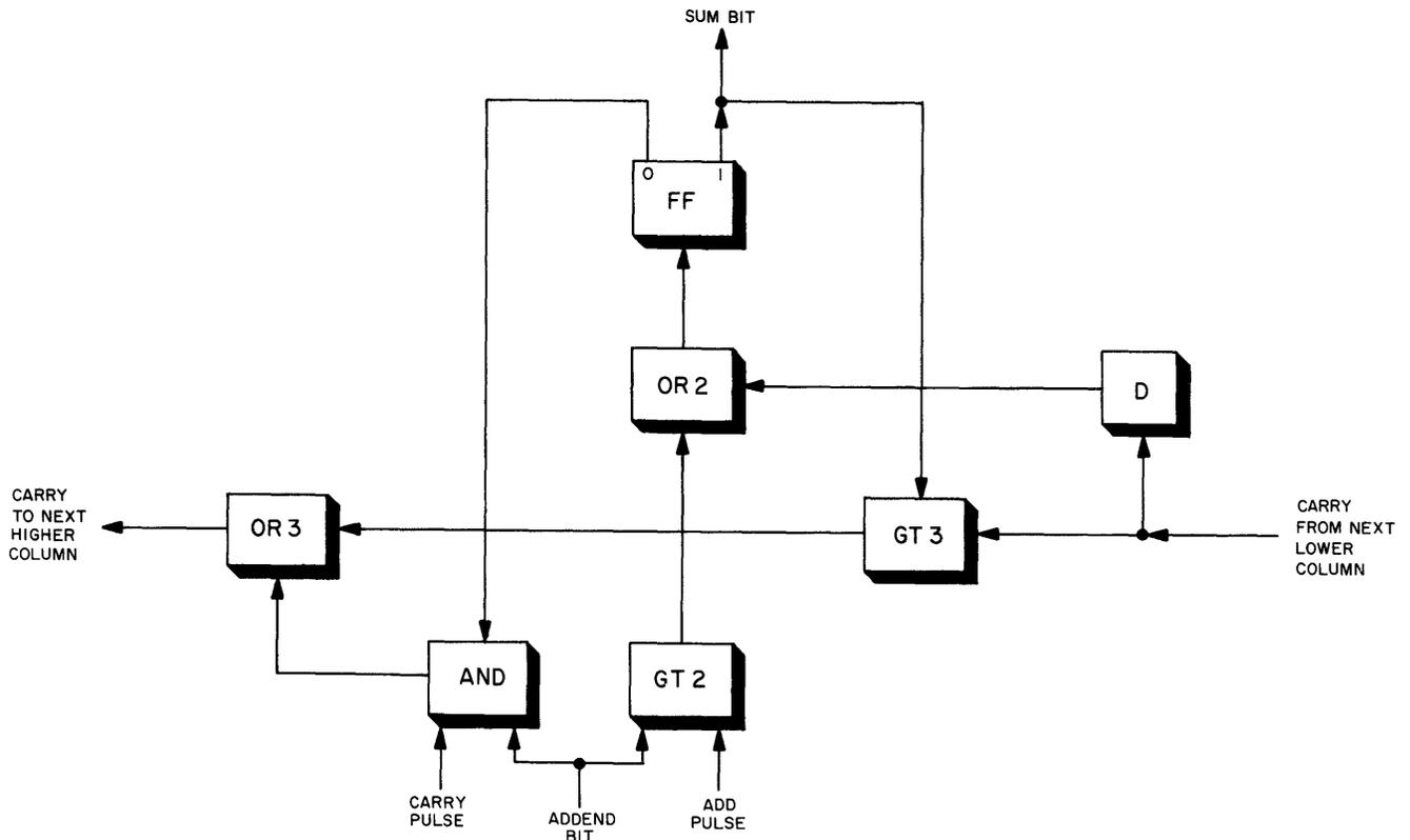
Figure 3-69. Stage of Accumulator With Faster Carry Propagation
