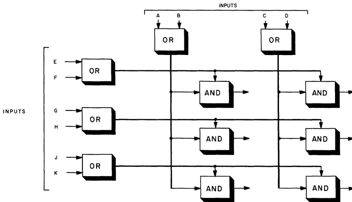
Figure 3-40. Matrix of Logic Circuits
