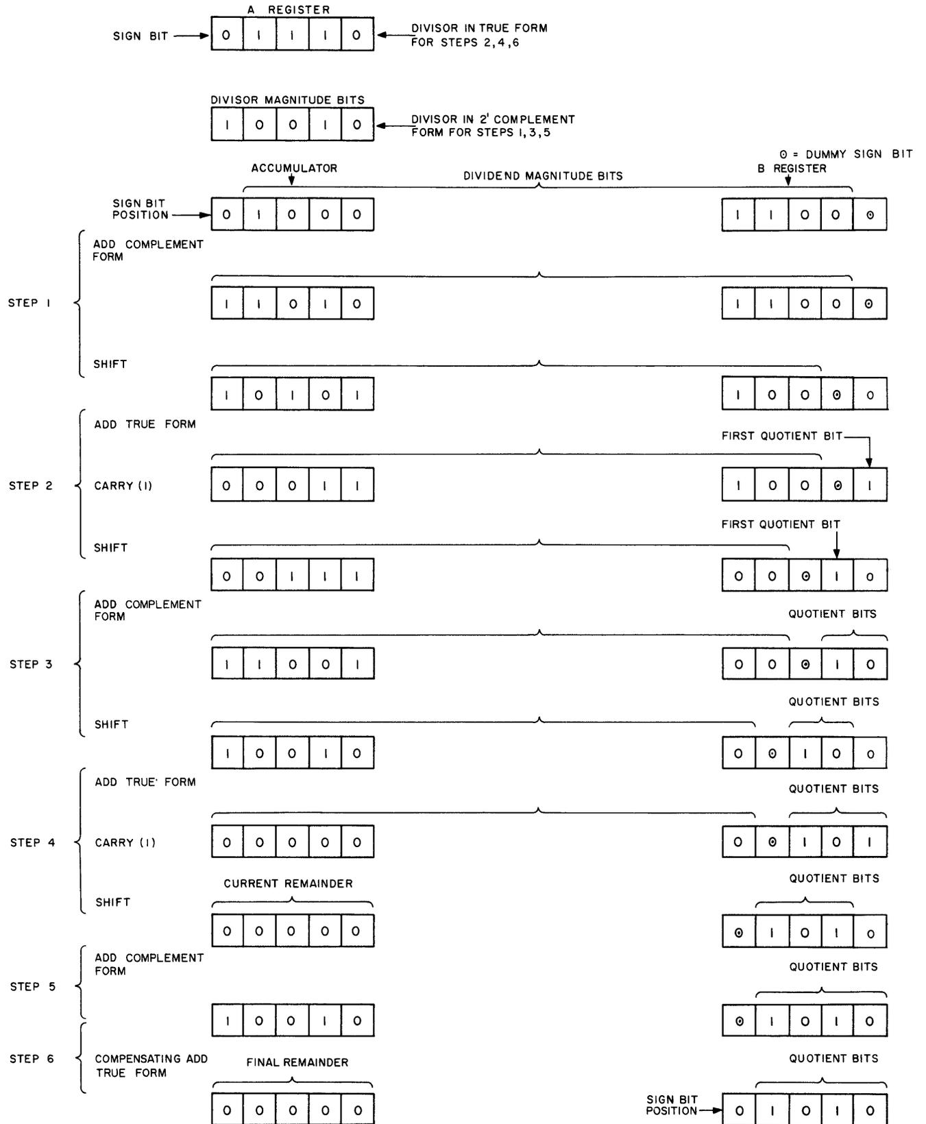
Figure 4-19. Contents of A-Register, B-Register, and Accumulator During Division
