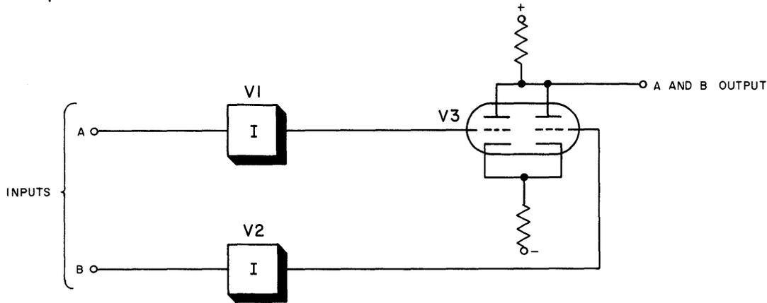
Figure 3-26. Vacuum Tube AND Circuit
