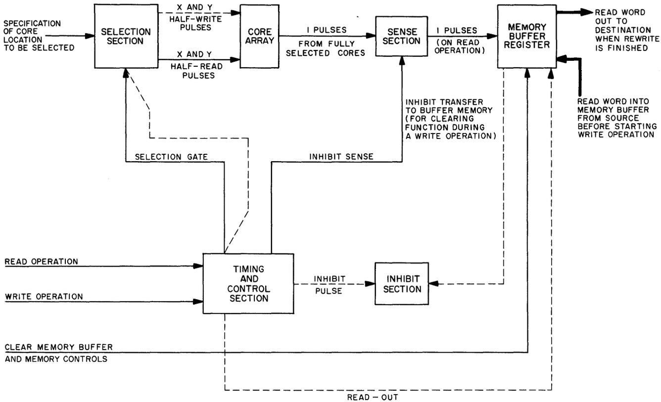
Figure 4-5. Read and Write Operation of Memory
