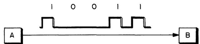
Figure 3-3. Serial Transmission of Numbers
