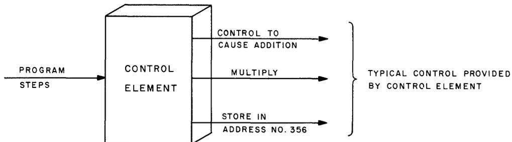
Figure 1-10. Typical Instructions from Control Element
