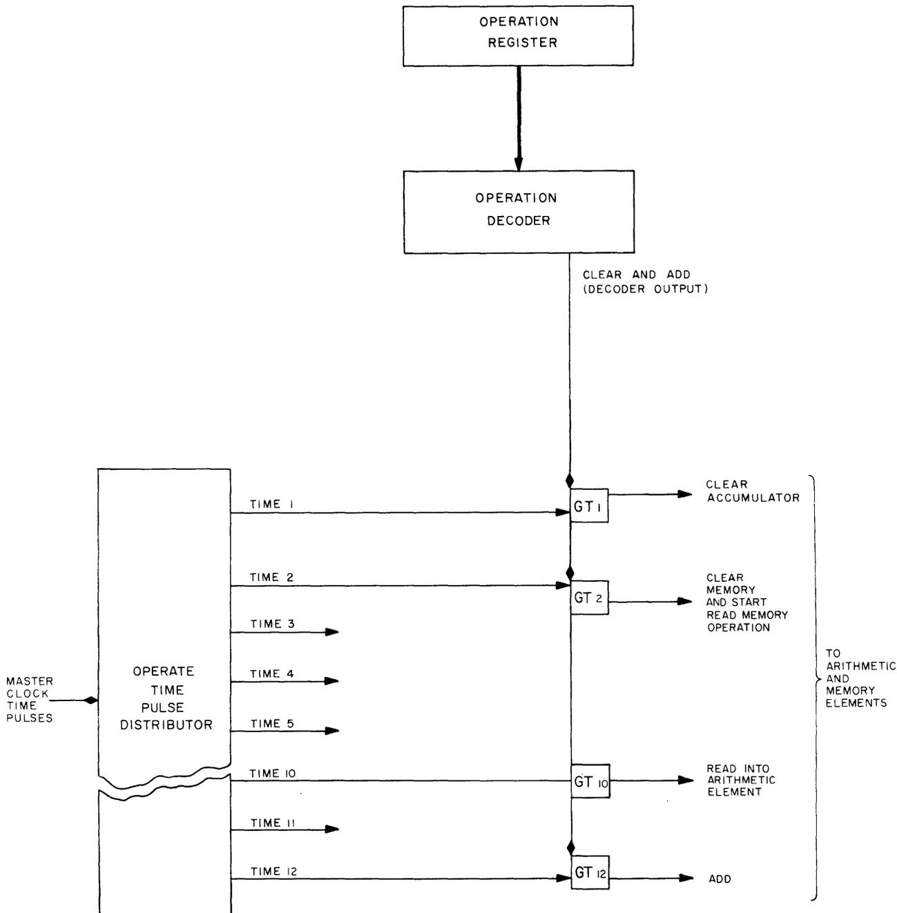
Figure 4-11. Instruction Decoding (Operate Time)
