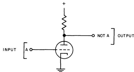
Figure 3-23. Vacuum Tube NOT Circuit
