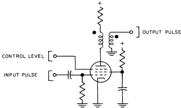
Figure 3-27. Gate Circuit
