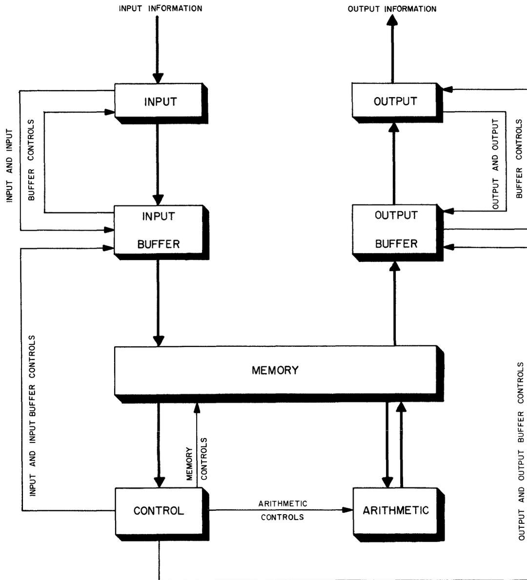
Figure 4-1. Elements of the Sample Computer
