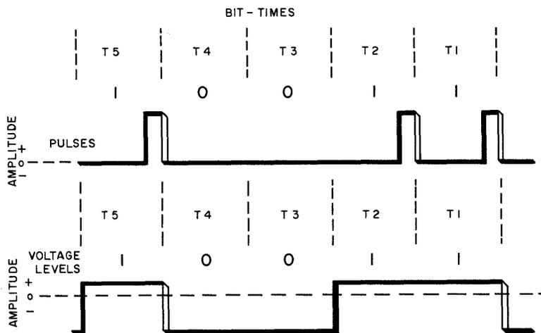
Figure 3-4. Timing of Serial Numbers
