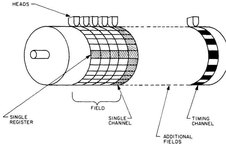
Figure 3-85. Storage on Magnetic Drum
