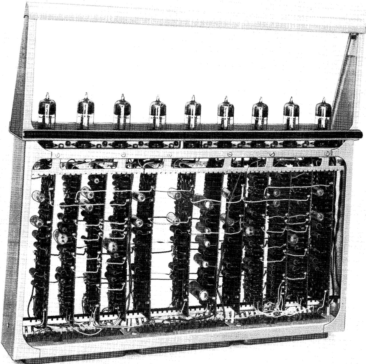
*Figure 3-58. Circuits Packaged in Pluggable Unit*
