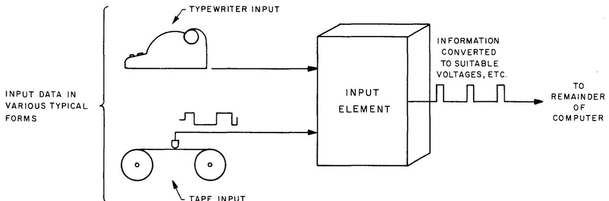
Figure 1-6. Input Element — This Element Receives Information and Converts it into Usable Form
