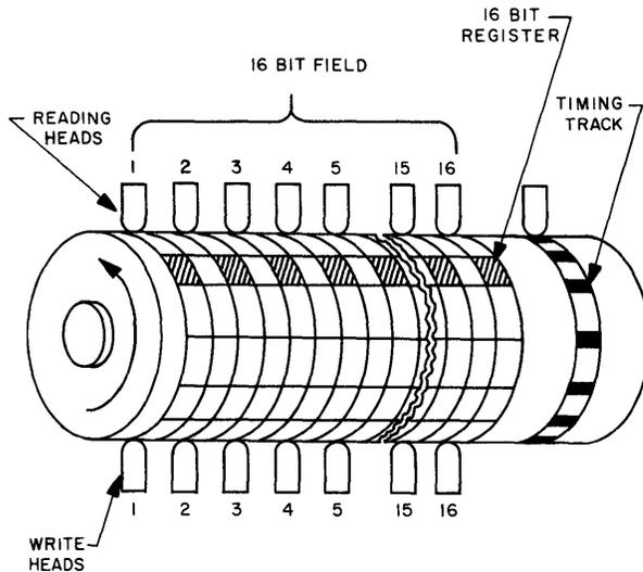
Figure 4-7. Auxiliary Memory Drum
