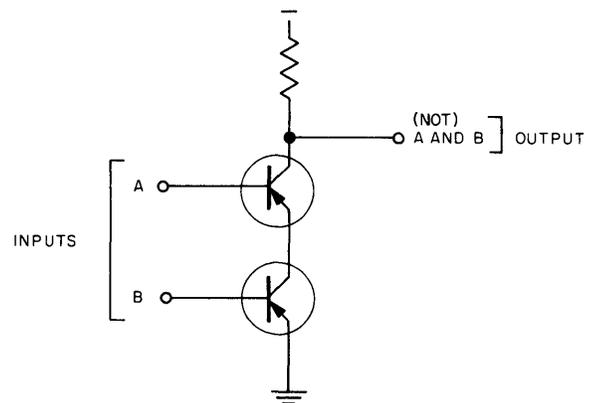
Figure 3-30. Transistor AND Circuit
