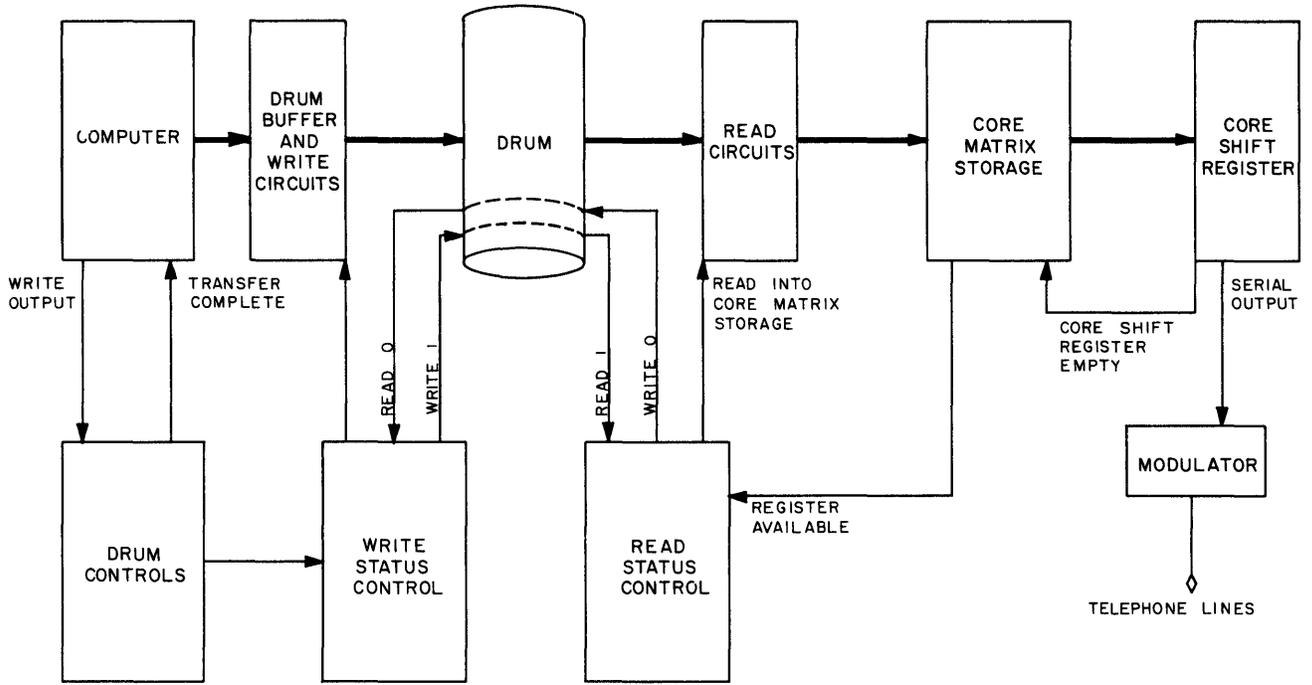
Figure 4-23. Automatic Output System
