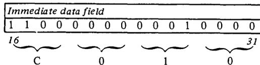
The Read ID (identification) command transfers a one-word identification field, called the DI ID word, into the immediate data field of the IDCB. The hexadecimal value of the integrated digital I/O feature DI ID word is C010. The device-identification word contains a unique identification code and physical information about the device, and can be used to determine the devices that are attached to the system.
