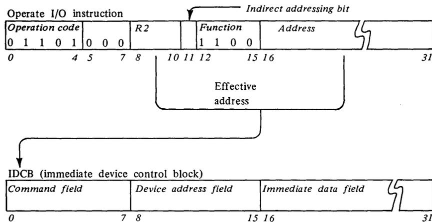
The address field (bits 16–31) and the contents of the register specified in the R2 field (bits 8–10) of the Operate I/O instruction generate an effective address that points to a main-storage location containing an immediate device control block (IDCB). IDCBs are doubleword blocks of storage reserved by programs for storage of device-directed commands.
