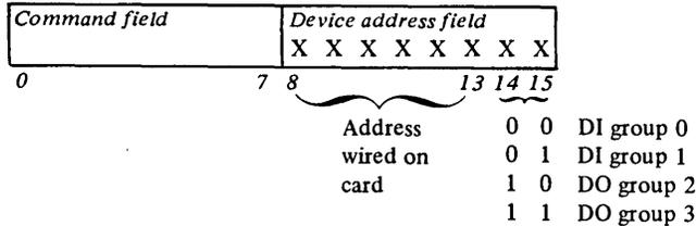
The first six (high-order) bits of the device-address field of the IDCB are defined by field-installable connectors (jumpers) on the integrated digital I/O feature card. The last two bits of the field define the DI groups. Bit values of 00 and 01 in bits 14 and 15 define the DI groups, and bit values of 10 and 11 define the DO groups.
