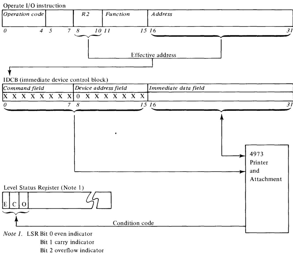
Figure 2-4. Direct Program Control I/O Operation
