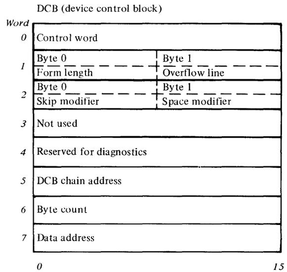
Figure 2-3. Device Control Block
