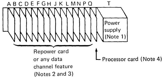
**Figure 1-2. IBM Series/1 4956 Model K00 Plugging Assignments**
